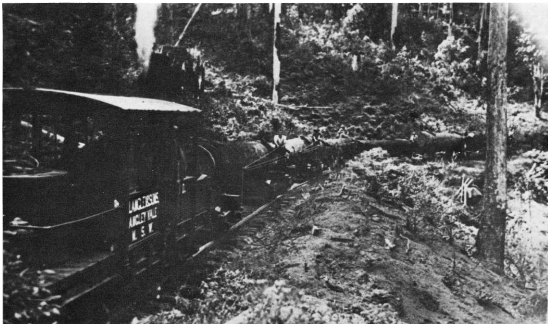
Langley Bros Climax locomotive descending 1 in 50 grade with log train. Note the brakeman applying the brakes on the forward 'sets' while the locomotive coasts downhill in neutral.
