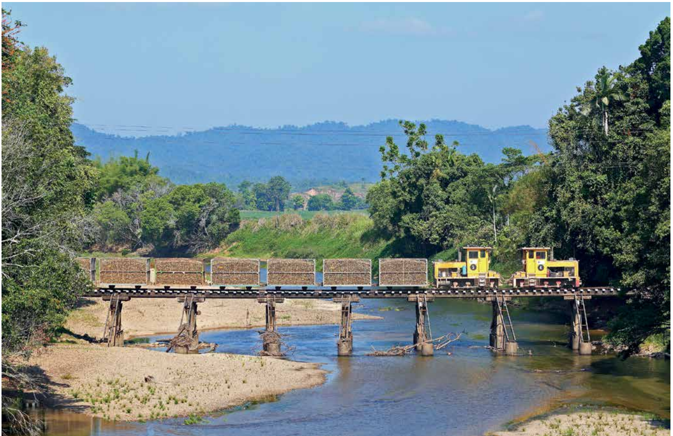
Com-Eng 0-6-0DH multi-unit locos 4 (AD1138 of 1960) and 5 (AH2460 of 1962) cross the Russell River on their way to South Johnstone Mill on 14 November. Photo: Hayden Quabba
