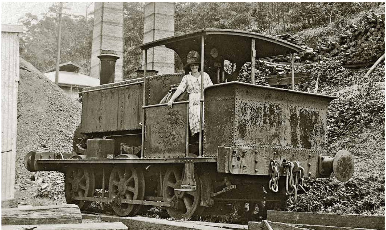
Metropolitan Colliery, 1924, showing a locomotive bearing a builder's plate of Henry Vale 30. However, as mentioned in the article, the loco shows all the attributes of a Manning Wardle. The suspicion is that it is an MW, that Vale repaired (maybe re-boilered) and then sold off, putting his badge on it! The smiling lass on the footplate is believed to be Eileen Carmichael. She and Giff Eardley were married in 1925.
