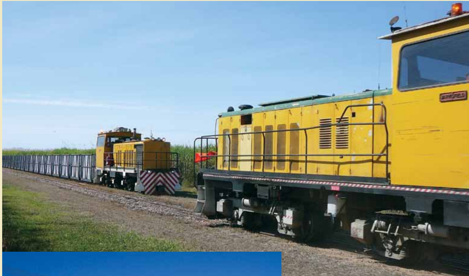
Big yellow bogie cane locomotives: □ Kalamia Mill's Walkers B-B DH JARVISFIELD (601 of 1969 rebuilt Tulk Goninan 1994) waits to cross Invicta Mill's Walkers B-B DH GIRU (593 of 1968 rebuilt Tulk Goninan 1994) hauling 100 new 6-tonne bins at Norham, 9 June. Photo: Luke Horniblow □ Newly rebuilt by N+P Site Boring at Brendale in Brisbane, Victoria Mill's EM Baldwin B-B DH 5423.1 9.74 of 1974, awaits loading for its return trip up north on 15 July. Photo: John Browning □ Victoria Mill's Walkers B-B DH HERBERT II (612 of 1969 rebuilt Walkers 1993) rolls into Goulburn, NSW, for collision damage repairs at the the United Goninan plant on 25 May. Photo: Leon Oberg
