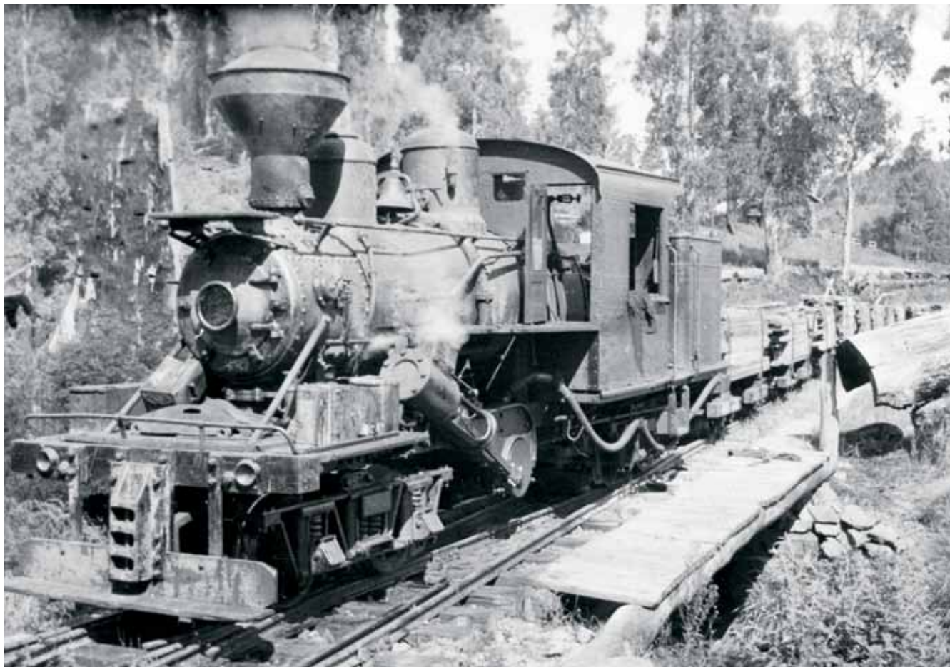
Climax locomotive No.1694 coming into Tyers Junction from West Tyers (on the Ten Acre Block branch). This shows the locomotive with the original riveted smoke box. Photo: W Saxton, courtesy Mike McCarthy
