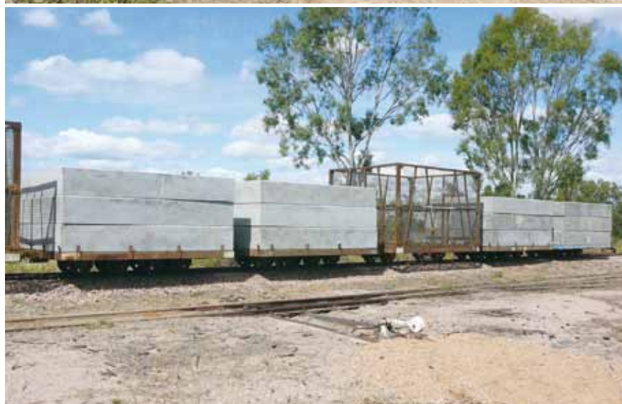
Top: Invicta Mill's Expedition Pass Creek bridge, showing the temporary steel span, the telemetry device described in the news report, and preliminary works being carried out in preparation for the replacement of the pier that was washed away in floods last year. Above: Nearby, the wagons used for load testing on the damaged bridges at Landers Creek and Exhibition Pass Creek. The test wagons each have four axles and are weighted with three 9-tonne blocks of concrete.
