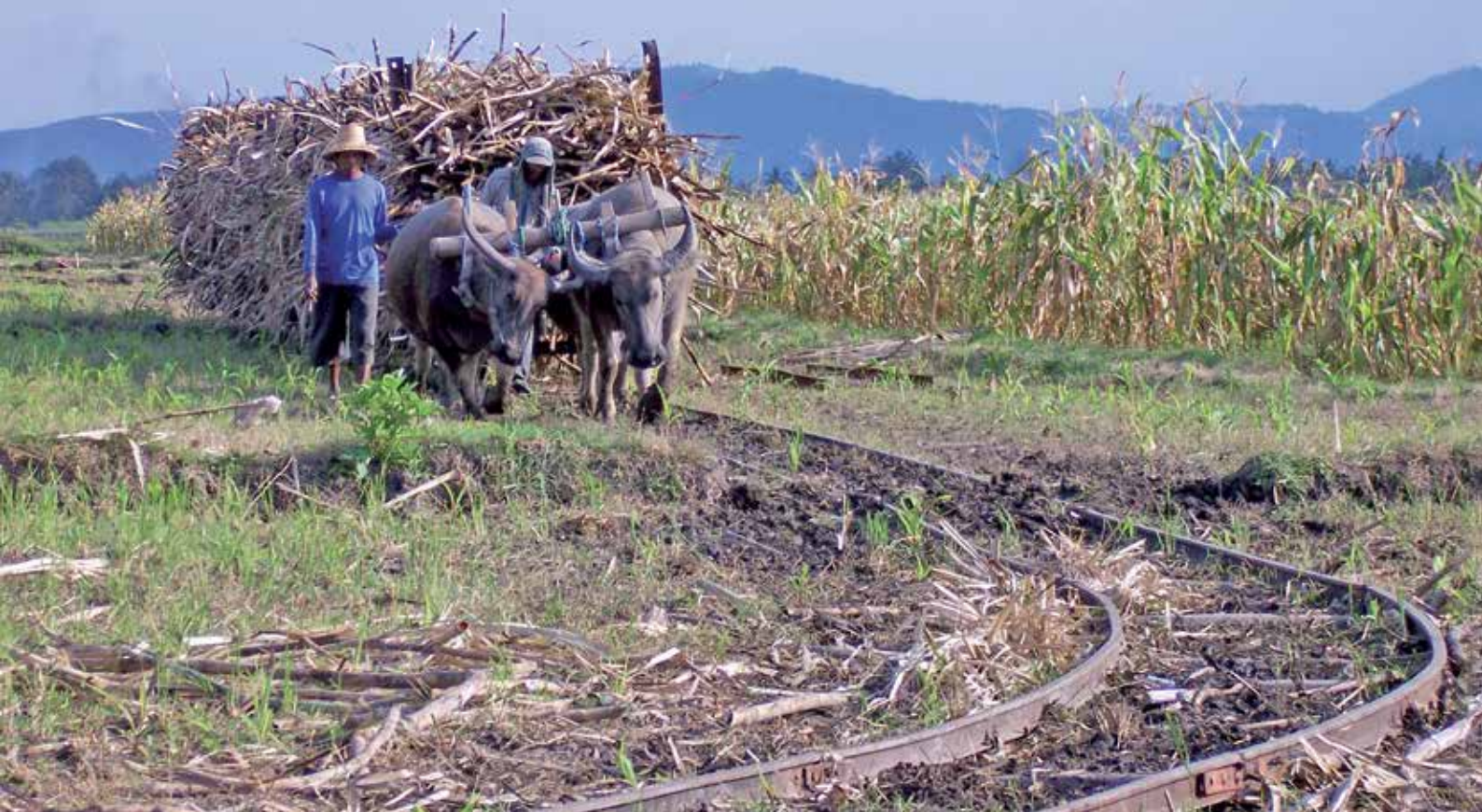
Olean Mill, Java: water buffalo pulling a single load of wholestick cane along a line constructed from portable track sections. Although the line looks to be quite well established, the ratoon cane springing up between the rails shows that the canefield was only harvested recently and the track will be moved elsewhere once harvesting moves to another area.
