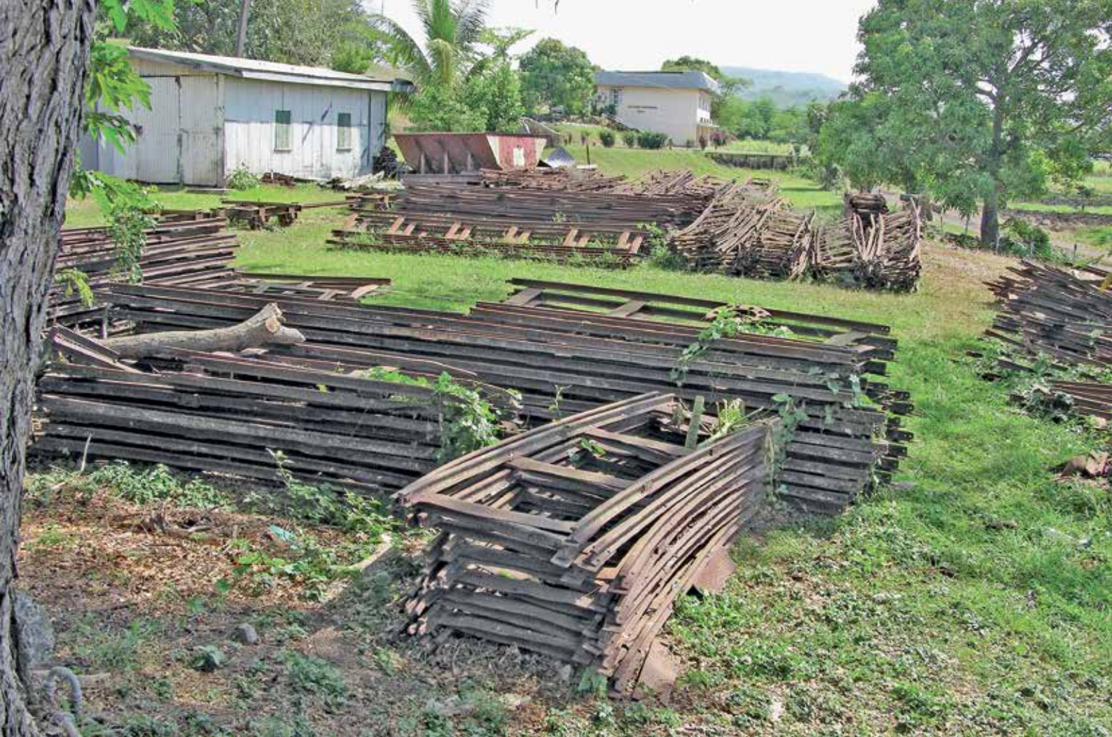
Portable track components at Tavua depot, Fiji, October 2009. Note that the track sections have a pair of fishplates at only one end of each rail.
