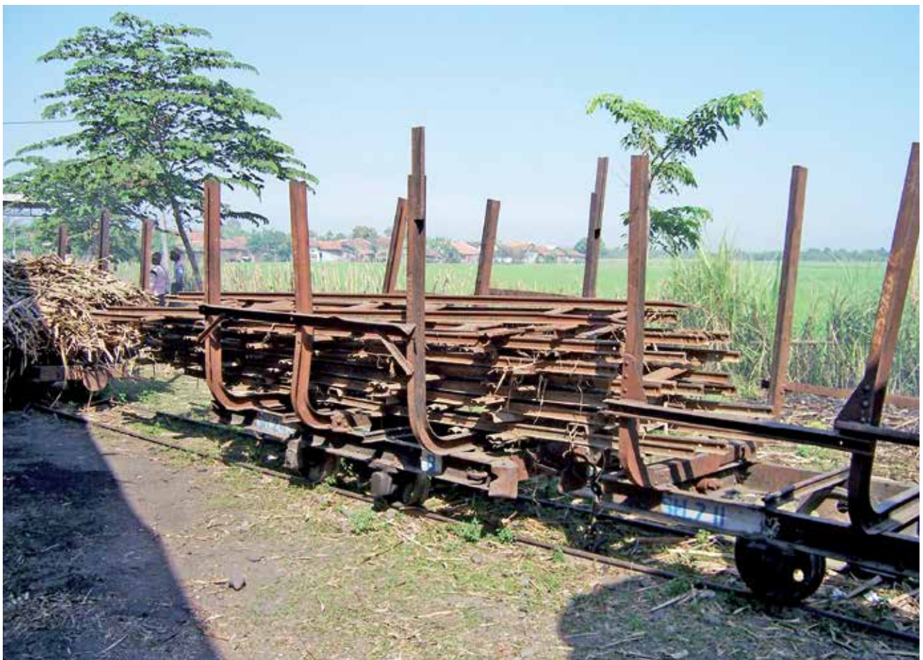
PG Sumberharjo, Java: portable track on cane truck. This mill loads its wholestalk cane longitudinally; unloading is done by sling, rather than tipping the truck. Sumberharjo still had seven steam locomotives in use in 2010 and is one of the few mills left in Indonesia to operate field lines.
