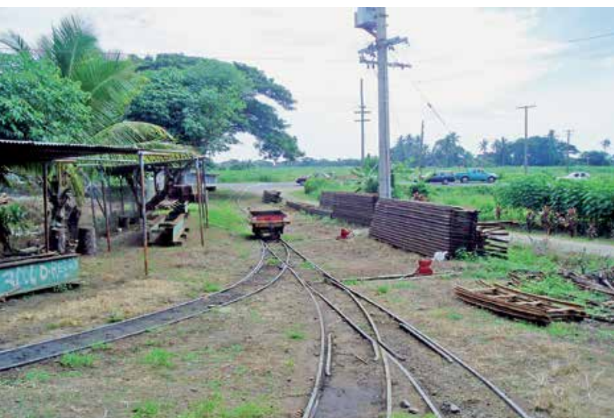
Out depot south of Nadi, Fiji, looking back towards the chain tightening gang's shed, with portable track stacked to one side, May 2010. The straight sections appear to be 7 metres long, while the curved sections are closer to 3-4 metres.
