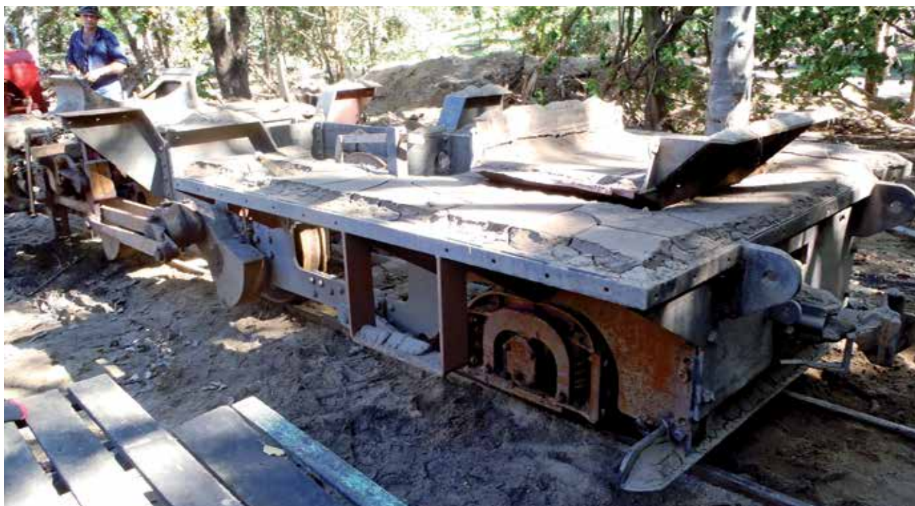
The mud-caked frames of Bundaberg Fowler 0-4-2T number 3 at the Australian Sugar Cane Railway, Bundaberg, in the aftermath of the January flood. At left of picture, volunteers are bailing water out of the smokebox saddle. Fortunately, the locomotive's boiler was off-site undergoing repairs. Photo: Ross Driver
