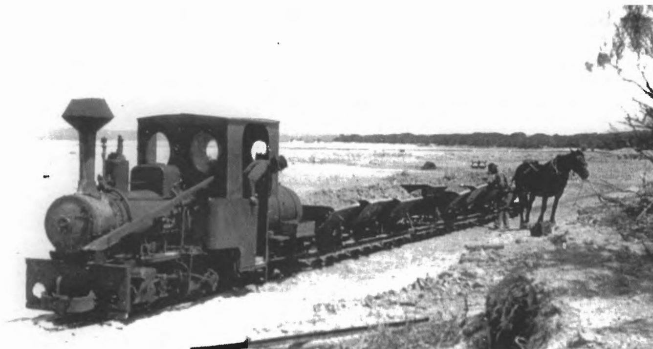
Krauss 0-4-0WT 2178 of 1889 and water gin coupled to a string of four-wheeled side-tipping wagons at Marion Lake circa 1920, during the period of ownership by A H Hasell. Photo courtesy Port Dock Railway Station Museum
