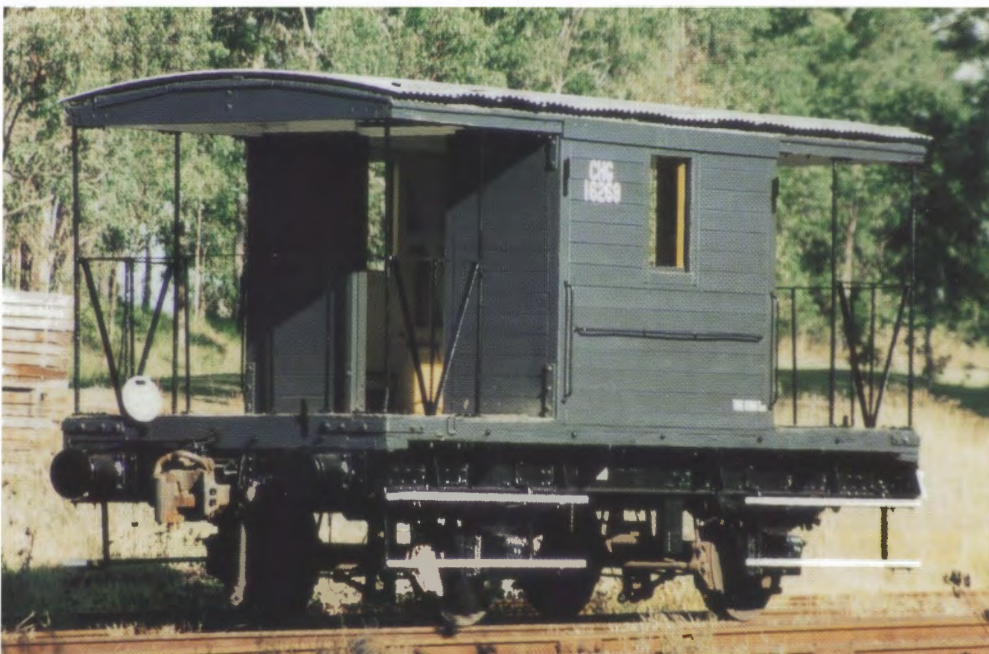
The CHG brake van was a feature on non-air coal trains on both the NSW government railways and private lines. Richmond Vale Railway has recently restored CHG 16269 and it sees regular use with 0-4-OST MARJORIE during open days.
