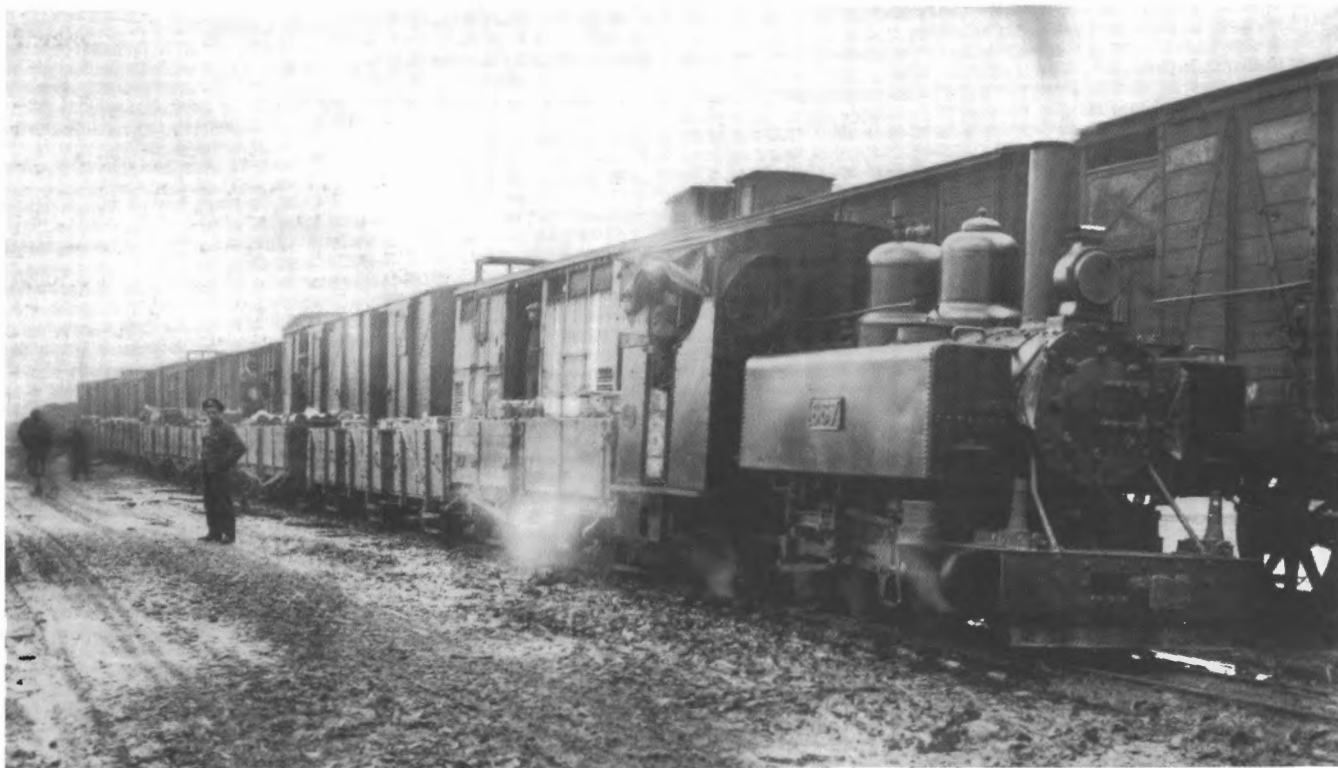
In October 1917, at Frizeville, near Poperinghe, Belgium, members of the 16th Australian Light Railway Operating Company are in the process of transferring ammunition from standard gauge wagons to their own. The Baldwin 4-6-0T, number 667 (45495 of 1917), is one of 495 such machines supplied to the British War Department Light Railways between October 1916 and April 1917. Photo: Australian War Memorial C1357
