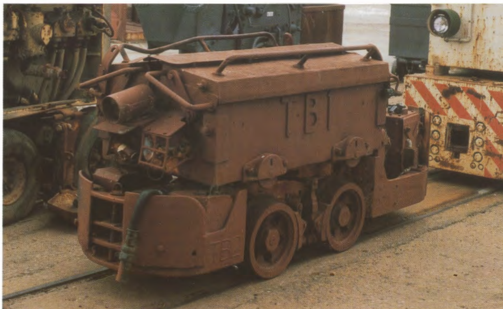
4wBE mine locomotive TB2 (carrying the battery box of TB1) at the Line of Load Museum, Broken Hill. Photo: Ray Graf
