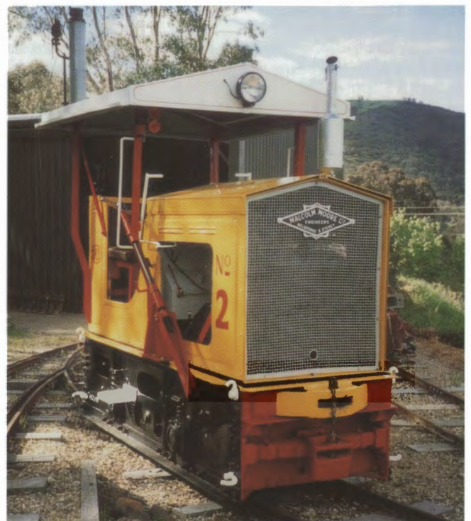
The restored Malcolm Moore locomotive, with new brake equipment prominent
