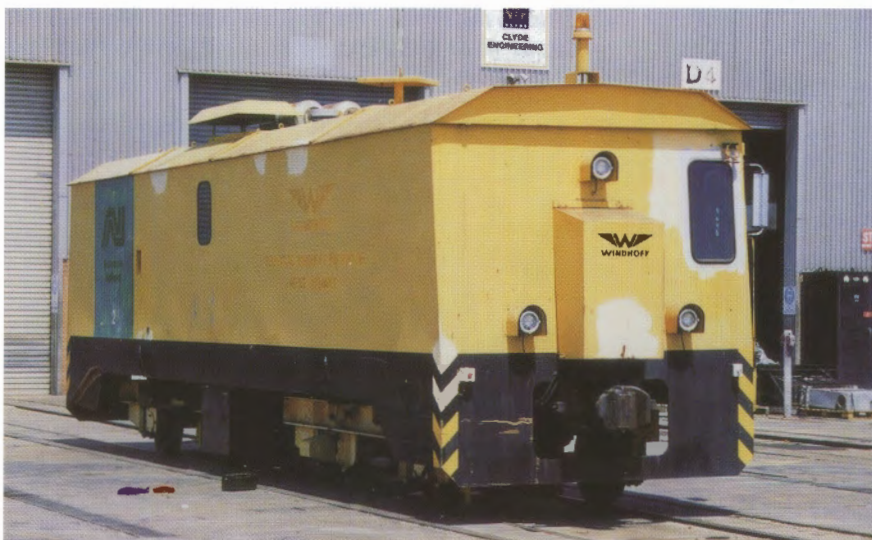
Windhoff 4wDH of 1982, the workshops shunter at Clyde Engineering, Port Augusta, on 8 February 2001. This standard gauge unit was originally used under remote control at ANR's Dry Creek bogie exchange facility. Photo: Brad Peardon
