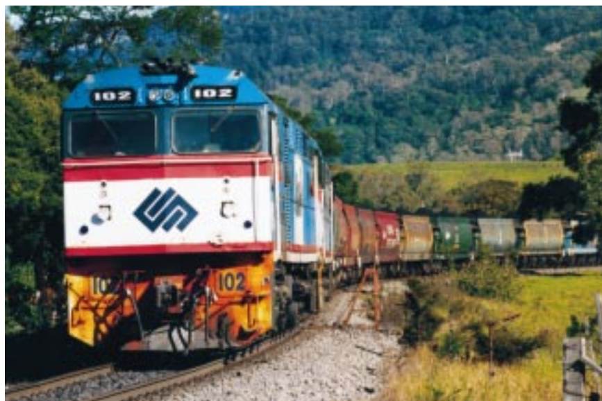
BHP Port Kembla's leased A E Goodwin Co-Co DE locomotives 102 (G-6048-13 of 1972) and 101 (G-6048-09 of 1972) with an up coal train at Wongawilli Village, 30 May 1998. Photo: Brad Peadon
