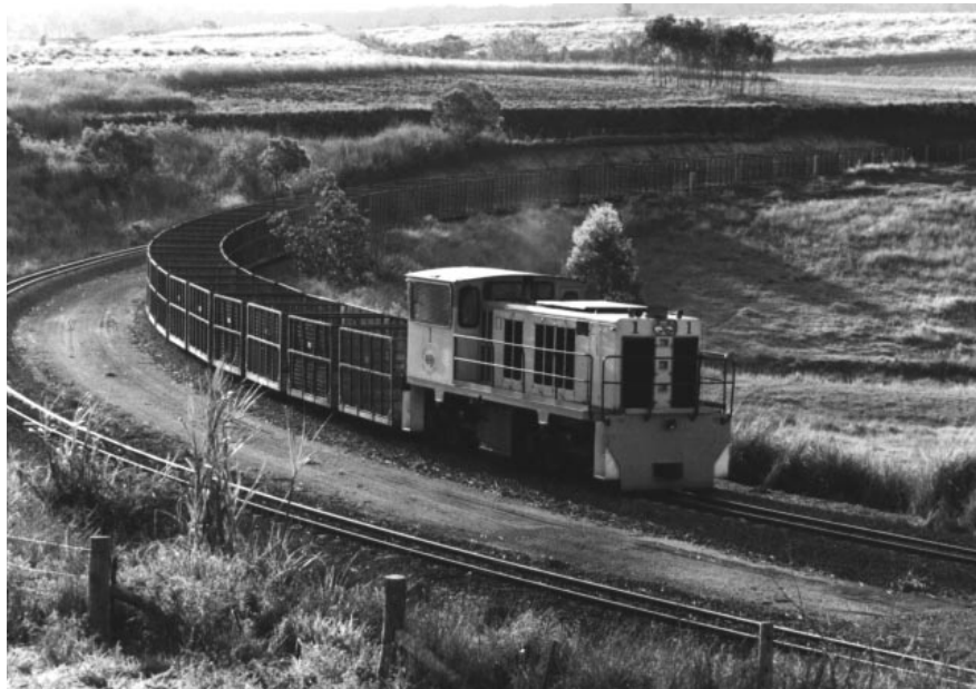
Isis Mill: 2ft gauge Walkers B-B DH 1 (602 of 1969; rebuilt Walkers 1991) hauls empty bins up the grade from the mill, 15/10/96. Photo: Brad Peardon
