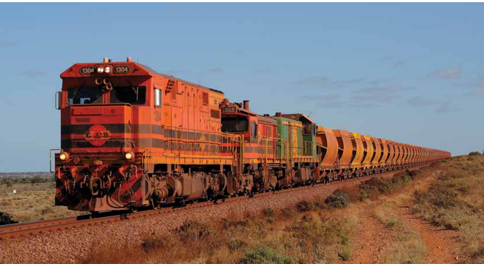
Arrrium ore train No. DW28 approaches Whyalla on 23 April 2013, with a typical mixture of ageing motive power at the head, comprising MKA unit 1304, Goodwin/Alco 904 and Clyde/EMD CK3. 1304 is a 1993 MKA rebuild of 1961-vintage ex-BHP Clyde/EMD locomotive DE 07. Photo: Andrew Rosenbauer
