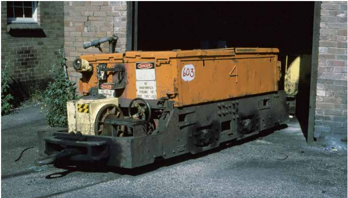
A Jeffrey type 4wBE locomotive built by Gibson Battle, carrying battery box number 4, photographed at Lithgow Valley Colliery on 3 January 1979, following the mine's closure. Note the link and pin coupling.
