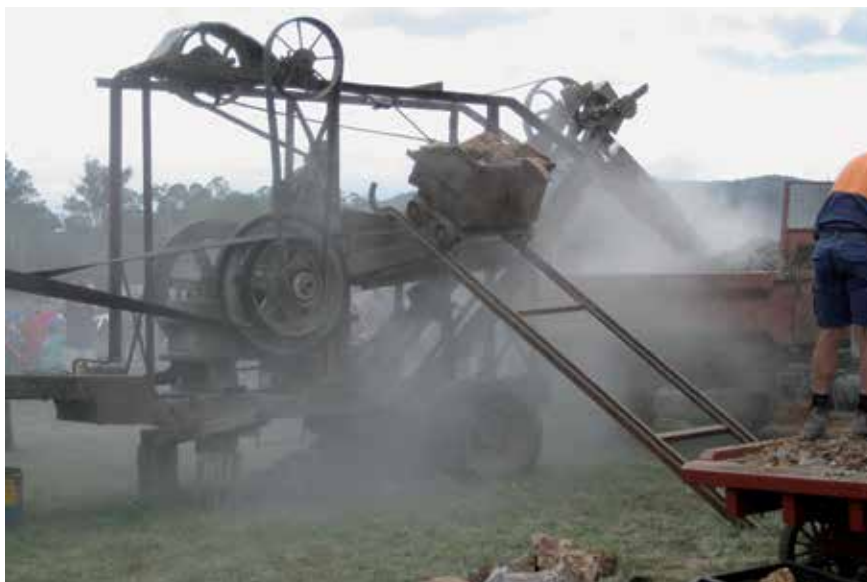
The remarkable steam-powered rock crusher, fed by a four-wheel skip on a short railed incline, in full flight at the 19th annual SteamFest Rally, at Sheffield.
