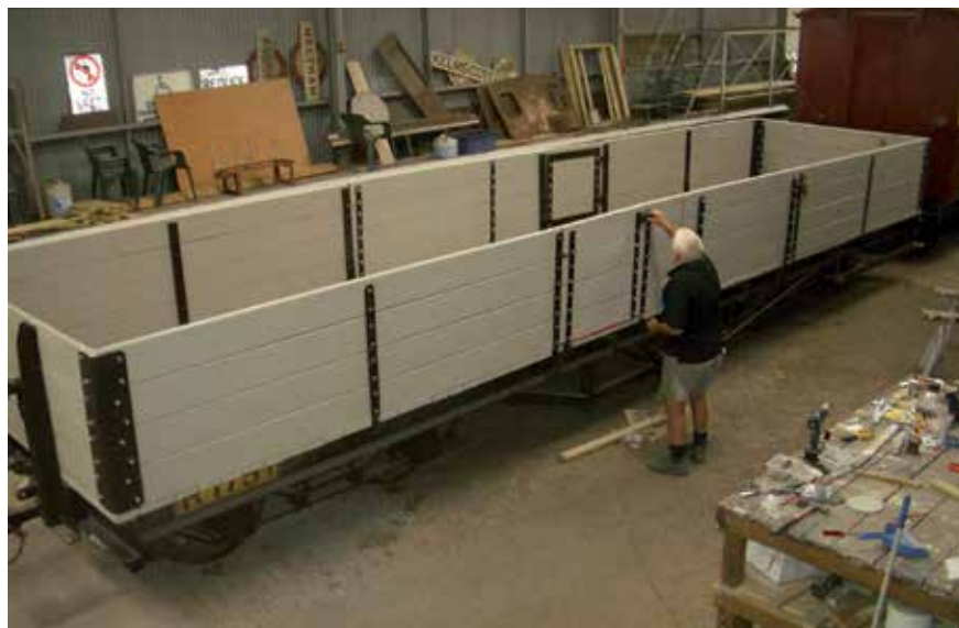
R 1751, an Oldbury C&W Co. product of 1894, regauged and rebuilt at the Mussel Pool workshops. Volunteer carpenter, Clarie Iopollo, is seen finishing off the woodwork. The regauging work was led by Michael and Lindsay Watson. Photo: Lindsay Watson
