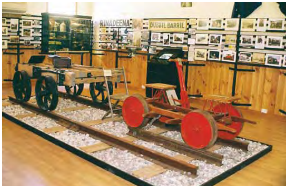
The displays at the Mt Lyell Abt Railway Society's museum in Queenstown railway station on Tasmania's West Coast. Featured in the centre are a 610mm gauge hand-operated fettlers' 'trike' and the 1067mm gauge fettlers' trolley behind was recovered the banks of the King River and restored by Society volunteers. Photo: Peter Ralph
