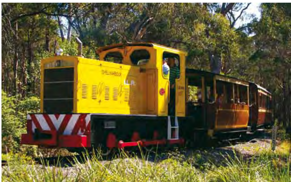
0-6-ODH SHELLHARBOUR (John Fowler 21912 of 1937; rebuilt EM Baldwin 1963) heads a train around the loop at the Albion Park Train Park during 2009.
