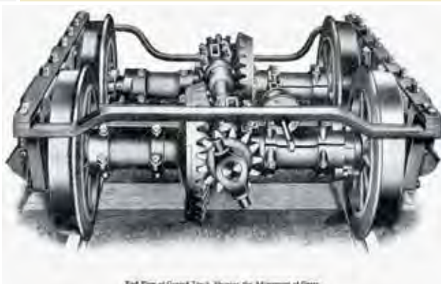
End View of Geared Truck, Showing the Adjustment of Gears
