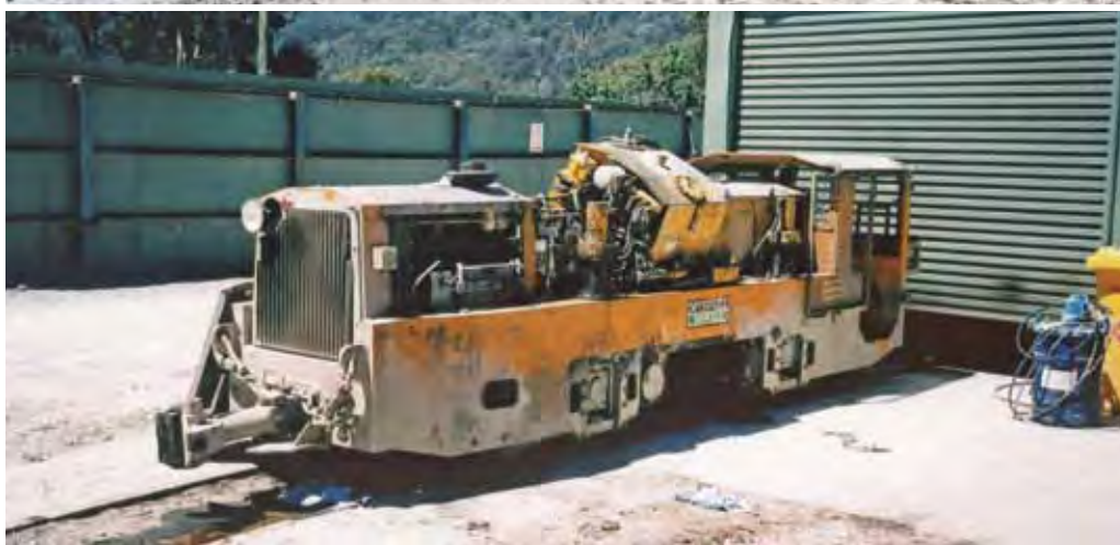
Above: The Clayton 4wDH and personnel carrier. Left: The F&M Baldwin 4wDH rack loco under repair. Below: The 8-wheel cement carrier and spraying tender. All photos: Simon Moorhead
