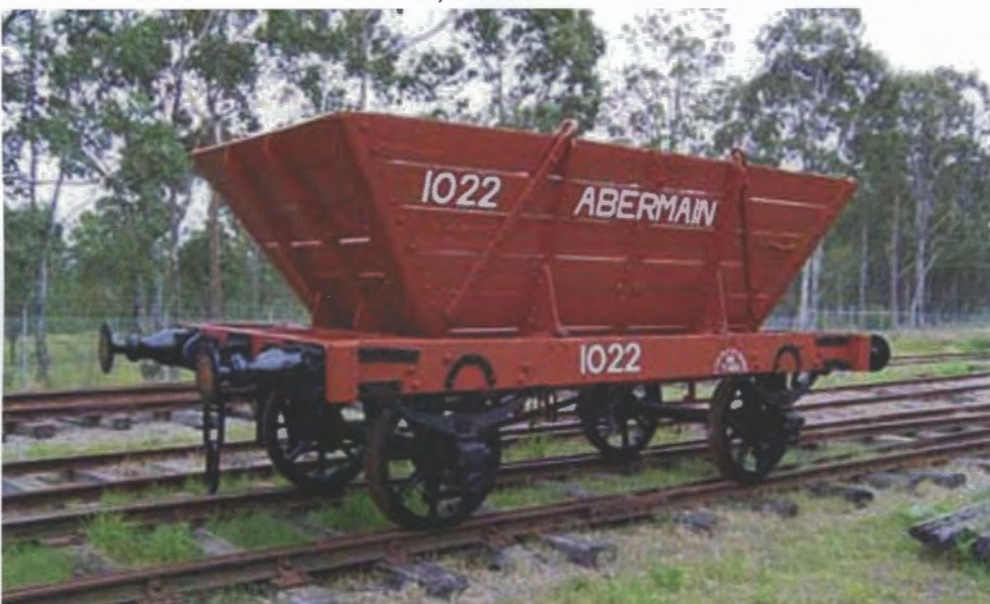
The Richmond Vale Railway has recently completed the restoration of wooden underframe 10-ton capacity non-air hopper 1022, built by A Goninan & Co at Broadmeadow in the early 1920s. Photo: Graham Black
