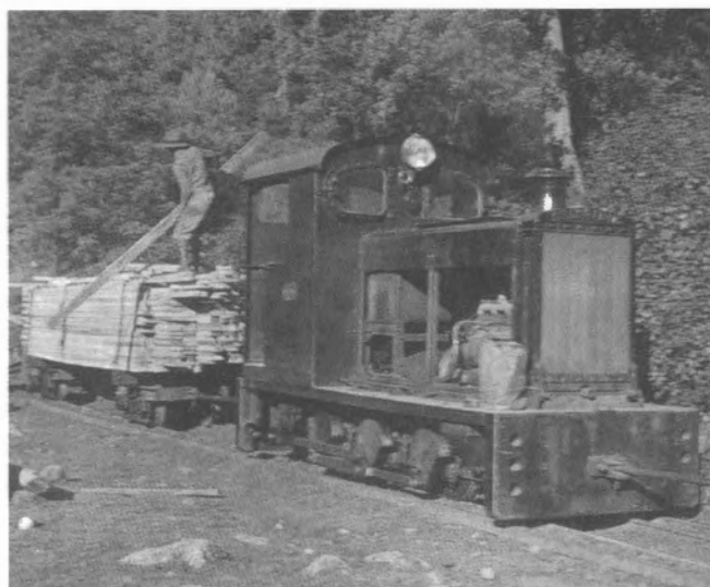
At Tin Hut on 11 February 1938, Kelly & Lewis 5957 waits as its driver prepares to insert a twitch plank to tighten the chains on a load of timber. Photo: WRB Johnson, from Mike McCarthy collection
