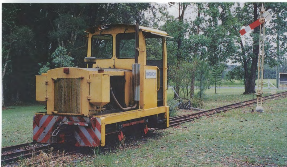
Former Moreton Sugar Mill 0-4-0DH MAROOCHY (EM Baldwin 6/1064.1.11.64 of 1964) at its new home at Eudlo, 19 November 2004. Photo: Clive Platter
