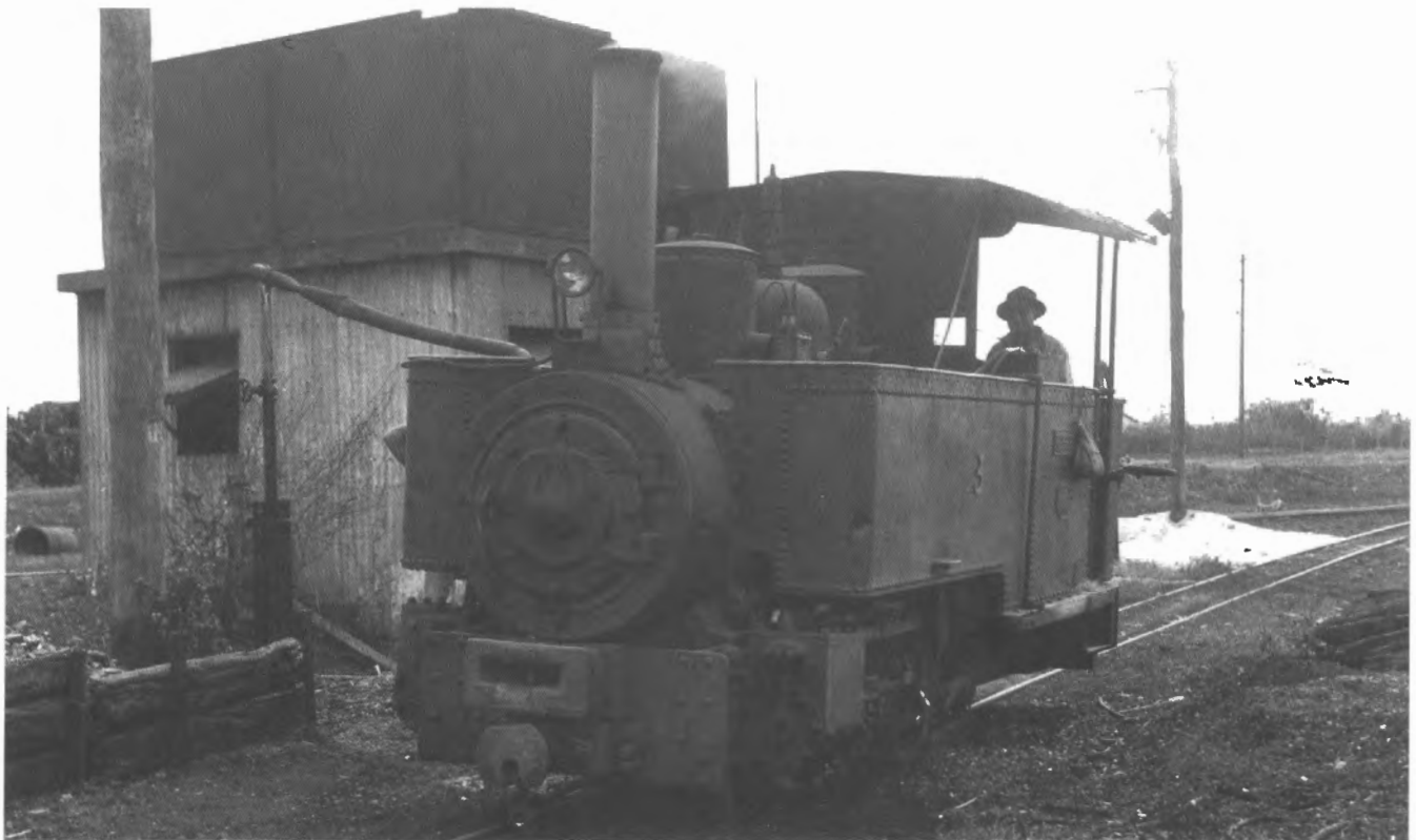
Taking water, in November 1946, is the locomotive first worked on by the author, John Fowler 0-4-2T 3 RUSSELL (14458 of 1915). The upper coupling pocket is to allow Innisfail Tramway stock to be handled.
