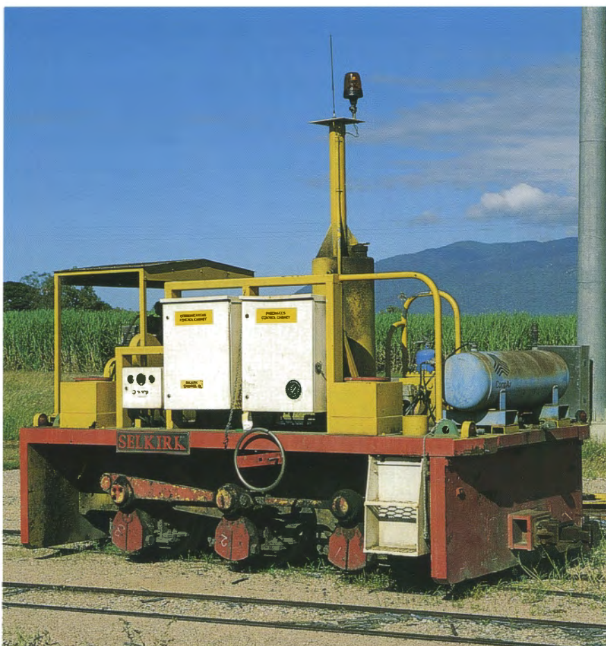
Invicta Mill's brake wagon SELKIRK was built from the chassis of Com-Eng 0-6-0DH SCOTT (C1015 of 1957) in about 1985 and is seen here in the mill yard on 19 March 2002. Photo: Scott Jesser
