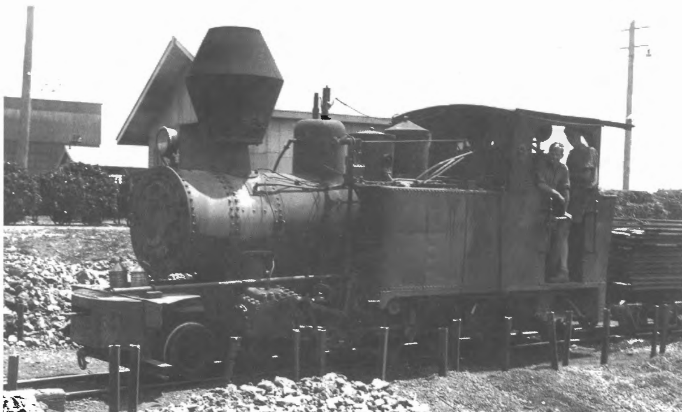
Ex British War Department Light Railways Hunslet 4-6-0T 9 (1250 of 1917) is in use hauling portable track at the mill in November 1946. Many local modifications have been carried out including extended smokebox, new smokebox door, spark arrestor, additional sandbox, rear cab roof extension, electric headlight and additional front buffer casting, not to mention the extra plumbing. Number 9 was a regular Silkwood loco from the late 1930s until the mid 1940s. It was retired in 1953.
