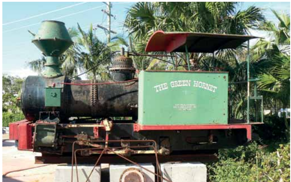
Former Timbertown, Wauchope 0-6-0T THE GREEN HORNET had been more or less 'off the radar' since being sold at auction in 1999, so Ian McNeil was surprised recently to discover it on display outside The Railway Lodge Motel at Taree, on the NSW mid-north coast. Before working at Timbertown, the 1910-vintage Fowler (B/N 12271) had been CSR's Macknade Mill number 8, and before that, Goondi Mill number 5 'The Flying Piecart' (see LR 219, page 18).
