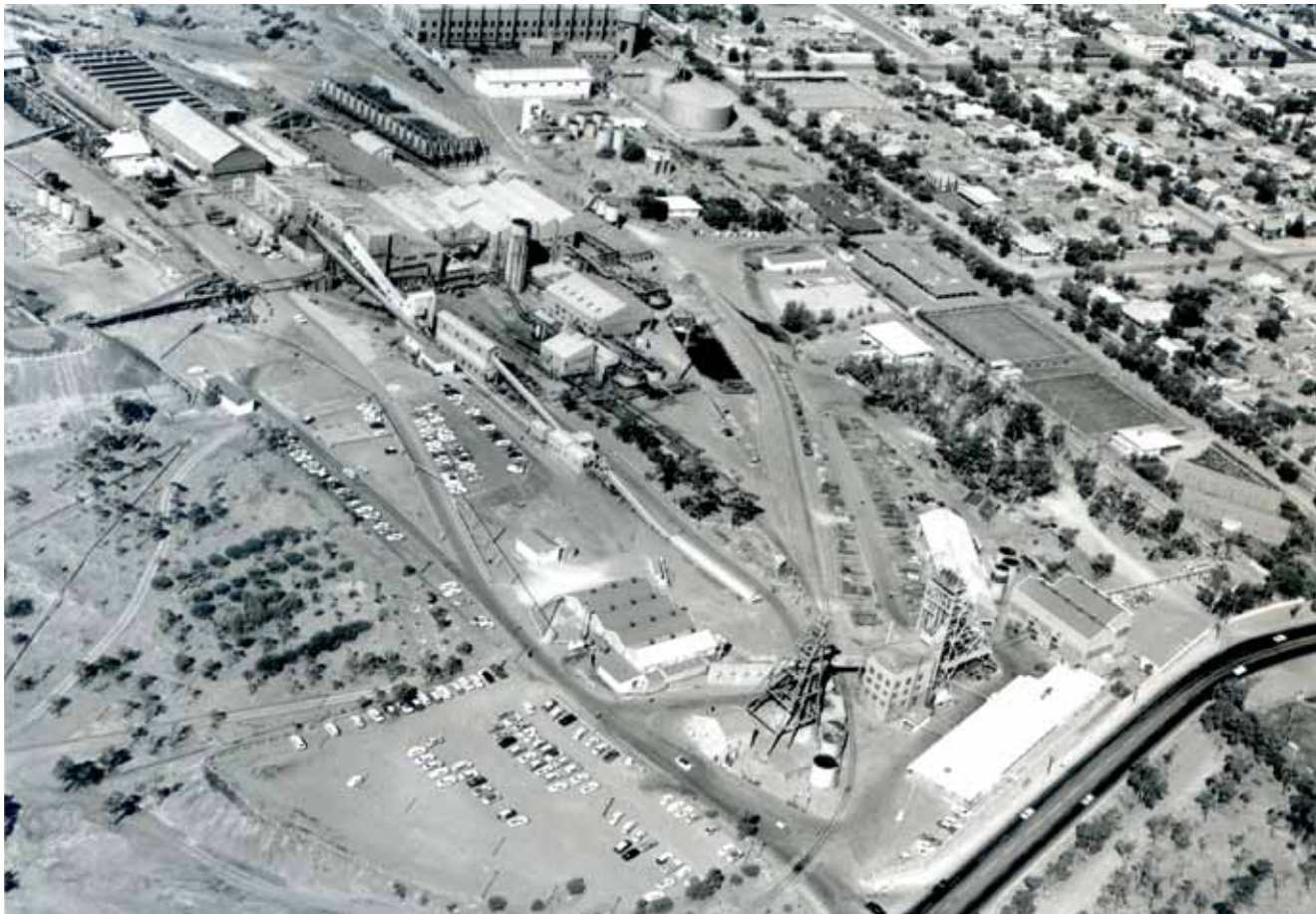
Located along a ridge on the southern flank of the Broken Hill, this is an aerial view of the Broken Hill South mine (dated 1967) looking east. In mid foreground, the South Road passes by the steel headframe of No.7 shaft (2,478 feet deep) which stands to the right of the obsolete timber headframe of No.4 shaft. The mine's branch line off the Silverton Tramway bisects the two. In mid centre, mill buildings can be seen while at top centre the "Central Power Station" building is visible with its attendant diesel fuel tanks. The township of South Broken Hill, once known as Alma, lies on the right of the photo.
