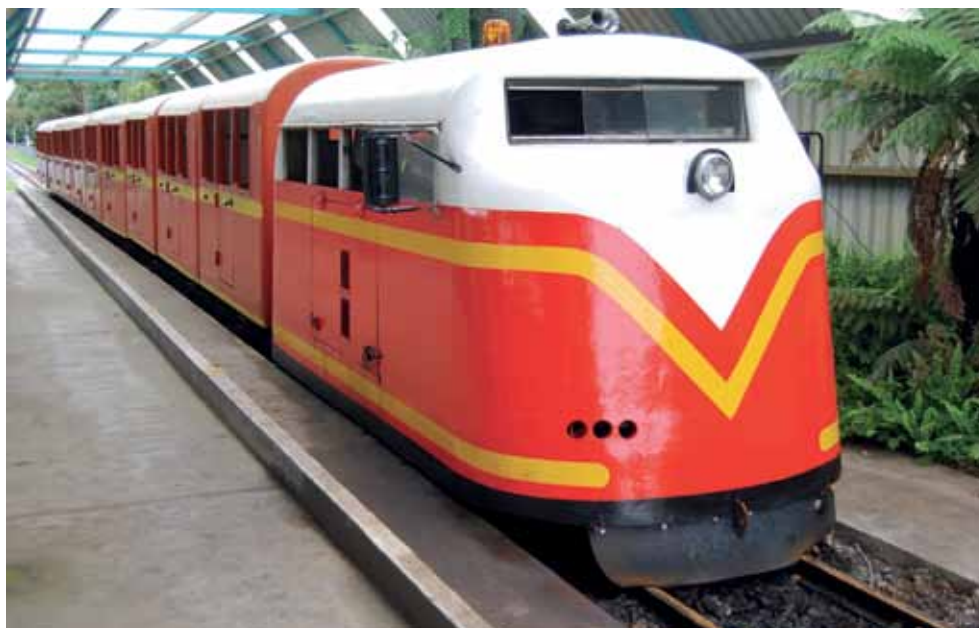
With the track newly upgraded at the Caribbean Gardens Railway at Scoresby, the fibreglass-bodied train was looking clean and fresh when photographed at Grand Central Station by Peter Evans on 22 June 2011. The locomotive is a converted 'Simplex' bow-frame 4wDM locomotive, believed to be Motor Rail 3711 of 1924.
