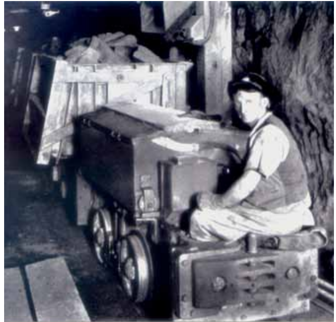
The first storage battery locomotive to be put to work at Broken Hill South was a 24 inch gauge Greenwood and Batley 3-ton unit. Pictured here, the 'electric mule' is hauling a rake of Granby cars. The 'mule driver's' cockpit offers minimal protection.
