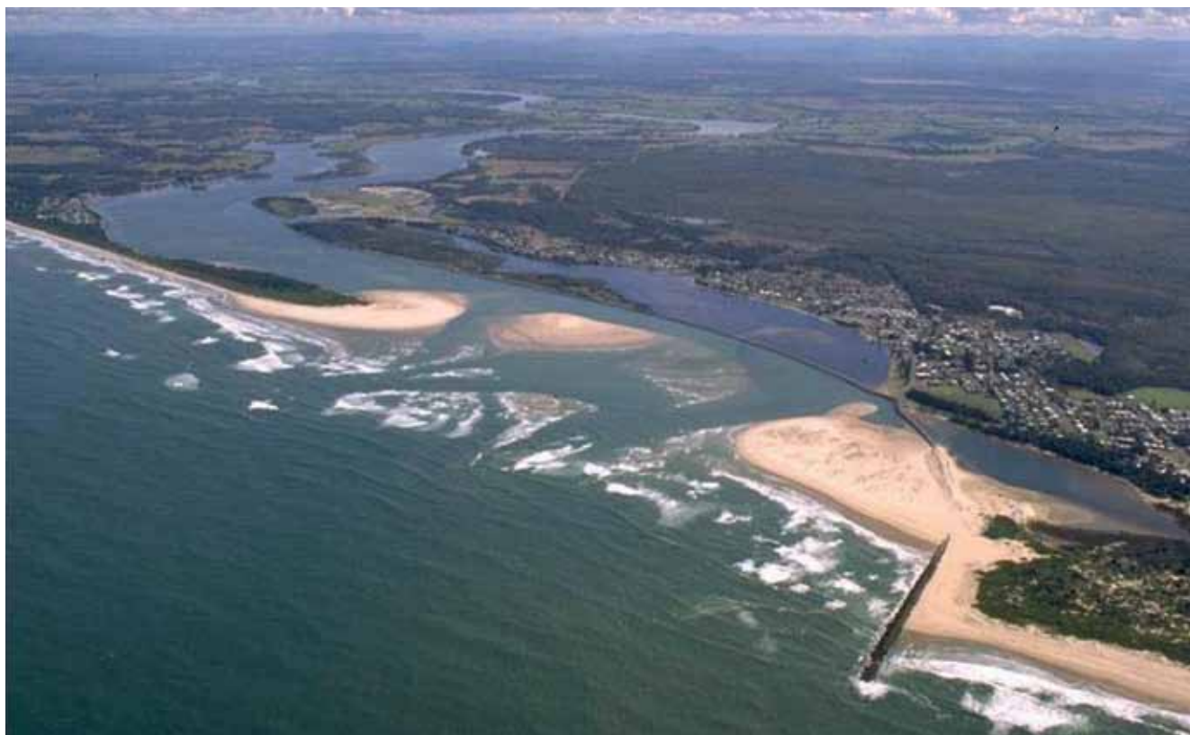
An aerial view of the Manning River entrance after winter storms. The navigation channel alongside the breakwater wall is completely blocked by sand and the river has broken new exit channels through the washed-out remnants of the tip of Mitchell's Island. This is what the old PWD dredges battled against for years, and what the never-built southern breakwater was supposed to prevent.
