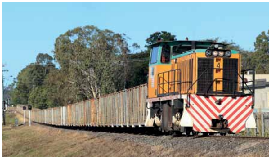
Plane Creek Mill's Walkers B-B DH 4 CARMILA (676 of 1971 rebuilt Bundaberg Foundry 1996) passes 'Zero Loop' in Sarina on 20 June with 231 loaded bins and brake wagon BV1. Photo: Scott Jesser
