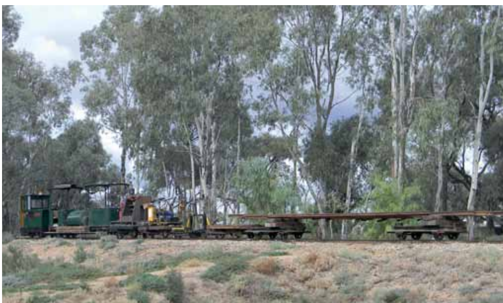
The work train heads out on the track extension from Cobdogla towards Loveday loaded with components for a points set. Simplex FARLEIGH, guard's van, tool wagon, flat top carrying the dog spike puller, rail bender, match truck and bolster wagons with components. The setting is the track along the top of the Humphrey Pump channel. The trees in the channel have all grown since the museum was formed.
