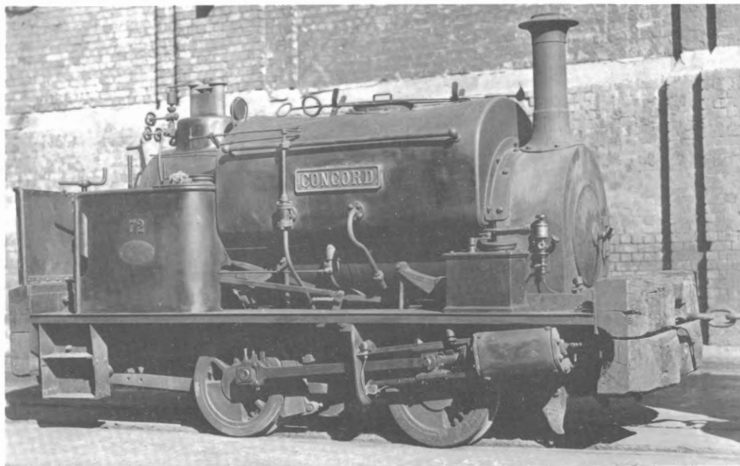
Typical of the Hudswell Clarke cableless 0-4-0ST locos Concord No. 72 (B/No. 1560 of 1925) posed for its portrait at AGL Co Mortlake gasworks circa 1937. Photo: AGL Co
