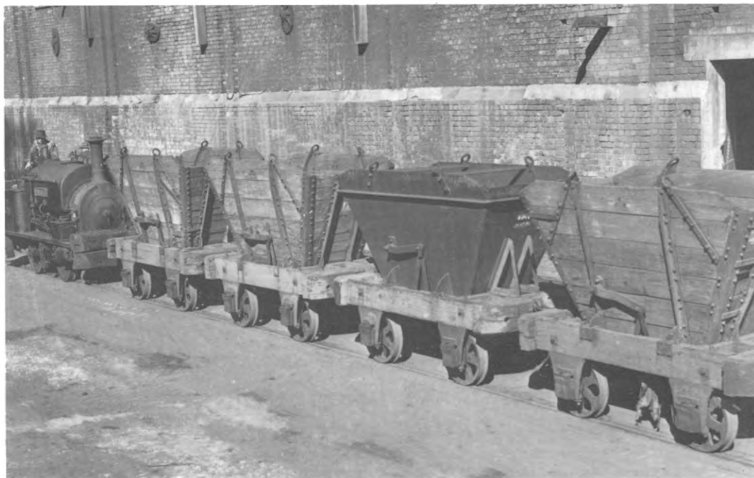
Typical of the drop-bottom hopper wagons with lift-out hoppers as used for coal haulage on the AGL railway at Mortlake with a rake coupled to the Hudswell Clarke loco Concord probably circa 1927.
