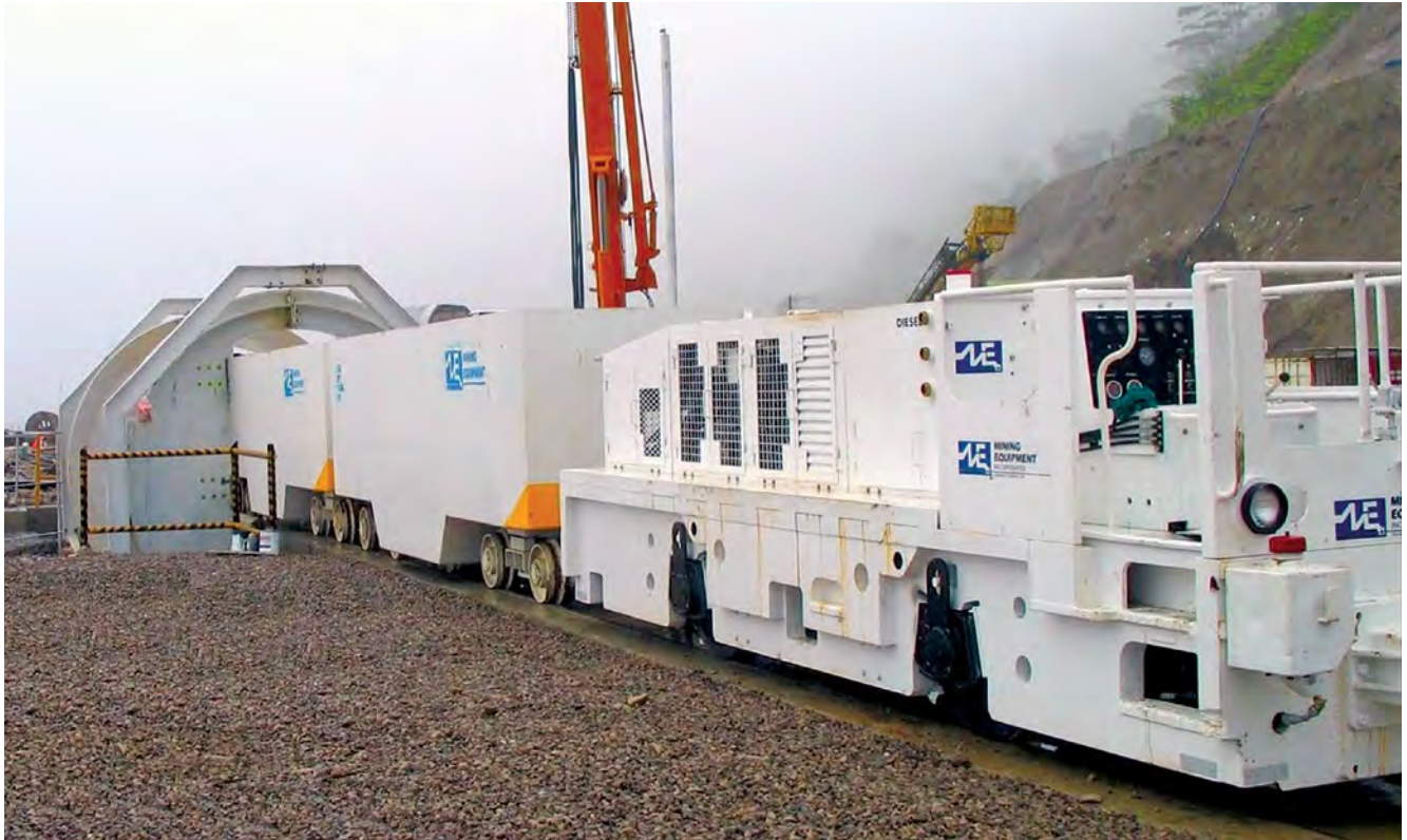
High in the mists of the Star Mountains, the muck tipping facility at Papua New Guinea's Ok Tedi mine, dumping MEL bogie rollover muck bins shunted by one of the two ex-TML Schöma CFL150DCL, this one with some significant modifications - an extra ballast slab on the deck-plate and an 'alfresco' open cab. Photo: Courtesy Mining Equipment Ltd.
