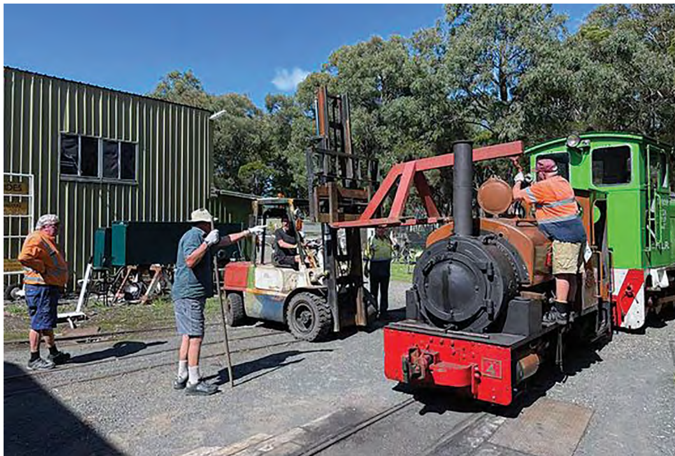
At Albion Park Burra is having its saddle tank removed as part of its ongoing restoration. Photo: Brad Johns
