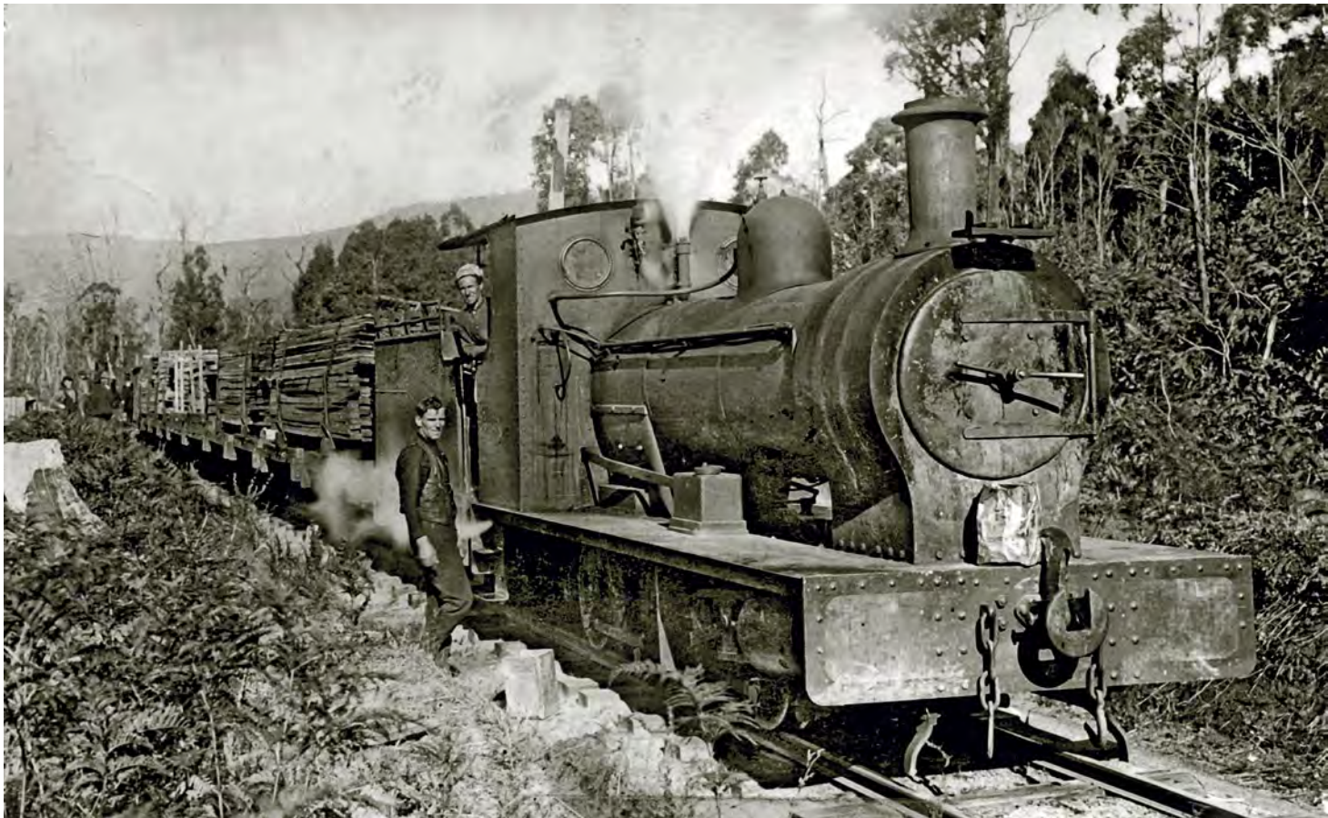
Above: Powellite, an 0-6-0 Bagnall locomotive hauling timber on the Powelltown tramway near Gilderoy in the 1930s.
