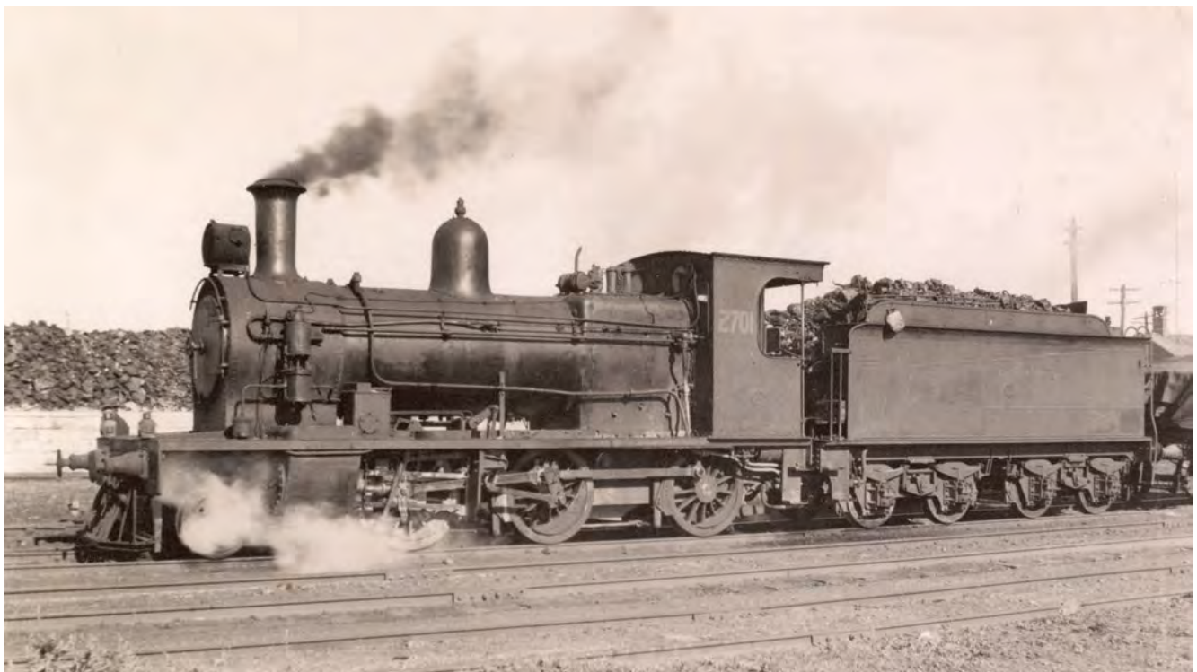
PWD locomotive No 1 became NSWGR G class No. 1204, and 2701 in the 1924 renumbering. From 1929 the eight members of the class were progressively rebuilt with standard 'B' class boilers and fitted with 'T' class tenders, as seen above. Photo: ARHSnsw RRC – Neg No 854272
