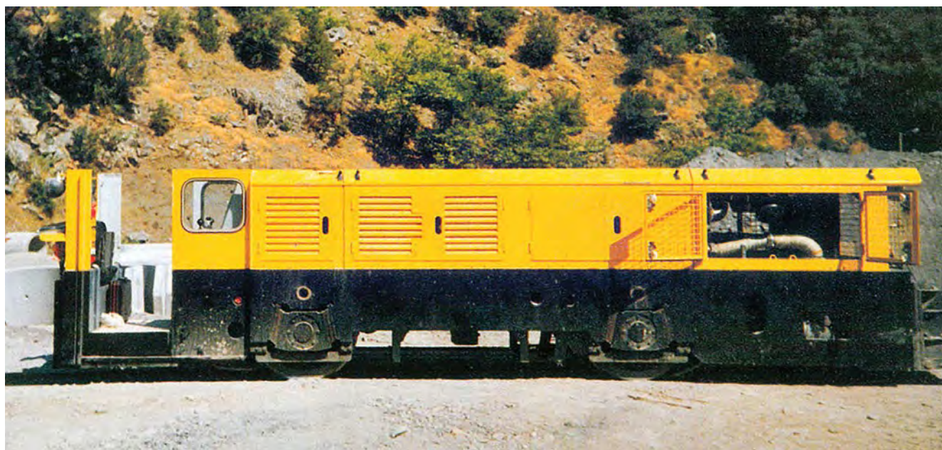
On site in Greece, one of the potential Auckland low profile CFL180DCL tunnel locos displays the roofless driver's position and the provision for track brakes - to be fitted in the slot between the driving axles. The prominent pipe in the engine compartment leads down to the exhaust scrubber apparatus in the forward section of the underframe. Photo: Courtesy Schöma Official
