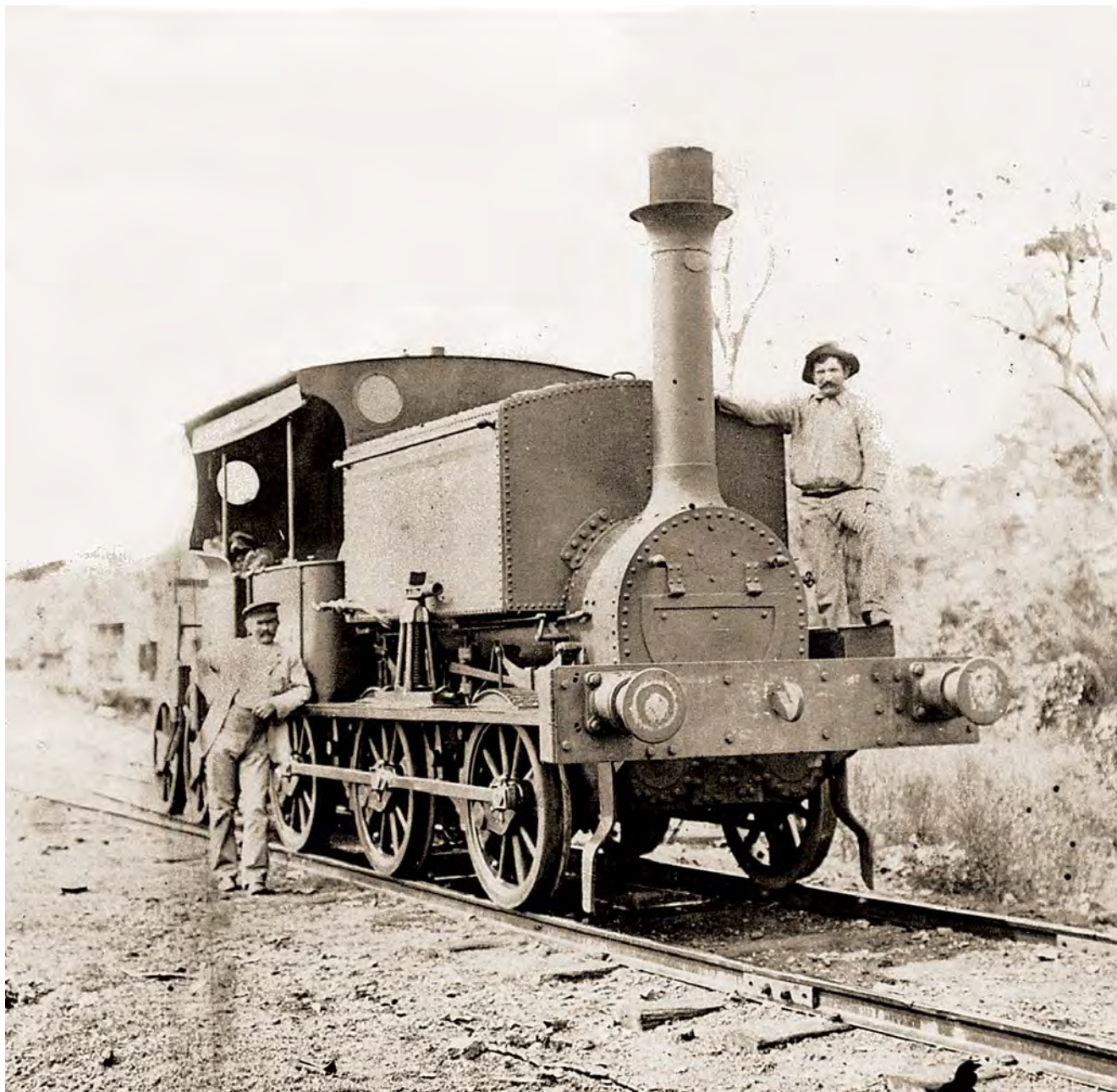
Above: No. 19 while working as an 0-6-0 at South West Rocks, 1908. The funnel extension had been installed while the locomotive was working on the Kogarah-Sans Souci tramway to above the height of the end loading carriages then in use. Photo: Mitchell Library collection
