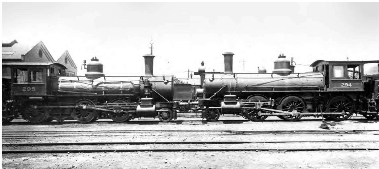
Comparison between NSWGR No. 295, on left, fitted with normal diameter driving wheels; and NSWGR No. 294, on right fitted with larger 55in diameter driving wheels for faster running, date unknown. Photo: ARHSnsw RRC collection 009887
