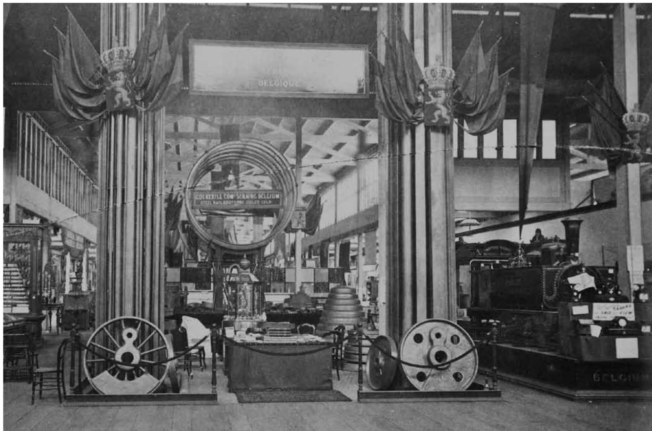
This photo of the Belgian Court at the 1880 Melbourne International Exhibition clearly shows the Couillet 600mm gauge 0-4-0T locomotive (B/N 421 of 1879) on the right.
