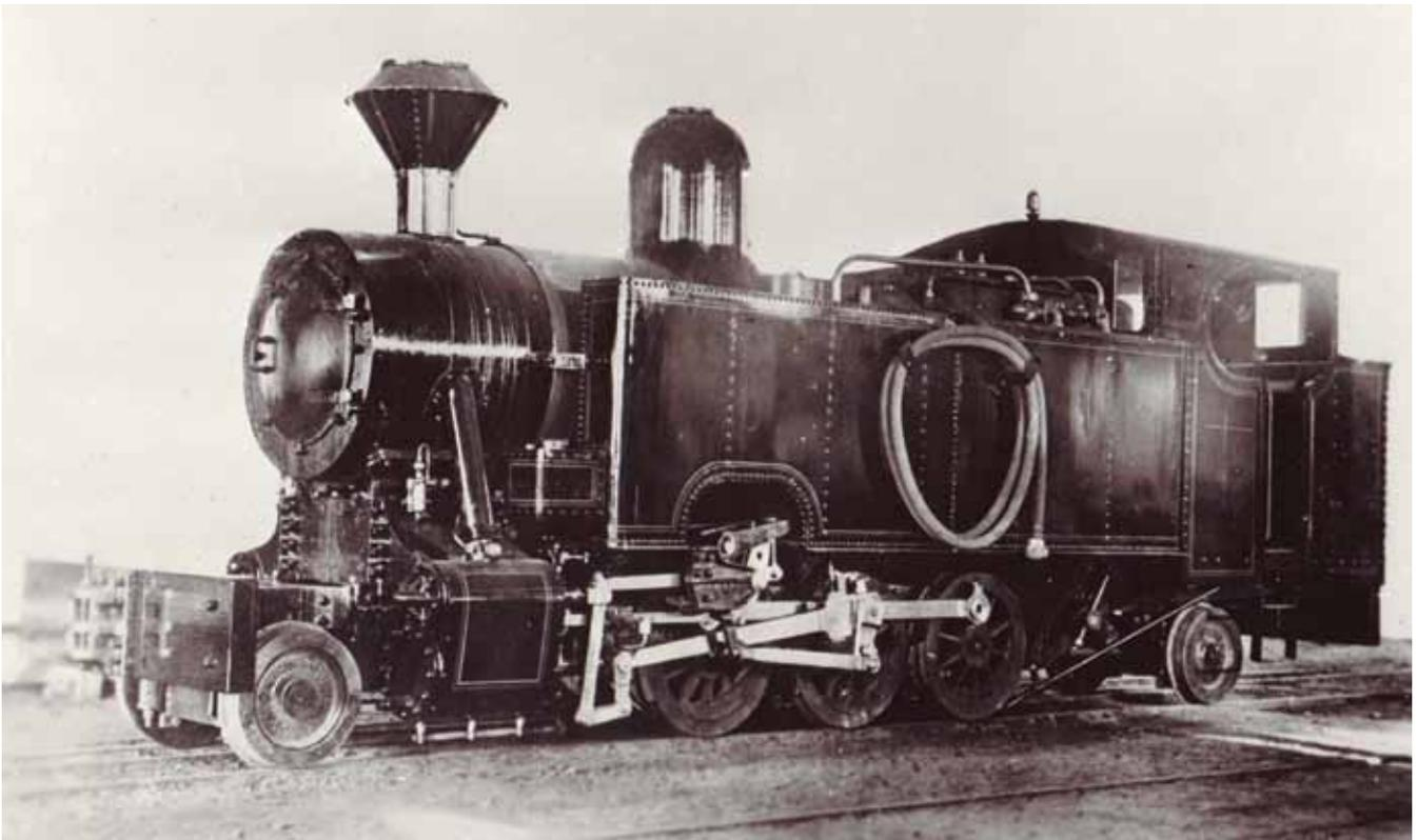
Allen Taylor's third locomotive was Clyde-built 2-6-2T Wootton (241 of 1919). Although a powerful loco, her 40-ton weight and rigid wheelbase were too much for the light rails and sharp curves of the Wootton Tramway. Less than three months after purchase, the company began making plans to dispose of the locomotive.
