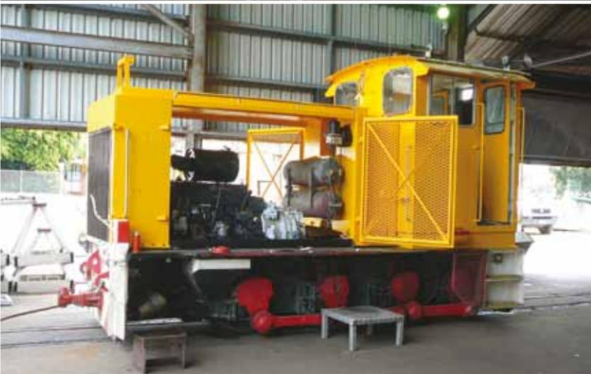
**Above:** The rebuilding of a Walkers B-B DH locomotive was progressing well in the Tully Mill loco shed on 23 March with work on the QR's former DH36 (618 of 1969) having reached the stage of the engine being placed in position. TULLY-11 (Com-Eng 0-6-0DH Ad1347 of 1960) looks on. Photo: Luke Horniblow
