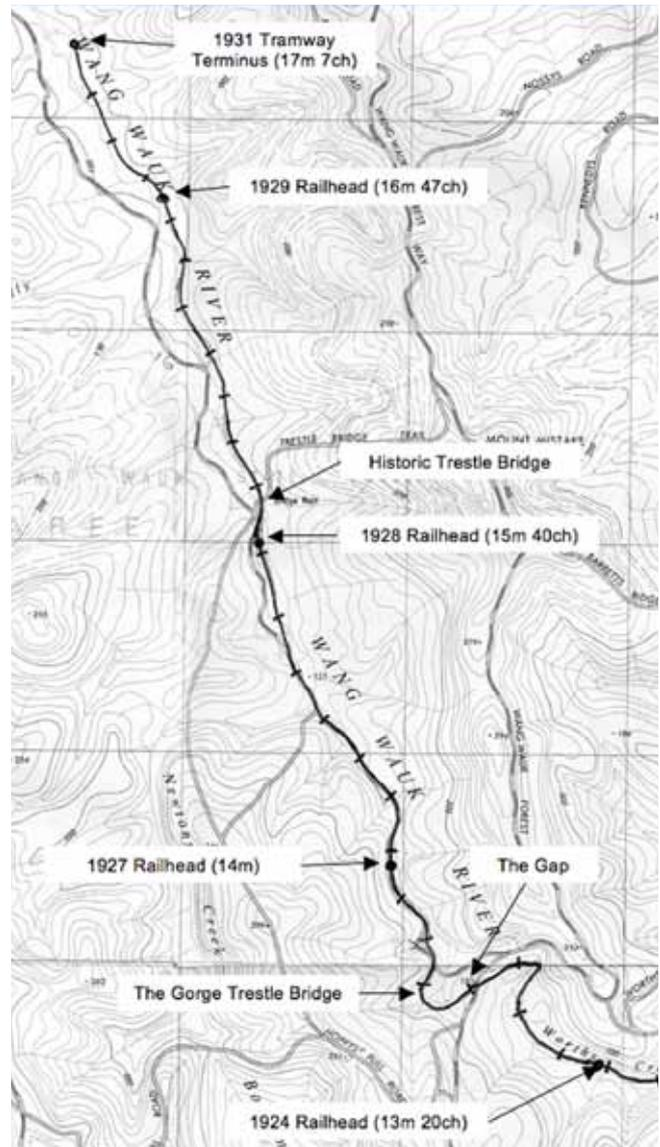
The *Wootton* Timber Tramway reached the headwaters of *Worths* Creek in 1924. Extending the tramway into *Horses* Creek valley began three years later. There were steep gradients on both sides of the dividing ridge, which was crossed at a point known as *The Gap*. Three large trestle bridges were constructed just north of this point. The final railhead was reached in late 1931.
