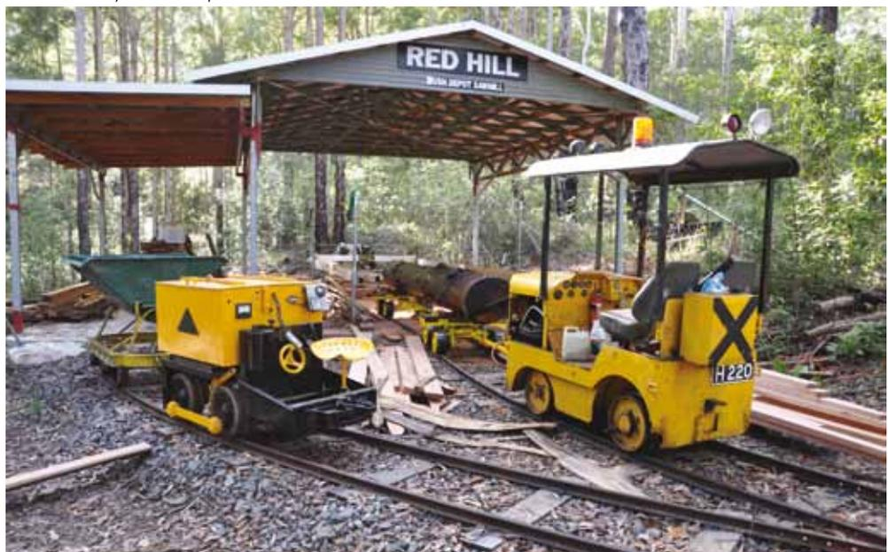
4wPM (built by Russell Savage in 1983) H220 shunting a new log into the Tinbeerwah Mountain Railway's Bush Mill in April 2010. The Wingrove & Rogers battery-electric loco 2216 of 1942 (ex Smithfield Magazine, Adelaide, see LR 148, pp.10-15) is on sawdust removal duty. Photo: Russell Savage
