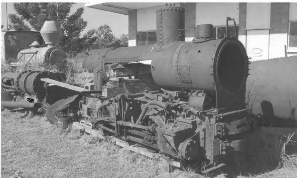
The remains of centenarian 0-4-DWT Jung 1052 of 1906, originally used on the Japoon Tramway in far north Queensland, at Graham Chapman's storage site in a northern Brisbane suburb on 10 April. Graham plans to restore it to working order at his new premises at Narangba. Fowler 0-4-2 17683 of 1927 in the background is for sale. Photo: John Browning
