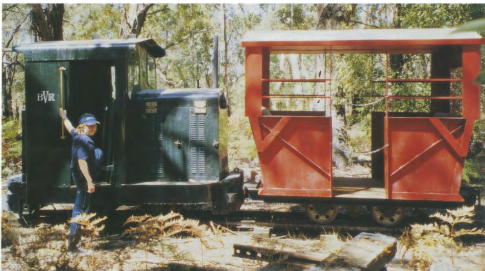
Co-owner Jack Loney with the ex-Cheetham Salt Works Ruston & Hornsby 4wDH locomotive and four-wheel passenger carriage at the new Gherang Gravel Tramway near Geelong. The loco still has its Bass Valley Railway logo. Photo: Peter Loney
