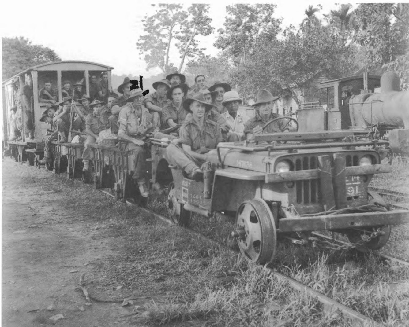
On 22 July 1945, a jeep locomotive prepares to leave Beaufort with 'The Membukut Special', as this particular run was known. The steam locomotive on the right is most likely Kerr Stuart 4-6-0 EMPIRE (B/N 1227 of 1911). Photo: Australian War Memorial No. 111845
