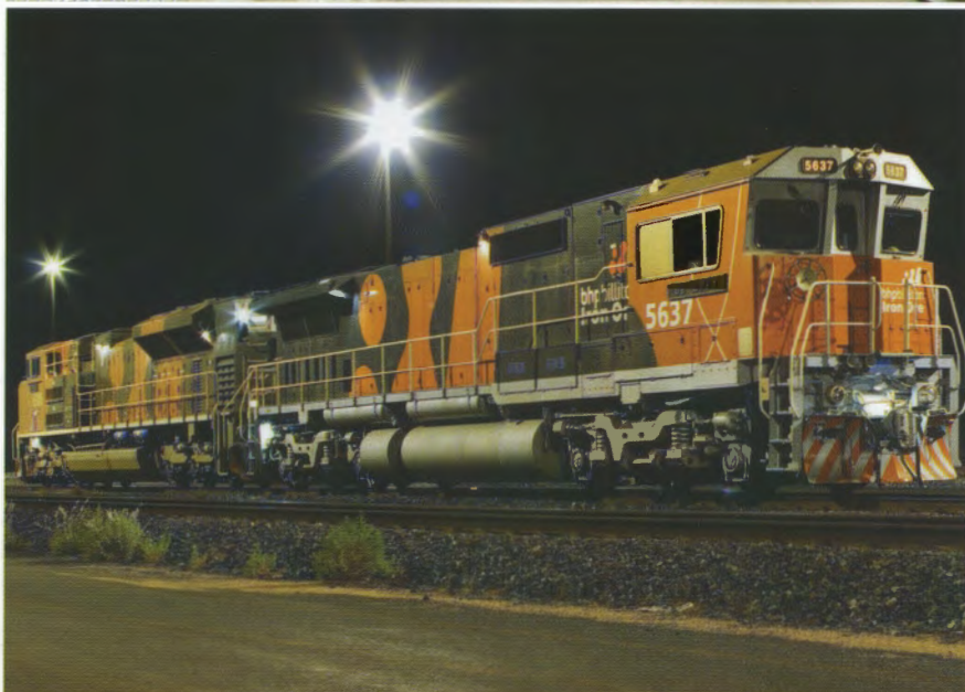
Top: Leighton Kumagai's 900mm gauge Schöma 4wDH 2 (5284 of 1992) at Esplanade Station, the entrance to Perth's Metro Rail Tunnel. Photo: courtesy Leighton Kumagai Joint Venture Above: Another superb night shot at Port Hedland shows BHP-Billiton's Co-Co DE locomotives 4305 COONARIE (Electro-Motive Canada 20038540-06 of 2005) and 5637 DE GREY (Goodwin G-6012-05 of 1968 rebuilt Goninan 123 of 1992) on 17 April 2006. Photo: Richard Montgomery
