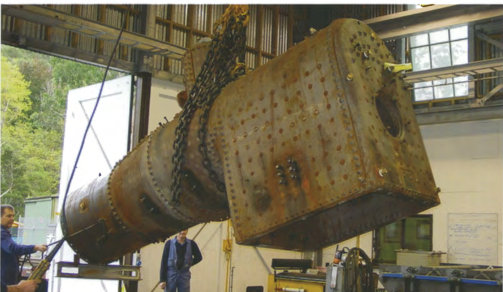
The boiler of Climax locomotive 1694 returned to Puffing Billy's Belgrave workshops on 24 April 2006 after reconditioning in the USA. Photo: Tony Johnson
