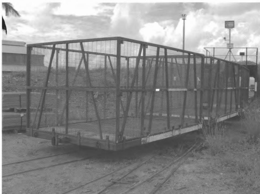
The first in the production line of ex-Moreton Mill bin conversions were turned out during March by Mackay Sugar's Marian Mill. Clearly visible is the added section to increase capacity from 5 to 6 tonnes. Photo: Reg Treloar
