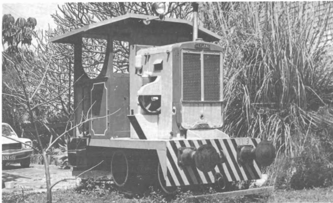
Alwyn Zinn built this four-wheel petrol locomotive in his back yard in the Ipswich suburb of Leichhardt in 1974. It was his third locomotive and was intended to be run on a tramway he hoped to construct. Unfortunately, his early death prevented him from carrying fulfilling this ambition. It is now part of the Australian Narrow Gauge Railway Museum Society collection and is pictured here in store in Brisbane in 1982.
