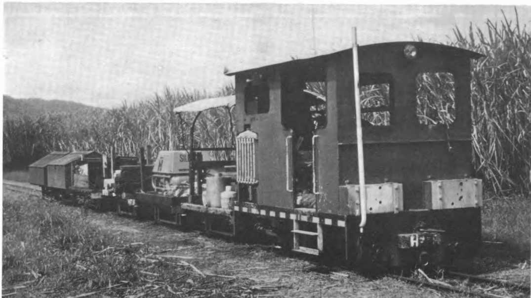
The Mulgrave Central Sugar Co. Ltd. constructed this locomotive in their own workshops in 1956. Equipped with a Southern Cross diesel engine, this four-wheel diesel-mechanical was designed to be able to haul cane over flooded track. It is now used to haul the navvies' train and was photographed on this duty near Fishery Falls in 1980.
