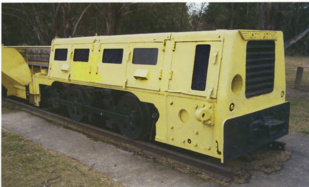
This rare North British 100hp 'Miner' type 0-4-0DH locomotive (B/N 27297 of 1952) formerly used at the Lithgow Valley Colliery is on static display at the Wallerawang-Portland Rotary Picnic Area. Photo: John Browning
