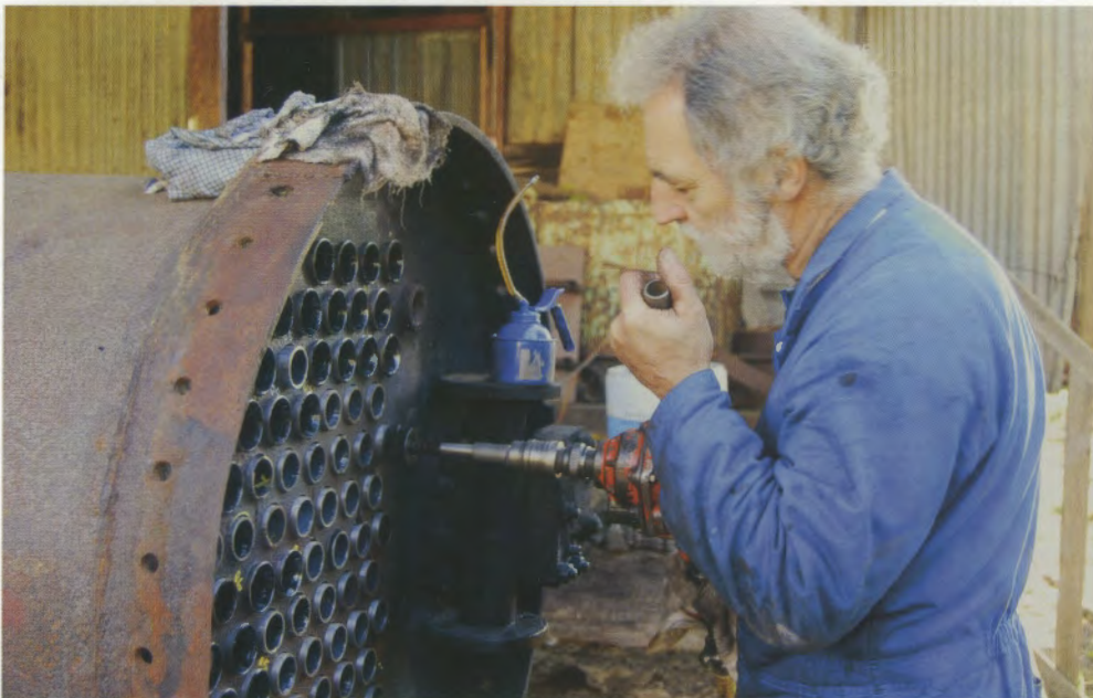
A consummate craftsman at work: Ernst, the ER Steam Engineering boiler-maker beading the tubes of the John Fowler boiler at Alexandra on 25 May with his special air-driven beading tool. Photo: Peter Evans
