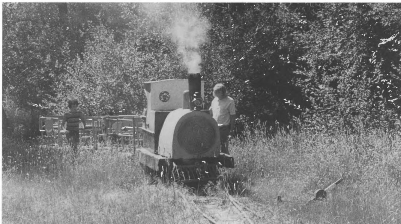
With the old jeep engine doing its best to imitate a steam locomotive, the WM MELDRUM has come to a stop near the eastern loop on Easter Saturday 1972.
