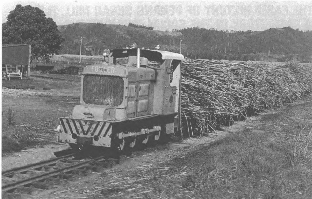
On 10th October 1968, Fowler 0-6-0DM 20827 of 1935 hauls a load of whole-stick cane towards Condong Mill. Unlike the majority of its Queensland colleagues, Condong did not upgrade its tramway network to cope with the transition to machine-cut cane, opting instead for a switch to road transport using the 'Canetainer' system. The last cane trams ran in 1974. Photo: R F McKillop
