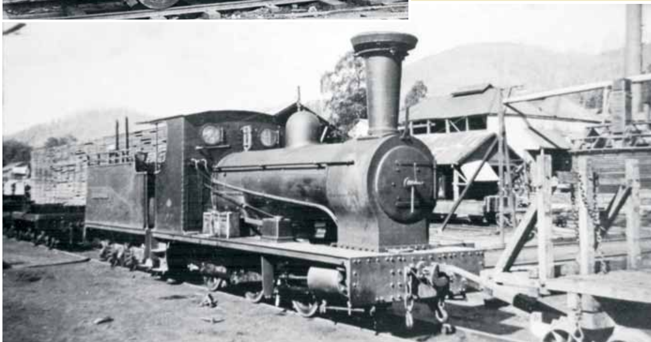
Baldwin 3ft gauge 2-4-0 LITTLE YARRA (B/No. 37718 of 1912) at Powelltown, c. 1937. The back of the tender has been dented as a result of a shunting accident, and the rails on the top of the tender have become very battered. Photo: JCM Rolland □ Kerr Stuart 3ft gauge 0-4-0T locomotive Coffee Pot (B/No. 643 of 1898) at Powelltown c.1937. The loco was painted green and traces of lining on the tank sides appear to be visible. Photo: JL Buckland □ Bagnall 3ft gauge 0-6-0 POWELLITE (B/No. 1965 of 1913) at Powelltown c.1937. The oversized funnel was fitted in the late 1930s by the Victorian Railways when the loco was overhauled at Newport Workshops, and in this view the pancake shaped object on top appears to be a Cheney spark nullifier. Photo: JCM Rolland
