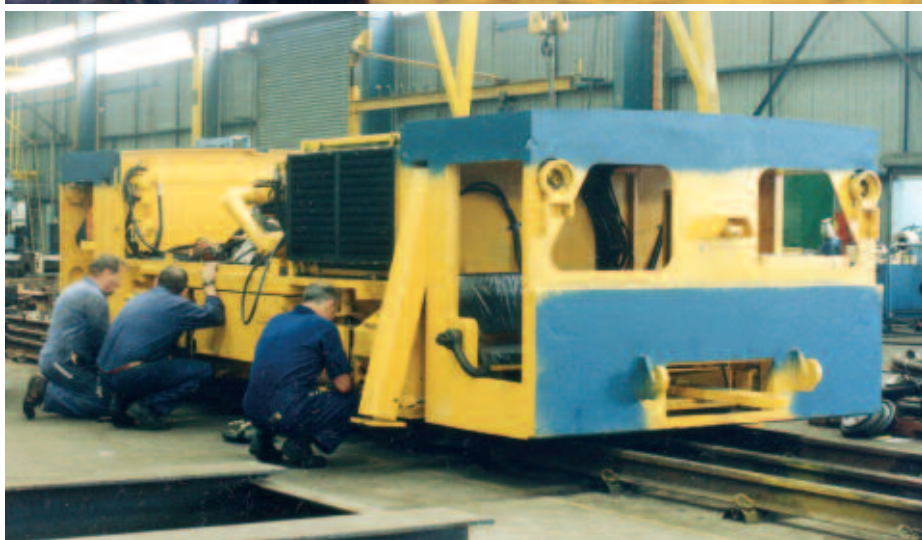
Above: South Bulli Colliery Fox man car 5A nearing the completion of repairs in the assembly area at Rooty Hill on 20 August 1991. Left: Working on Ellalong number 1 in January 1992. The lifting legs, which were a feature of these rack locomotives, can be seen partially extended. They could be used to rerail locomotives derailed underground and also to raise the locomotive in the surface colliery workshops to facilitate access. Below: Ellalong number 2 rigged up to a final drive gearbox test rig on 11 February 1992. The locomotive was delivered two months later. Photos: Craig Wilson
