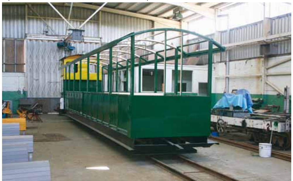
Former Mulgrave Mill 'Rambler' passenger vehicle No 3 under restoration in Melbourne. Com-Eng 4wDH (GA1148 of 1961) formerly Fairymead Mill No 72 is in background also under restoration, awaiting the installation of a replacement Perkins R6 diesel engine.
