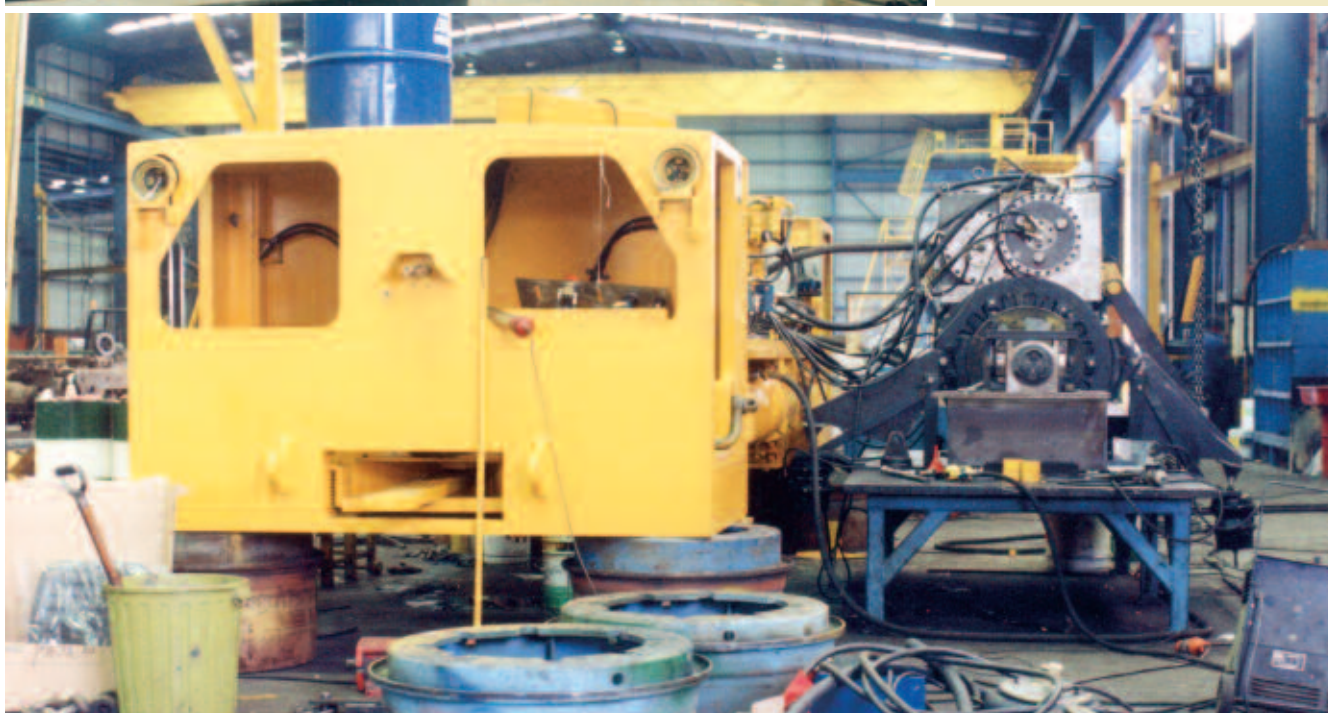
Above: South Bulli Colliery Fox man car 5A nearing the completion of repairs in the assembly area at Rooty Hill on 20 August 1991. Left: Working on Ellalong number 1 in January 1992. The lifting legs, which were a feature of these rack locomotives, can be seen partially extended. They could be used to rerail locomotives derailed underground and also to raise the locomotive in the surface colliery workshops to facilitate access. Below: Ellalong number 2 rigged up to a final drive gearbox test rig on 11 February 1992. The locomotive was delivered two months later. Photos: Craig Wilson
