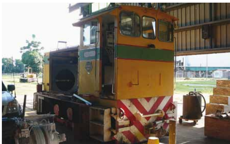
In the Macknade Mill loco shed, EM Baldwin 0-6-ODH HOBART (4413.1 7.72 of 1972) awaits the fitting of its new Mercedes-Benz engine on 15 February 2010.
