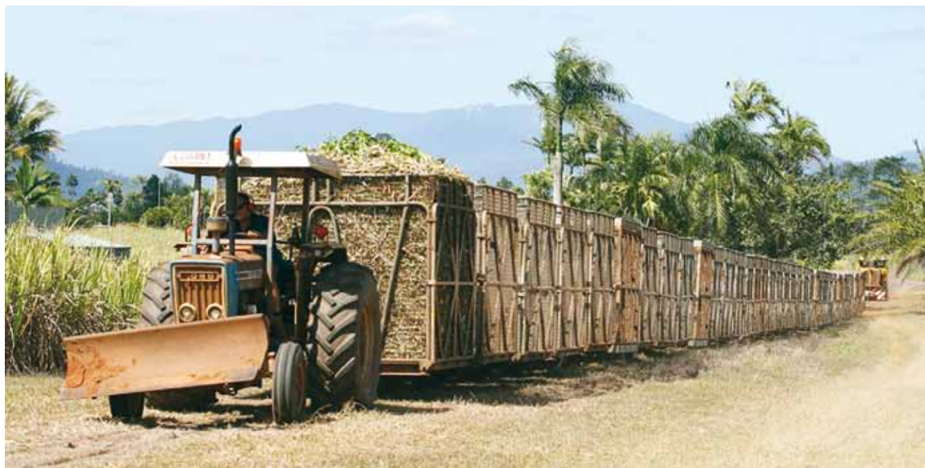
On 20 September 2009, South Johnstone Mill's Com-Eng 0-6-ODH 38 (AH4695 of 1965) was pushing 40 empty bins up the Little Tableland line when some became derailed because of dirt over the rails at a banana shed. The offer of the farmer to pull the bins up with his tractor was accepted and here it heads up the rake with one full bin in the lead while the locomotive crew look on from the rear.
