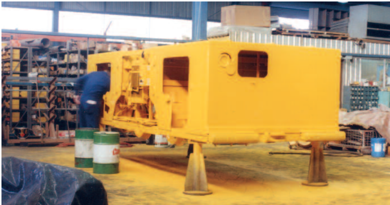
Above: South Bulli Colliery Fox man car 5A nearing the completion of repairs in the assembly area at Rooty Hill on 20 August 1991. Left: Working on Ellalong number 1 in January 1992. The lifting legs, which were a feature of these rack locomotives, can be seen partially extended. They could be used to rerail locomotives derailed underground and also to raise the locomotive in the surface colliery workshops to facilitate access. Below: Ellalong number 2 rigged up to a final drive gearbox test rig on 11 February 1992. The locomotive was delivered two months later. Photos: Craig Wilson
