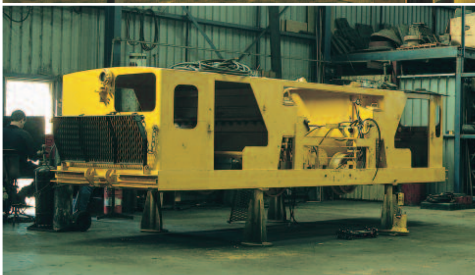
Above: AI&S Cordeaux Colliery man car AIS 139. Built by Vernier, the man car came to Rooty Hill for accident repair and overhaul. With repairs completed the man car awaits return to the colliery on 17 April 1991. Left: South Bulli Colliery SBC 23 (13800.2 5.91) under construction at Rooty Hill on 17 April 1991. Below: Ellalong number 2 (14526.1 3.92) was returned to Rooty Hill in October 1992 for warranty repairs on the gearboxes and is pictured here on 9 October 1992 at the works. Photos: Craig Wilson
