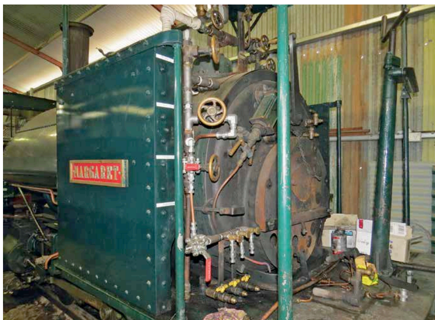
Cobdogla, Bagnall locomotive: the Christmas tree from top, isolating valve, blower, injector and tender steam heat. The two off three valve branches are top row, oil burner steam supply, bottom row, oil supply. Photo: Denis Wasley
