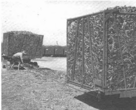
Above A typical rail-backed truck operation where tramway bins are winched onto the back of a truck or trailer which has been fitted with rails. The wagons are then taken to be loaded with cane. Heck's Rocky Point Mill, 1974.
