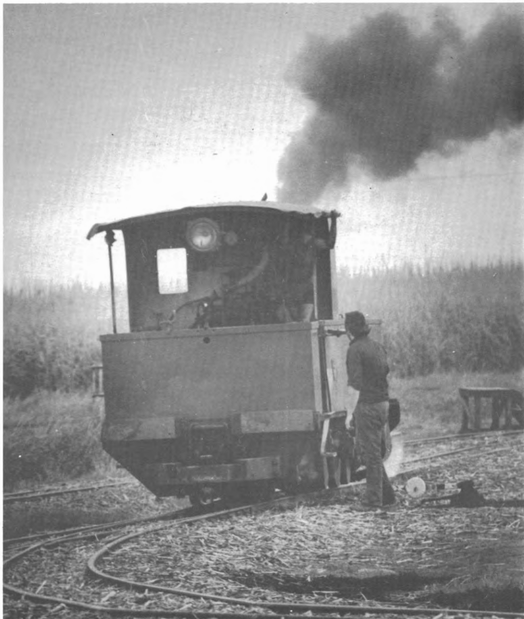
One of the last surviving steam locomotives in the Australian canefields today; Marian Mill's 0-6-2T Perry (B/No.2601.51.1 of 1951) seen here shunting the yard on the southern side of the mill. 1977.
