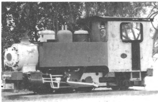
Above This Fowler locomotive, ex-No.8 of Pleystowe Mill, is a sorry sight at Bucasia Beach near Mackay in 1977. The loco (B/No. 20764 of 1937), is corroding and is missing various parts. It and several other 'preserved' locos have recently been taken away for scrap as local authorities find the task of properly caring for the deteriorating relics to be beyond their resources. Unless properly cared for, they quickly become a danger to the safety of the children who love to play on them.
