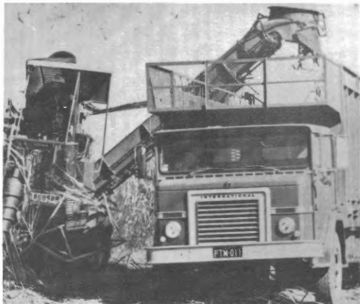
Above In some cases road vehicles are taken into the canefields and loaded direct for road transport to the mill or transfer points where their load of cane is tipped into tramway wagons.
