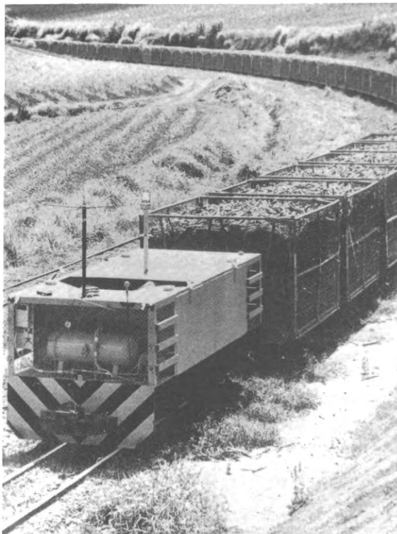
Above An early experimental model of the Clyde radio-controlled remote brakevan. Seen here undergoing trials in the early 1970s.
