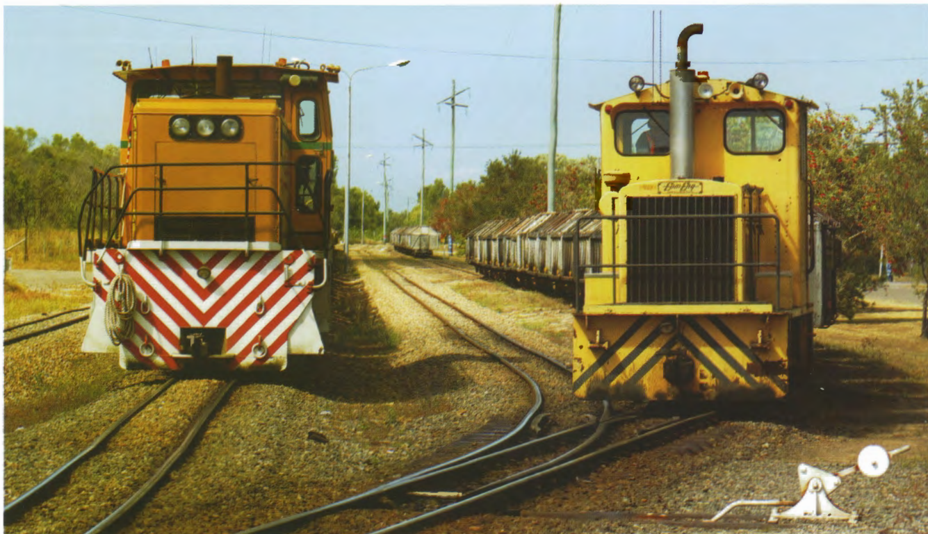
Dignity and impudence. Victoria Mill's Walkers B-B DH CAIRNS (681 of 1972 rebuilt Bundaberg Foundry 1997) waits while the Queensland Sugar Industry Corporation's Com-Eng 0-6-0DH G1023 of 1958 shunts sugar boxes at Lucinda Bulk Sugar Terminal, 27 August 2006.
