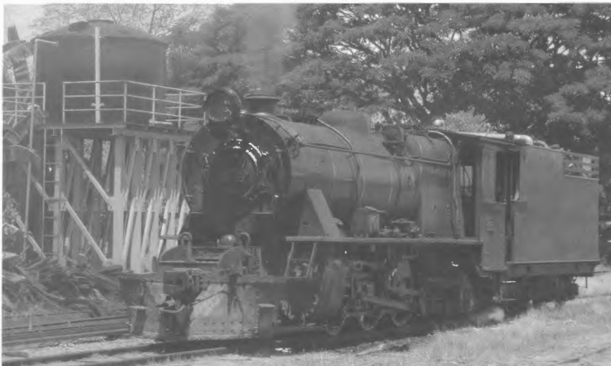
Engine 6-016 (Vulcan 6276 of 1955) takes water after being turned at Papar ready for the return run to Tanjung Aru on 17 June 2006. Photo: Kevin Waid
