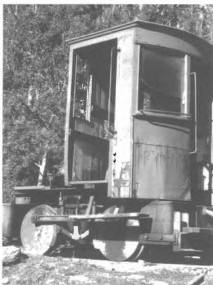
The 0-4-0DM Days loco frame with cab from ex-Hobart Municipal 'Tramways' sprinkler car at Cornwall Colliery, November 1966.
