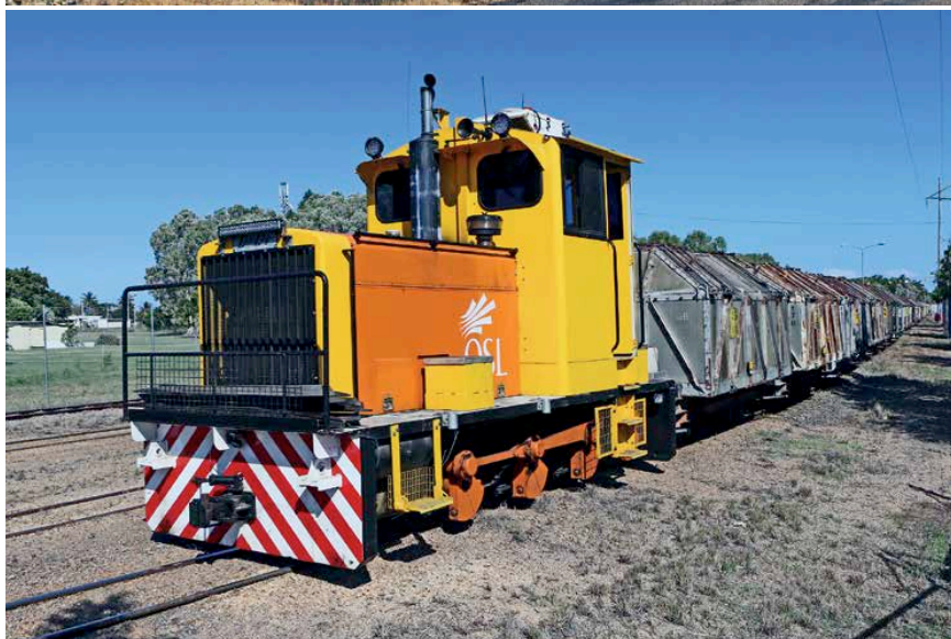
Top: Walkers B-B DH 4 (656 of 1970 rebuilt Walkers 1994) has just retrieved its Hexham Engineering bogie brake wagon 4 (HE 684 of 1987) from the end of a rake of bins in the Isis Mill full yard on 14 July. Photo: Brian Bouchardt Centre: Farleigh Mill's EM Baldwin B-B DH Inverness (10123.1 5.82 of 1982) on the Palmyra branch with twenty-three full 6 tonne bins from Palmyra 6 siding on 29 June. Photo: Steven Jesser Above: Sugar Terminals Ltd Com-Eng 0-6-0DH (G1023 of 1958) shunting at the Lucinda Bulk Sugar Terminal on 29 July. Photo: Luke Horniblow
