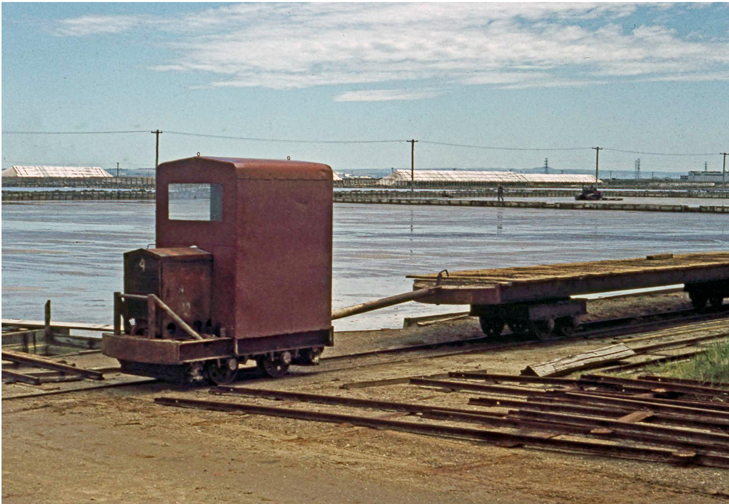
Below: Cheetham light loco No.4 with a bogie flat truck at Moolap on 2 November 1965. Note the method of making a temporary crossing of two tracks by simply removing a section of rail. Photo: Ray Graf
