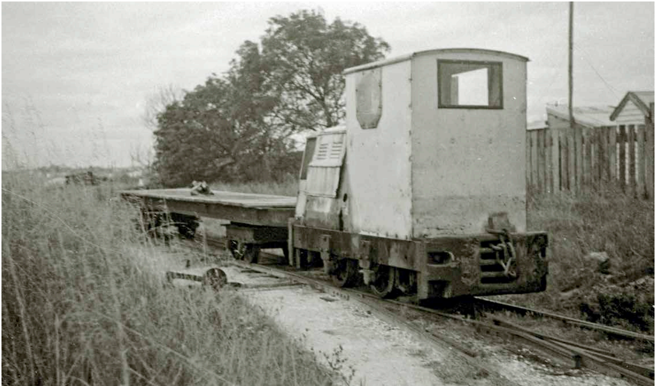
Above: A bogie flat-truck of the type used for construction work around the salt pans and for transporting bagged salt to Cheetham's siding on the Geelong-Queenscliff railway. The locomotive is one of the Ruston 30DLUs. Photographed on 1 March 1969 by Phil Rickard
