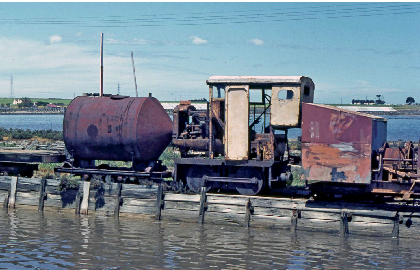
Above: 'Rotten Row' at Moolap on 2 November 1965 with, from left, a bogie flat-truck, an improvised loco fuel wagon, a derelict Day's loco, and a powered winch for placing the conveyor system on the crystallisers for harvesting. Photo: Ray Graf
