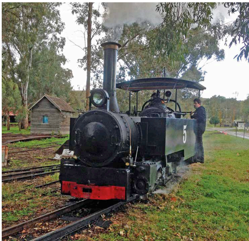
John Fowler 0-6-0T 11885 of 1909 undergoes a steam test at Alexandra on 11 August following the successful completion of its annual boiler inspection.
