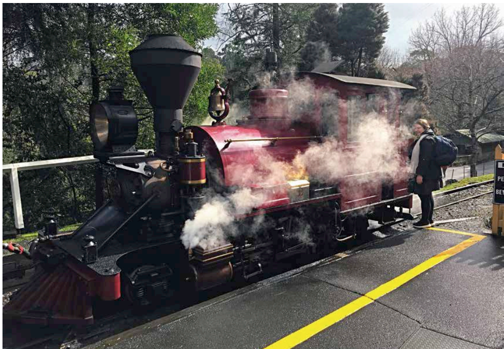
Former West Melbourne Gasworks 0-4-0T JOHN BENN (Couillet 861 of 1886), rebuilt as a 2-4-2ST and renamed JC REES, at work on a Footplate Experience Train at Lakeside on Sunday 19 August 2018. Photo: Mike McCarthy
