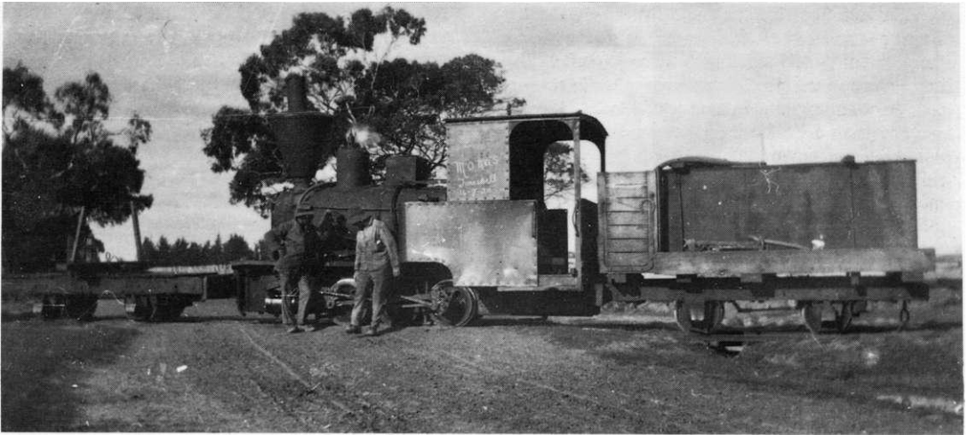
The rebuilt Mona on its last trip on 14 July 1920 at the head of a dismantling train. The locomotive shows a distinct change in its appearance following its reconstruction with a somewhat makeshift cab replacing the elegant original Krauss construction, and a home-built spark arrester replacing the original funnel. Note the horseshoe attached to the tender as a reminder of its calamitous past.
