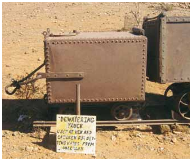
The ex-Hen & Chicken dewatering truck on display at the Daydream Mine at Silverton. Photo: Alf Atkin
