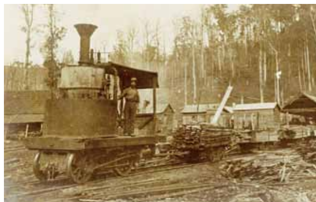
Ex-Victorian Railways Rowan car engine unit (Kitson B/No. T69 or T70 of 1883) regauged to 3ft 6in at Sanderson's Barwon Mill c. 1908. These locomotives performed well, and were popular with the crews.
