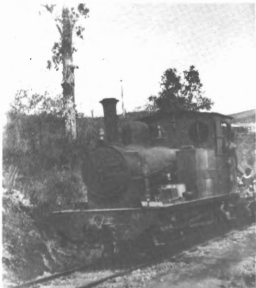
Polygon, Andrew Barclay's 0-6-0T locomotive (B/N15144 of 1918) at work on the Bootless Bay railway.
