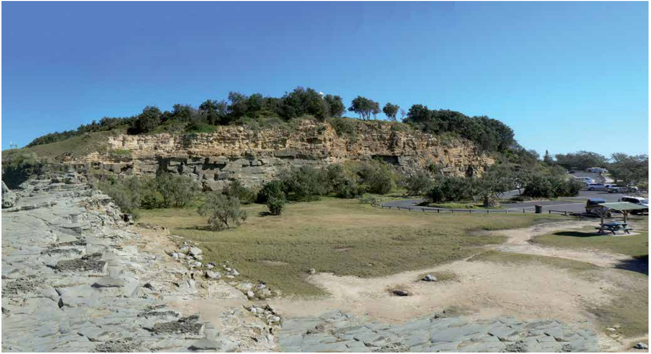
Panoramic view of the quarry face of South Head Quarry 2015. The dark-coloured lower layers of rock were the hard blue sandstone used for breakwater construction. The lighter coloured upper layers were softer rock which had to be run to spoil. Photo: Ian McNeil
