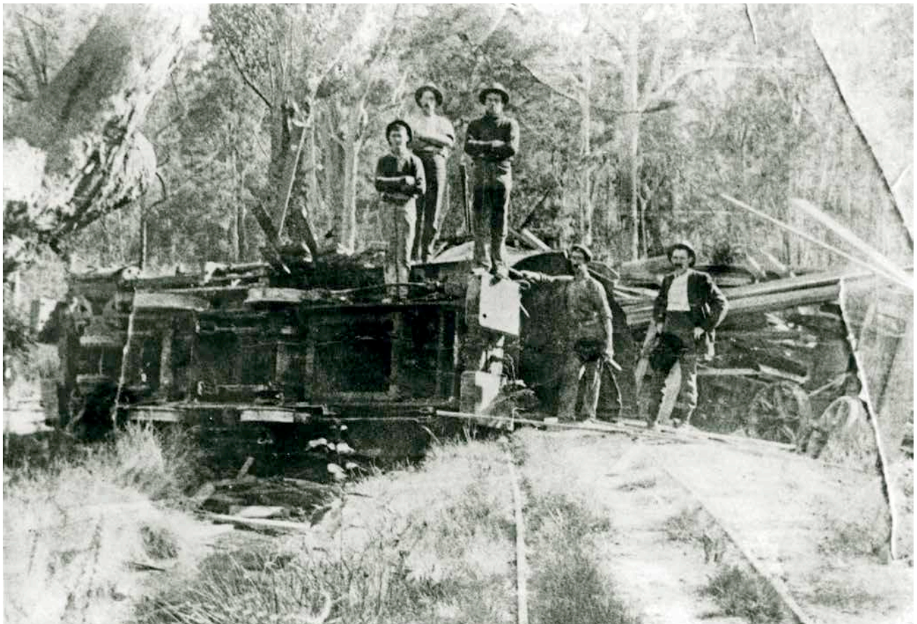
This is believed to be the result of the July 1915 runaway involving 0-4-0ST Andrew Barclay 237/1881 on the Boambee Tramway. The crew were able to jump clear but the locomotive suffered damage variously reported as either 'not serious' or 'severe,' depending on which newspaper is to be believed. The locomotive later inherited the boiler and cab from 0-6-0ST Andrew Barclay 222/1880, and the damage sustained in this accident may have been one reason why.
