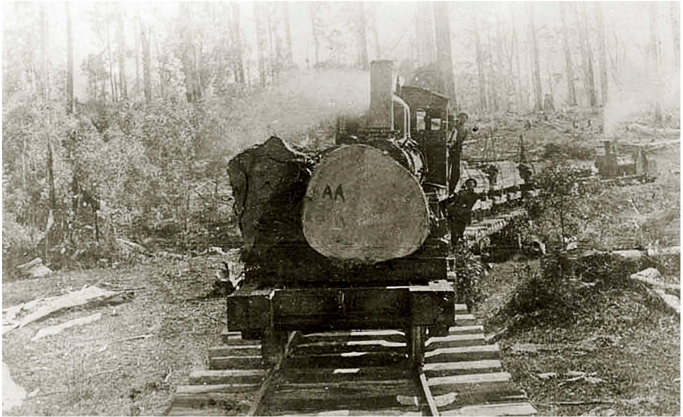
A-class Shay (Lima 2135/1909) propelling a loaded log truck and hauling a trainload of sawn timber with 0-4-0ST Andrew Barclay 237/1881 bringing up the rear on the Boambee Tramway c1915. The CHTCo. had plans, which never eventuated, for 17 miles of logging tramways in rugged country west of the Coast Range. The Shay was acquired with this aim in mind. Photo: Coffs Harbour Library
