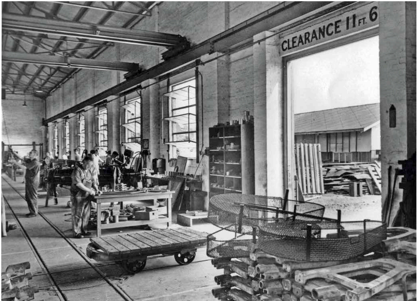
John Heine & Son. The 4-wheel flat top trolley looks rather like a V-skip frame on which has been laid the timber decking.
