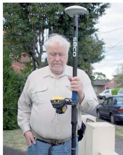
Iain Stuart demonstrating the set-up of a professional grade GPS – A Trimble Geo7X with an external aerial on a carbon fibre pole. This set up with real time correction would give an accuracy of 1cm horizontally and 2-3cm vertically in the open.
