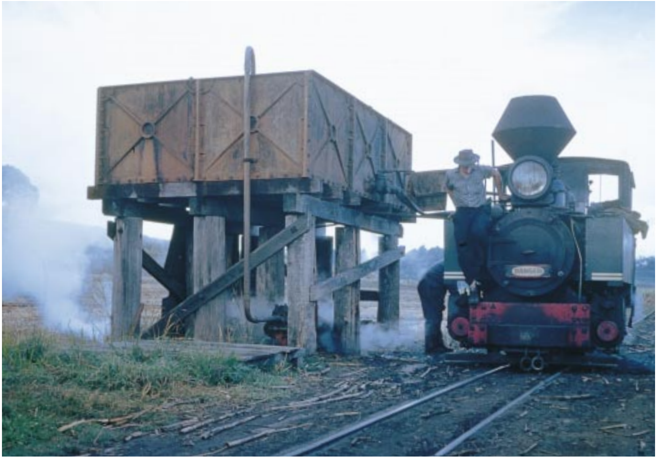
On 7 September, 1965, Robert spent much of the day riding on COOLUM (Fowler 16036/1923) and he recorded this scene as it stopped for water at Bli Bli Tank. As the loco takes water, its steam is being utilised to replenish the supply, by way of the horizontal steam pump mounted between the tank footings.
