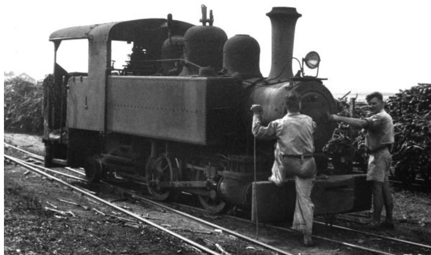
Driver George Fabris and his fireman prepare to clean out the smokebox of South Johnstone No.1 (Porter 5812/1916) which regularly operated the Warrakin Branch in the 1940s. By then, it had acquired a Hunslet chimney and a locally-cast smokebox door. Photo: Ken Rogers via George Bond
