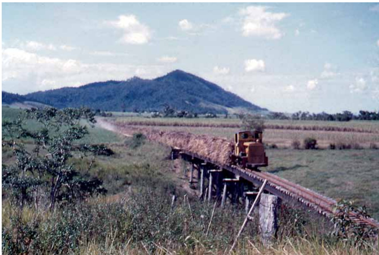
John Fowler 0-6-0DM 8 (21912 of 1937) was re-engined with a Caterpillar diesel in 1950 and was thereafter known as 'the Cat'. Here it has hauled its rake across Kelly's flat and is commencing its ascent of the range. Photo: Len Heaton
