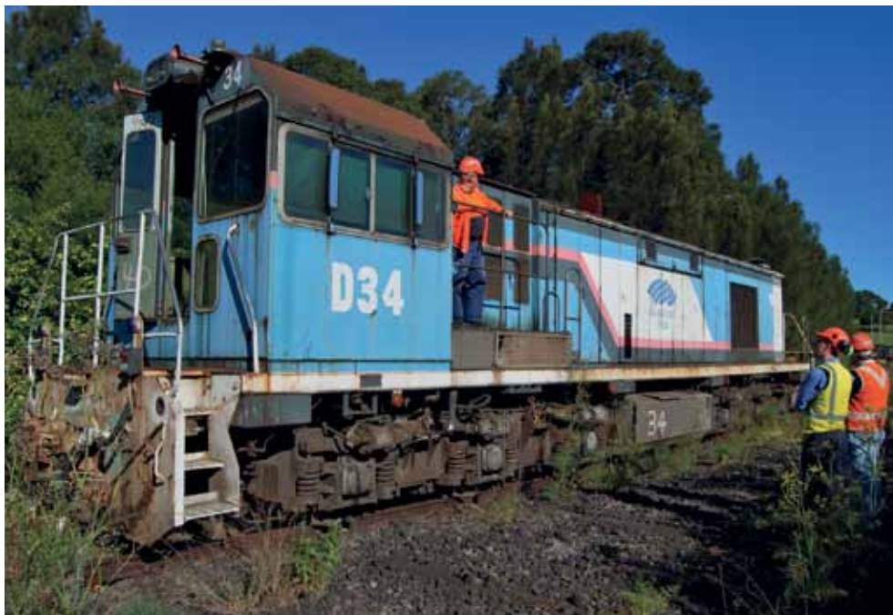
The former Bluescope Steel 1800hp locomotive (English Electric Aust. A.197 of 1969) in storage at Port Kembla was photographed by Michael Wilson when a group of State Mine Railway officials inspected it in September 2011.
