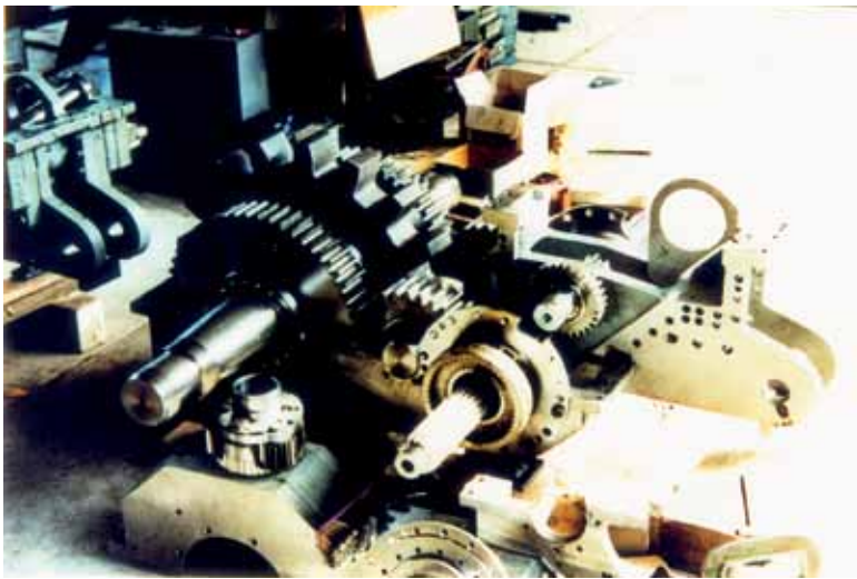
Above: Late in the afternoon of 13 February 1994 the first of the locomotives built by the partnership was tested. On hand (L-R) are Frank Baldwin, Brian Watts and Maurice Baldwin. Also present were Stewart Baldwin and the author. Photo: Craig Wilson Left: The final drive unit for the 12 ton locomotive partially assembled. The picture is taken from the rack side with the rack drive bull gear closest on the rear axle. The adjacent shaft carries idler gears. Next to it are rack side idler gears and on the far side the traction idler gear. The final visible shaft formed part of the Clark clutch pack assembly. Not visible due to its being located in the top cover assembly is the shaft and gearing powered by the Rexroth hydraulic motor. Photo: FE Baldwin Below: The rack locomotive under construction in February 1995. Photo: Craig Wilson
