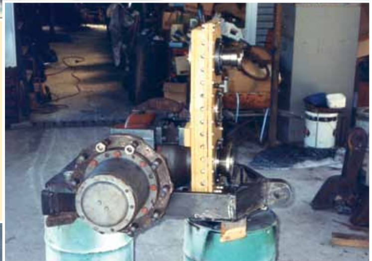
Above: The first set of brake wagon bogies for Invicta Mill at Kings Park in 1993. The disc brakes can be clearly seen. Photo: FE Baldwin
