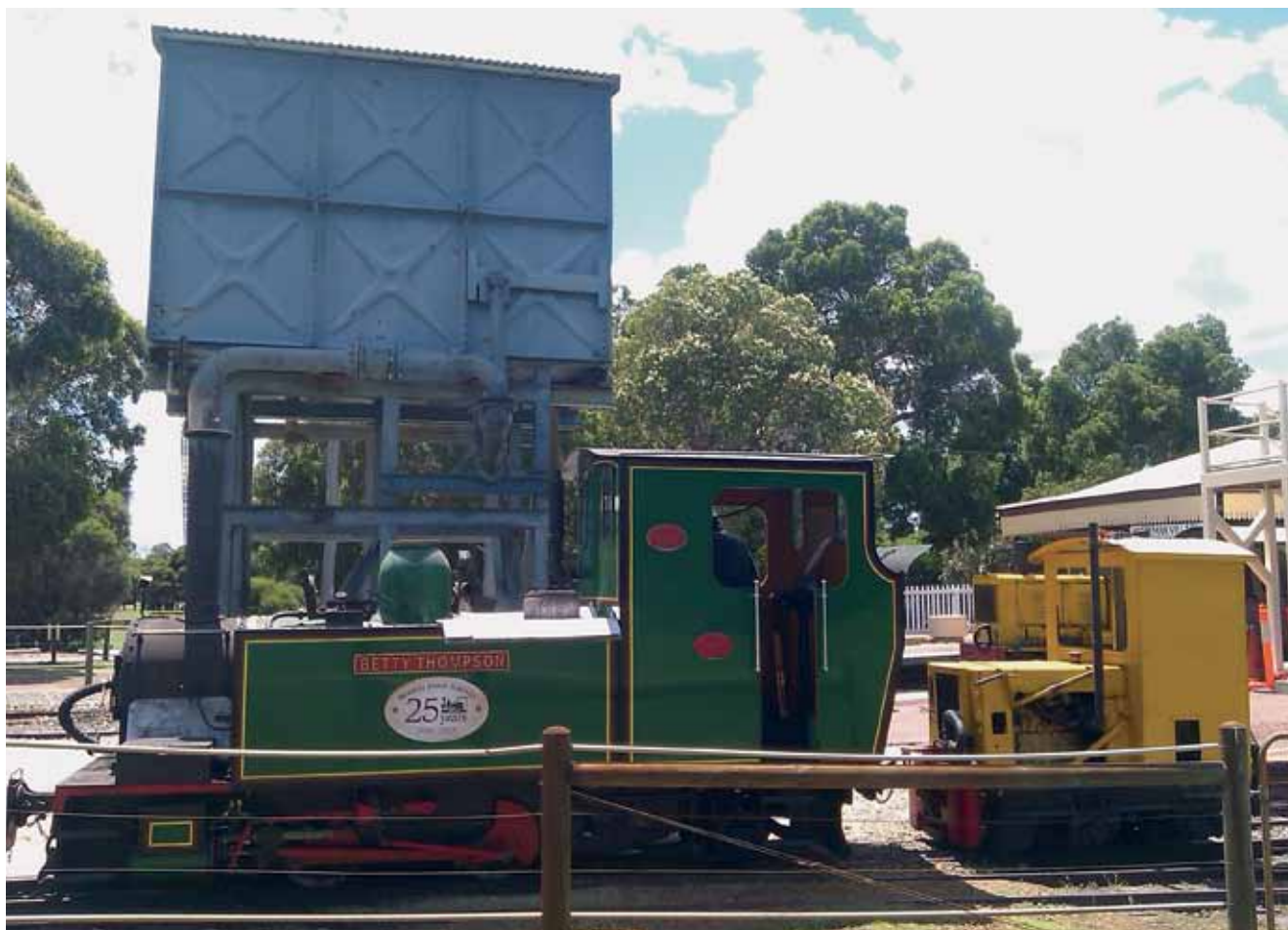
The Bennett Brook Railway's former Bunning Brothers 4wDM RUSTON (Ruston & Hornsby 1957) assisted in moving 0-4-2T BETTY THOMPSON (Perry Eng 8967.39.1 of 1939) to the new water tank at Whiteman Village Junction station on 21 January 2012 to test how long it took to fill the side tank. Photo: James Waterhouse
