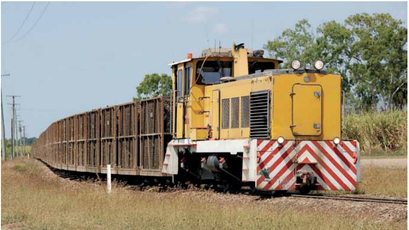
Invicta Mill's Westfalia B-B DH STRATHALBYN hauls a loaded train to the mill on 28 September 2006. A set of bogies came with this locomotive for Invicta to build a brake wagon. Its success inspired further orders, which the Baldwin brothers were happy to fill. Photo: Matt Green
