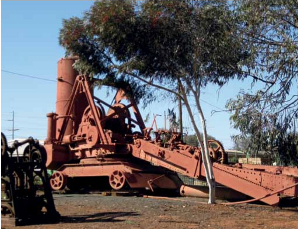
This unusual vertical-boilered, rail-mounted machine was photographed at Boulder railway station on 24 August 2011. Unfortunately there was no interpretative signage provided, but it is understood that this is a steam navy built by Whittaker Brothers. Can any reader provide details of its origins and purpose? Photo: Bob McKillop
