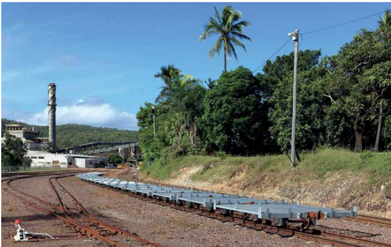
On 4 March 2012, new bin chassis, delivered to the Plane Creek Mill yard, await the fitting of sides and ends in the mill truck shop to be ready for service in the 2012 season. Photo: Carl Millington
