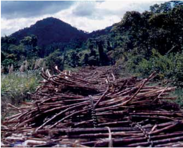
Heading up the range, the driver continually looks back to check that the rake is intact. The taut chains hold down the cane and stop it slipping sideways off the trucks. Photo: Len Heaton
