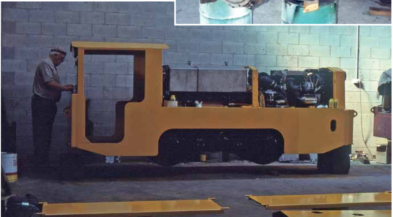
Below: Frank Baldwin working on DL 1 on 13 February 1994. The larger of the two tanks in front of the cab is for water for the scrubber while the smaller is the fuel tank. Photo: Craig Wilson
