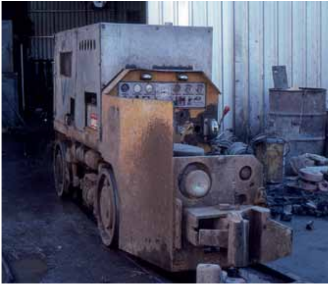
DL 3 at Lawson after installation of a new Deutz engine.
