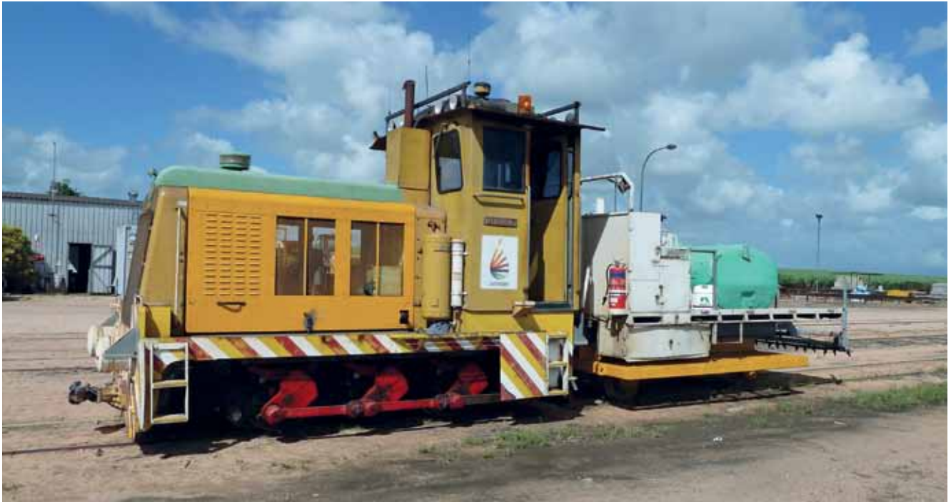
Above: Another weed spray unit, as used on the 1067mm gauge Pioneer Mill system, with Clyde 0-6-0DH MAIDVALE (63-266 of 1962) on 1 March 2012. Photo: Luke Horniblow Left: Clyde 0-6-0DH 19 REDLYNCH (65-435 of 1965) with Mulgrave Mill's weed spray unit at Redlynch depot on 3 March 2012. With its low-profile cab it is able to pass under the QR and travel to the extremities of the rail system in the Barron delta. Below: The appearance of Pioneer Mill's 5803 (Walkers B-B DH 682 of 1972) has changed little since it left the Mt Isa Mine in 2007. Here it shunts QR molasses tankers at the mill on 1 March 2012. Photo: Luke Horniblow
