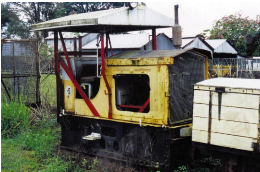
Mourilyan Mill's unidentified 610mm gauge Malcolm Moore 4wDM •5 at Goondi Mill site during 1998, shortly before its acquisition by Andrew Forbes. The original Malcolm Moore cab supports have had some additional side bracing added by the mill.
