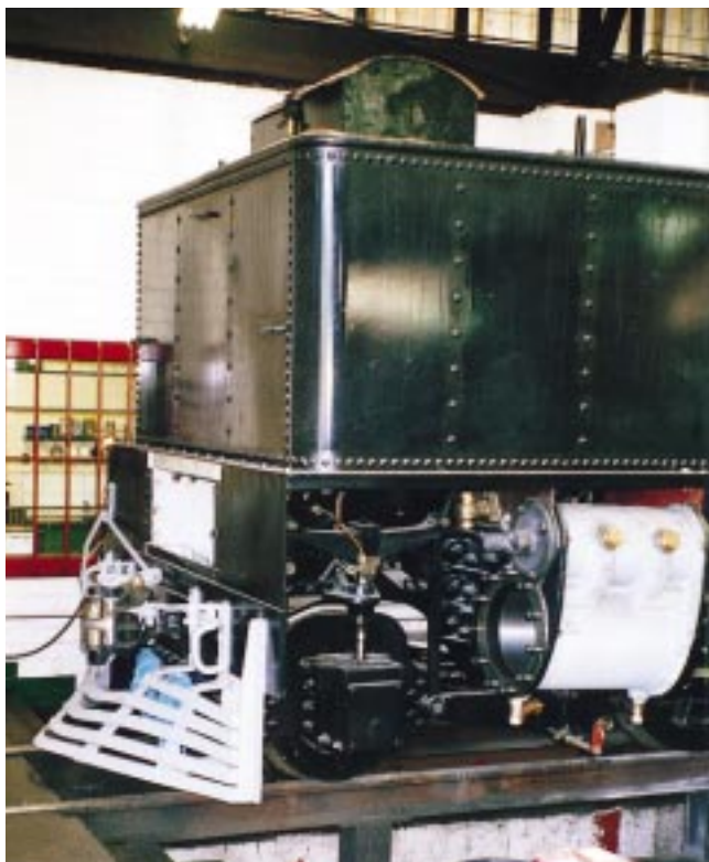
The front unit of Garratt G42 in Belgrave workshops, 12 December 1998, with the water tank now permanently attached. Photo: Peter Medlin
