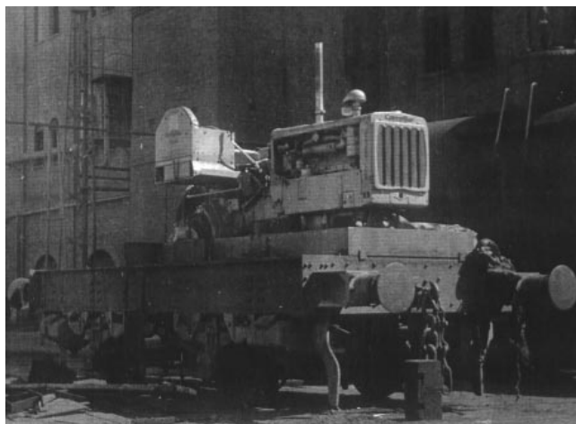
The former Sentinel loco as rebuilt by the Company in 1947. At this stage, there was no protection for the driver - in wet weather, he had to wear a raincoat!
