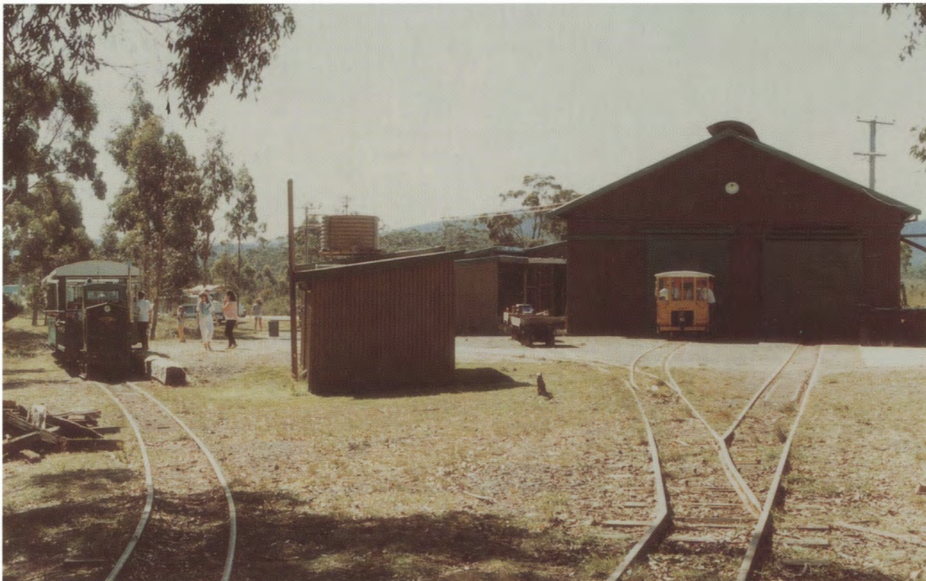
A view of the depot at Ida Bay, 30 March 1986, seen from the quarry side. Number 1 is in the platform on a 3-car train. During school holidays, trains of up to 4-cars loaded with over 90 passengers were not uncommon. The single-bladed points look very primitive, but did not cause any problems, provided they were tackled at low speed.
