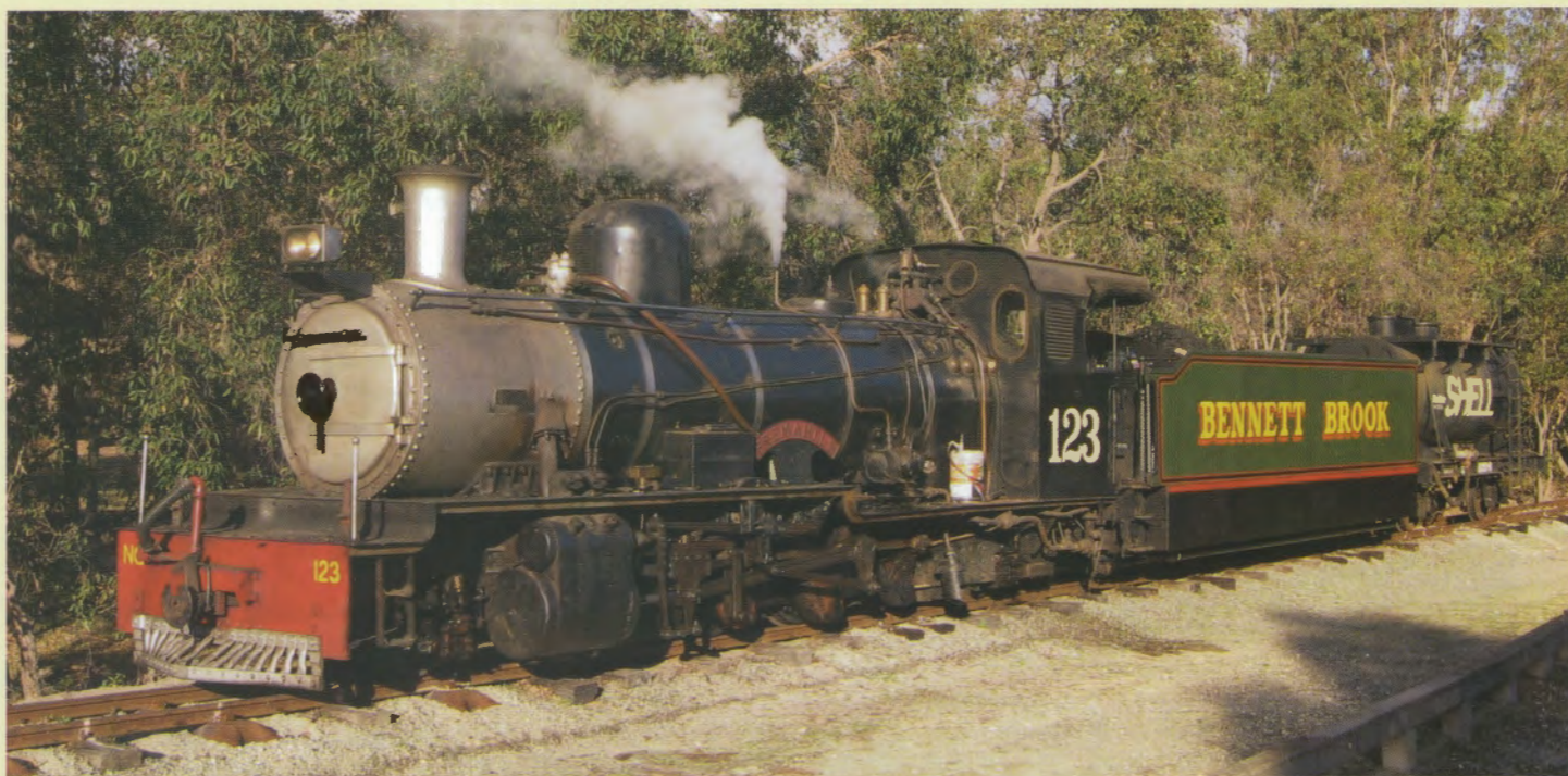
An important event on the Bennett Brook Railway as 2-8-2 NG 123 (Anglo-Franco-Belge 2670 of 1950) arrives in 2 Road at Whiteman Village Junction station under its own steam for the first time in 12 years during a test run on 12 May 2007. The locomotive is attached to the tender from NG 118 (Henschel 24476 of 1938) Photo: Neil Blinco □ Newly painted for the start of the season, Plane Creek Mill's Com-Eng 0-6-0DH 4 (FA1037 of 1960) heads north at Koumala on 29 June 2007 with an empty ballast train from Tinerta bound for Shannon's Flat depot. Photo: Carl Millington □ Following a mishap in 2006, Mackay Sugar's Walkers B-B DH BALBERRA (Walkers 657 of 1970 rebuilt Tulk Goninan 1994) has been repaired and repainted in the new yellow livery. It commenced the 2007 season working out of Pleystowe Mill and is seen here on 9 July 2007 crossing Sandy Creek on the old North Eton Main Line 2. Photo Carl Millington
