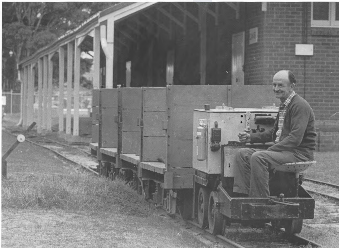
An empty explosives train of SAR-designed flat cars departing the Unloading Sheds, August 1972. Driver Bert Halfpenny is at the controls of the Wingrove & Rogers BEV locomotive type W.217 minus its coupling rods. Photo: F Brian Andrews
