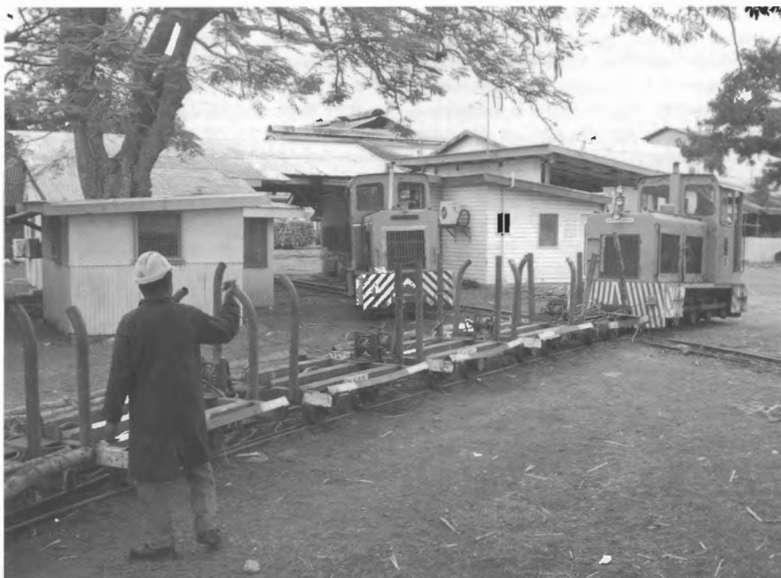
Fiji Sugar Corporation, Penang Mill. Baguley-Drewry 0-6-0DH 9 (3772 of 1983) pushes empty cane trucks over the diamond crossing and towards the empty yard as Baguley-Drewry 0-6-0DH 18 (3770 of 1983) looks on from the weighbridge line, 4 October 2006.
