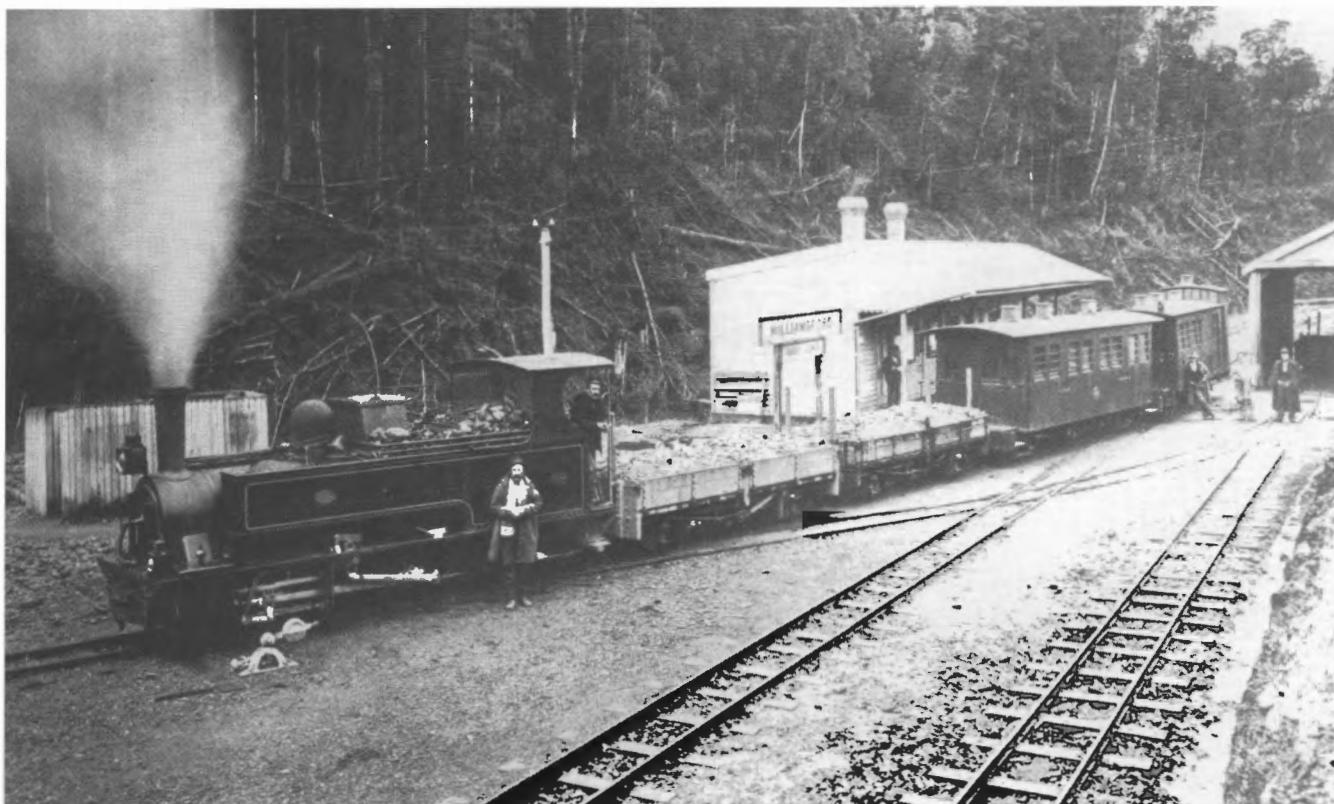
One of the G-class 0-4-2T locomotives (Sharp Stewart 4432 of 1898 or 4619 of 1900) about to leave Williamsford with a mixed train consisting of two loaded A-class ore trucks, an AB composite carriage and 1st/brake composite car AD1. Photo: National Archives, Hobart Office
