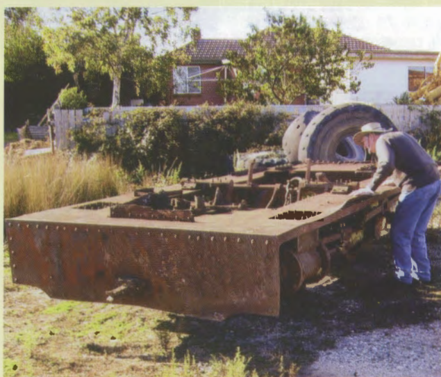
The frame of the former Beaconsfield Tramway 0-4-OT (Kerr Stuart 685/1900) in the yard of a local sand and gravel merchant at Beaconsfield, where it is intended to restore the remains to display condition. Photo: Ken Milbourne
