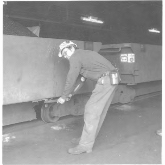
Pulling the doors of mine cars using "U" shaped tool. Photo: Brian Andrews
