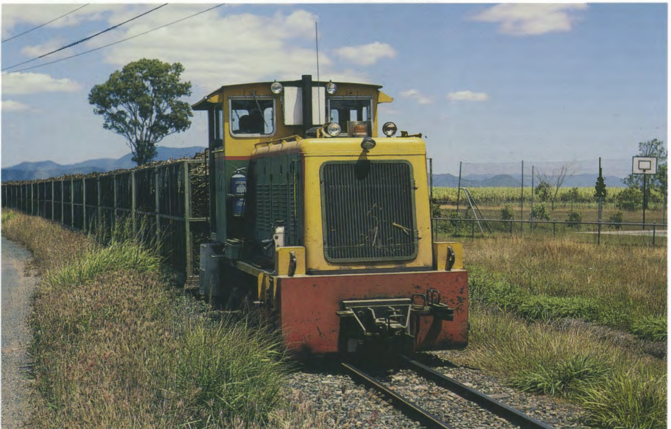
MELBA brings in a load of cane to Marian Mill on 1 October 1995. The Baldwin replacement cab was different in design to those made at Castle Hill with the air conditioning fan located on the front of the cab rather than for all earlier Clyde replacement cabs at the rear. Photo: Craig Wilson
