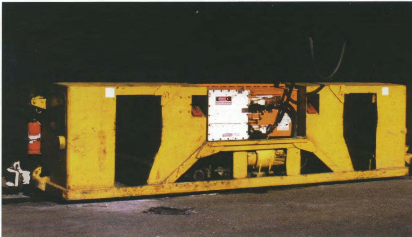
PC 11 (EMB serial 9981.1 10.82) stands under charge at Cooranbong Colliery pit top on 18 June 2000, fifteen years after its only visit to Rooty Hill. Since that time it has had its frame and body strengthened with additional welded supports in the battery bay, and strengthening steel also welded at the top of the doors. It will be noted that the cars also retain their Hexham heavy-duty haulage couplers. One wonders what stresses the cars were still undergoing especially as the sister cars at Myuna were not all converted in the same manner. Photo: Ray Graf, Craig Wilson Collection
