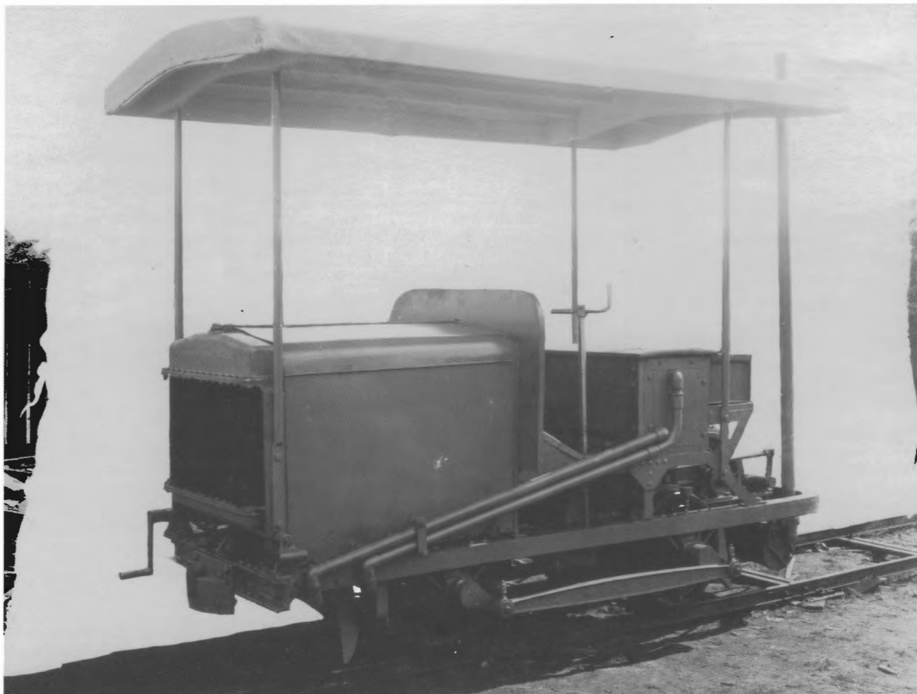
Retouched builder's photograph of the completed locomotive at Caldwell Vale's Auburn works. The starting crank handle, fabricated frame, tall and dainty canopy supported on four spindly columns, the skinny brake handle, exposed pipes, and extremely long exhaust pipe gave the locomotive a somewhat Emmett-like appearance
