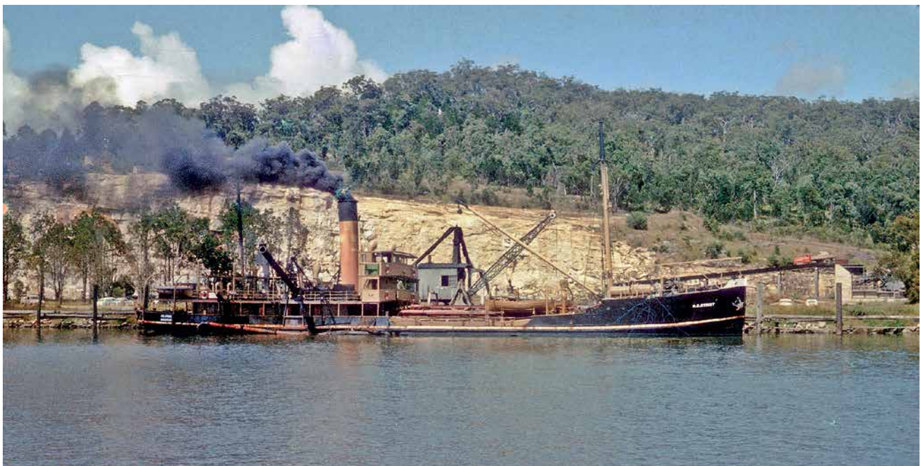
The modern twin-screw suction dredge, H.E. Street, built in 1949 at Newcastle State Dockyard for service on North Coast rivers, at work in the river channel fronting Ilarwill Quarry. The quarry's 10-ton steam crane is visible behind the dredge, while the vehicle ramp and jaw crusher – part of the concrete block plant – can be seen to the right of the ship's bow.
