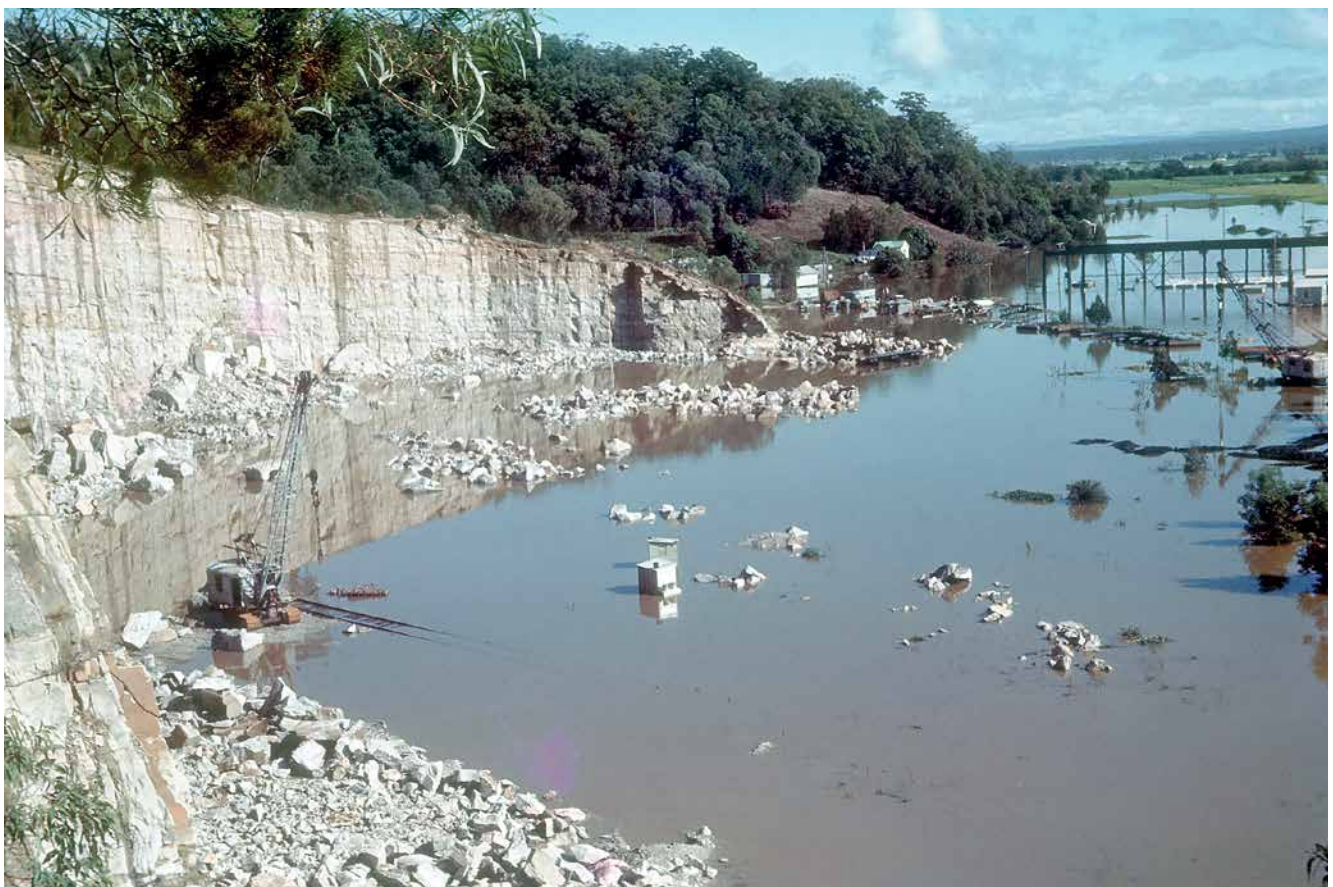
Below: Ilarwill Quarry here seen underwater during major flooding on the Clarence River in May 1963. Sections of the quarry face were over 140ft high and required specialised deep-drilling equipment to bore full-length holes for explosive charges. One of the big diesel caterpillar cranes employed to load stone onto rail trucks is dwarfed by the rock wall behind it. Photo: Norman Brown collection
