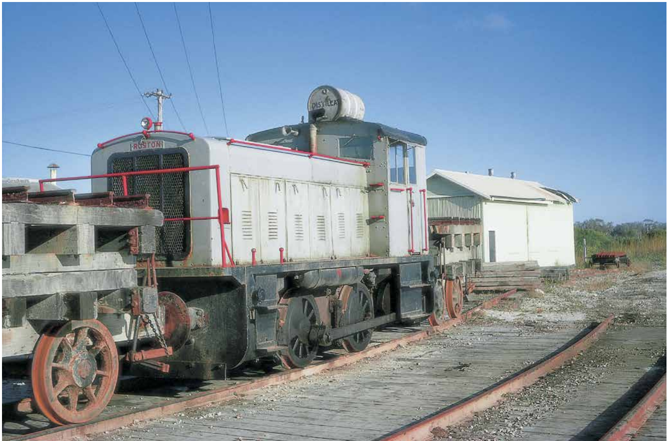
A 28-ton standard-gauge Ruston & Hornsby diesel locomotive at Yamba Crane Wharf circa 1970. It was one of two locomotives, Nos 310085 and 313393, imported new from England by the PWD in 1952 for the breakwater project. One was employed at Clarence Heads, the other at Ilarwill Quarry.
