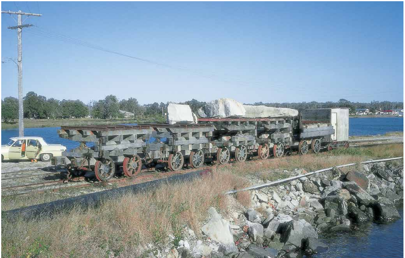
Above: A short rake of side-tipping and end-tipping standard-gauge stone wagons stabled on the South Training Wall at Yamba, near the 40-ton gantry crane. They were built in the Ilarwill Quarry workshops and subsequently strengthened to carry 40-ton concrete blocks. The NSW PWD used these ubiquitous four-wheelers on breakwater and harbour construction works for over 50 years. Photo: Ron Preston
