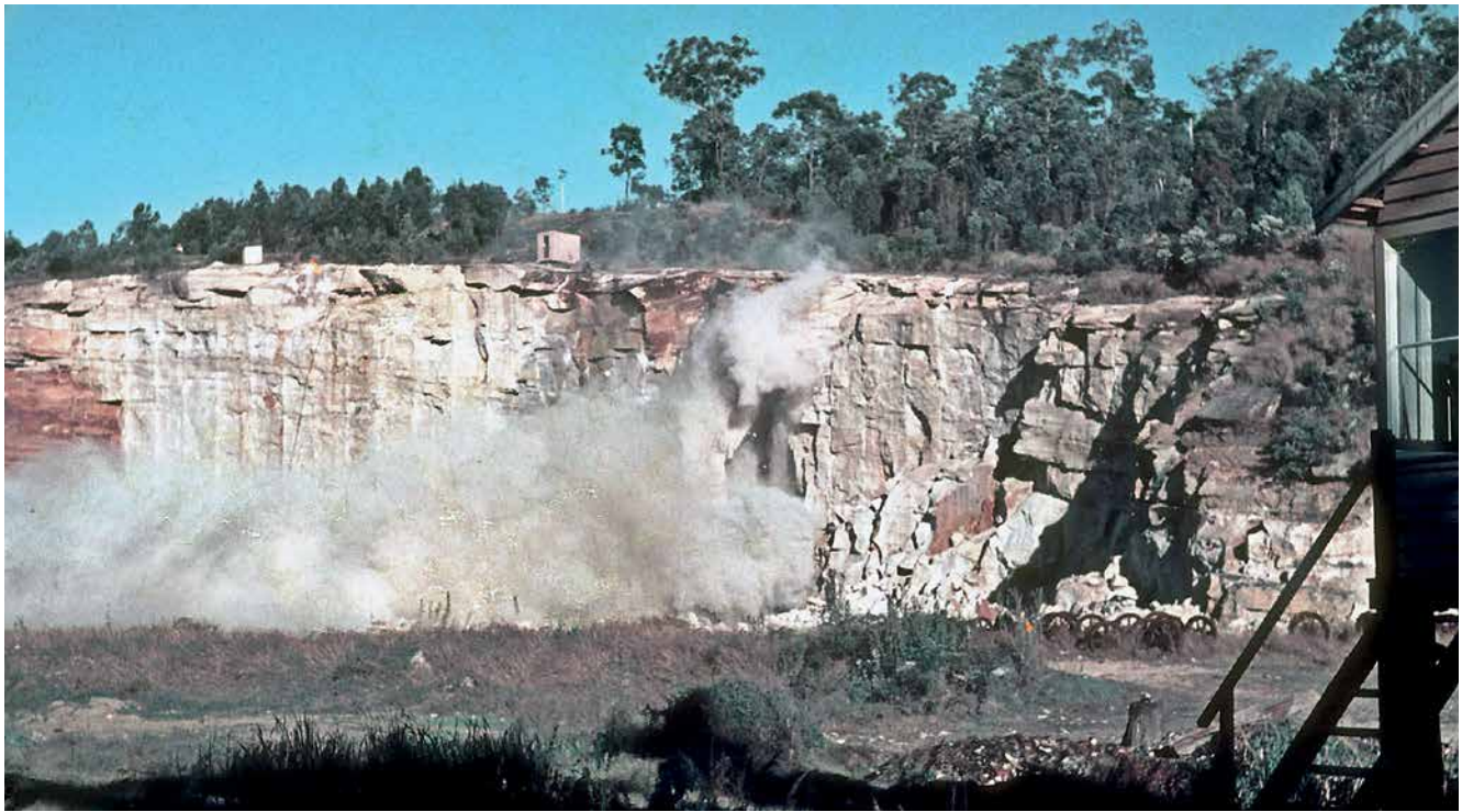
Blasting operations involving up to 1,800lb charges of explosives were carried out every month or so at the quarry, periodically shaking the nearby town of Maclean. Each blast could bring down anything up to 60,000 tons of stone. About half was fed through the jaw crusher for the manufacture of concrete blocks, the other half was sized into blocks between five and thirty-eight tons apiece for the breakwaters.
