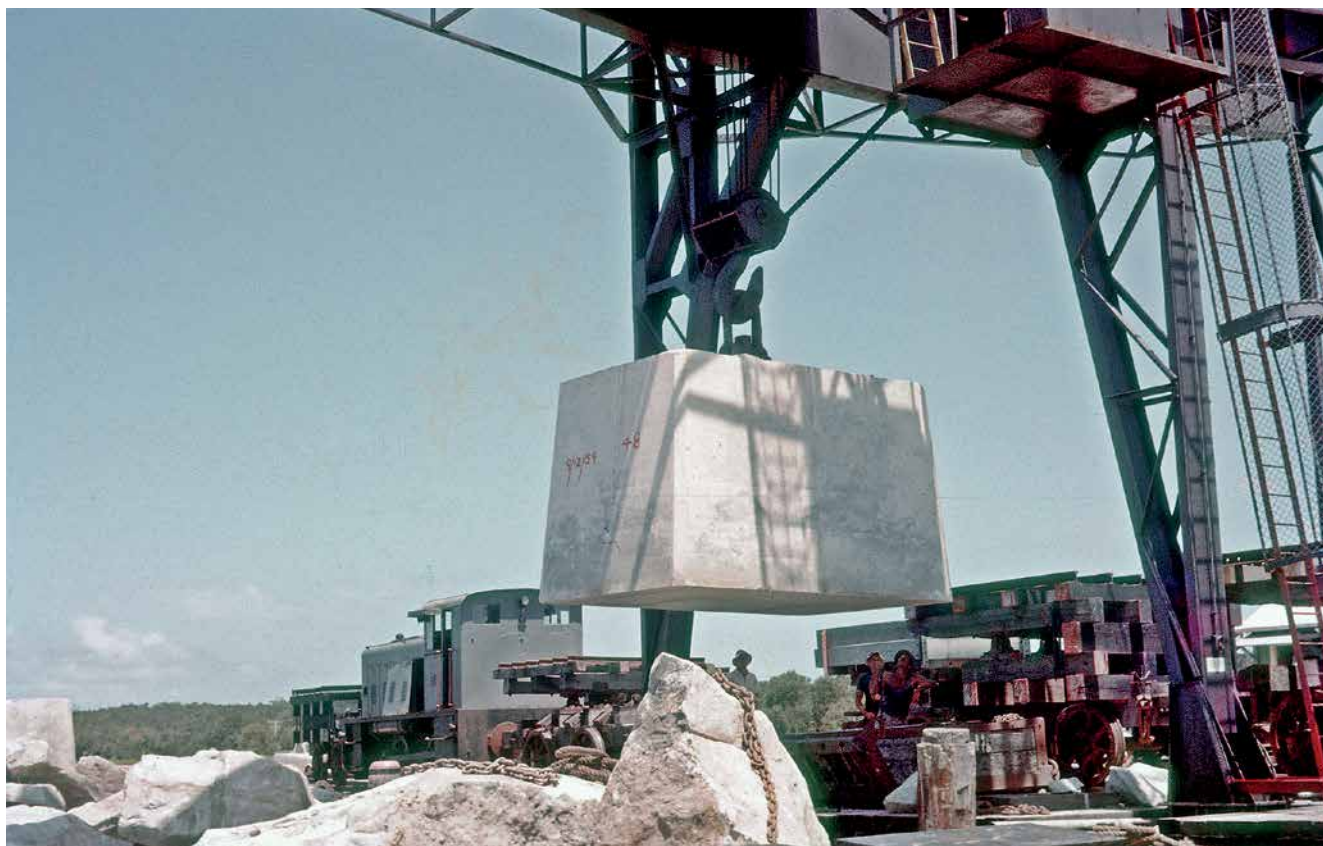
Unloading operations at Yamba Crane Wharf. With no stock-piling ability at the wharf, the diesel locomotive needed to be on hand to draw a train of empty wagons one-by-one under the portal crane for loading.
