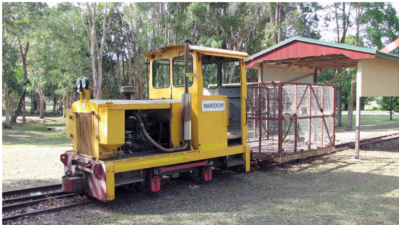
Ex Moreton Mill, Maroochy, E M Baldwin 1064 of 1964. Purchased by Tender in 2004 following the mill's closure in 2003. ' MAROOCHY ' is still pretty much in its 'work clothes' condition that it left the mill in, a broken window replaced, seats re-upholstered and the headlights moved from the roof to give clearance in Clive's shed.
