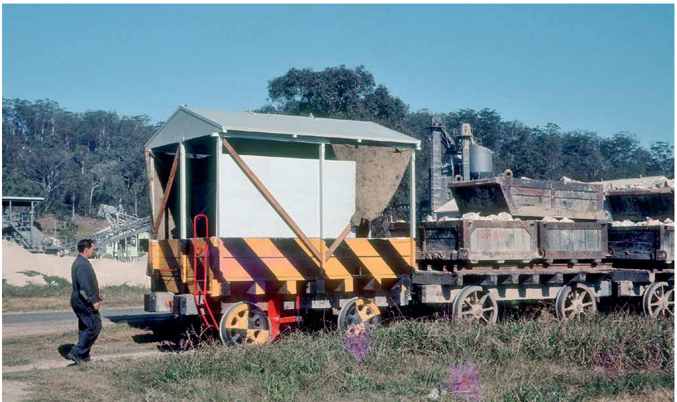
One of the four-wheel stone trucks was converted into a home-made brake van for use on the breakwater railways. It is not clear how it was used in service, or if it found much use at all. Photo: Norman Brown collection
