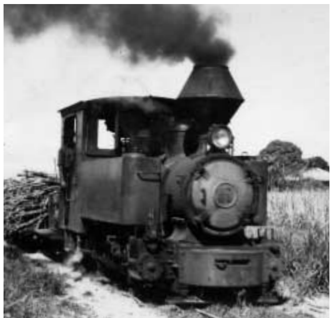
In 1953, 0-6-2T BUNDY (Bundaberg Foundry 2 of 1952) is about to cross the Daintree Road at 'Cedars' level crossing with a load of cane from Saltwater.
