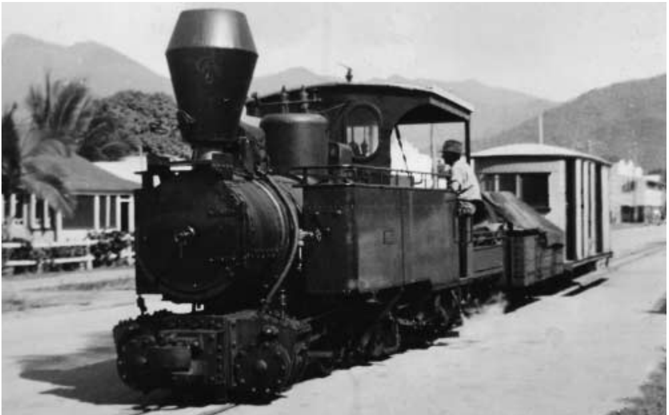
In June 1947, the Mowbray Tram is passing down Mill Street, Mosman, headed by the Shire Council's Orenstein & Koppel 0-4-4-0T compound loco DOUGLAS. (B/N 943 of 1902). Photo: E M Loveday
