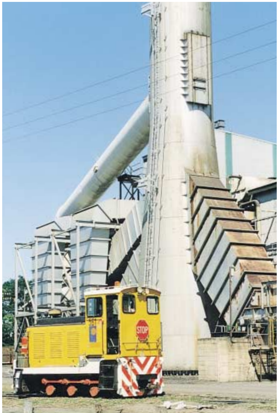
As the mill chimney towers above like a Saturn rocket, Clyde 0-6-0DH 561 (57-159 of 1957) rests briefly between duties at Millaquin Mill on 15 August 2000. Photo: Brian Webber
