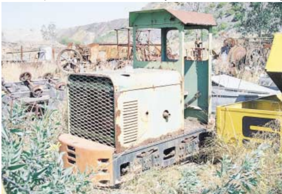
Ipswich Historical Society's Bundaberg Jenbach 4wDM 11 of 1953 in storage 27 August 2000. The bodywork and cab are not original.
