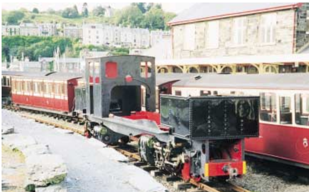
K1 parked at Porthmadog. As can be seen from the size of the Garratt, compared to the FR carriage stock on the right, it will not fit the FR loading gauge. However, this is not a problem on the WHR. Photo: Michael Chapman
