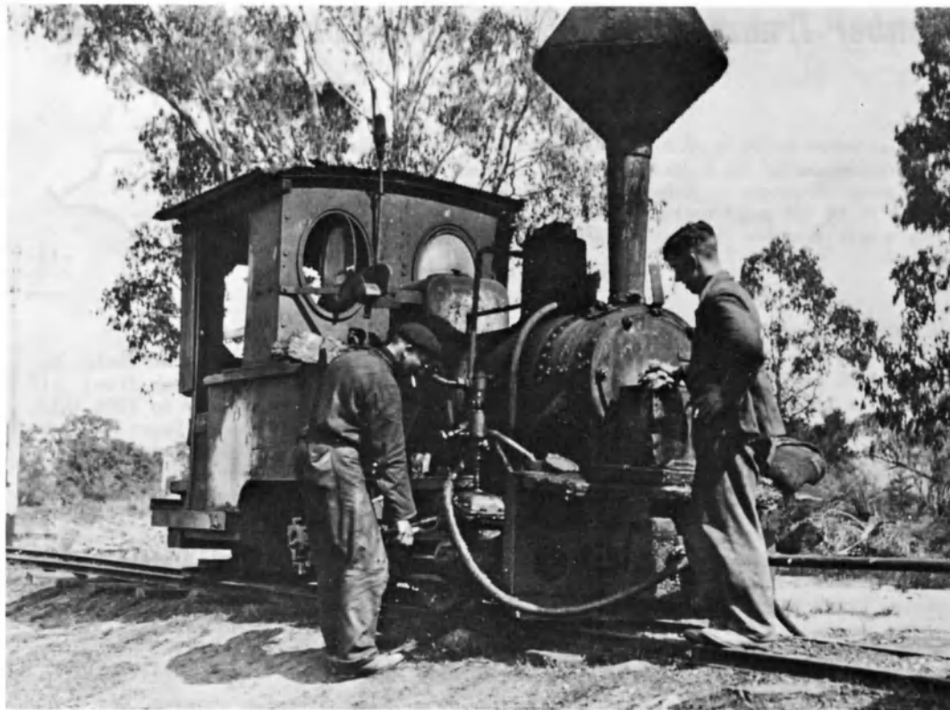
In 1934 the R.L. & T.Co's second locomotive, 2 ft gauge Krauss 0-4-0WT B/No.2591 of 1892, takes water near Thornton. Steam operation of the tramway ceased on 30 November 1935.
