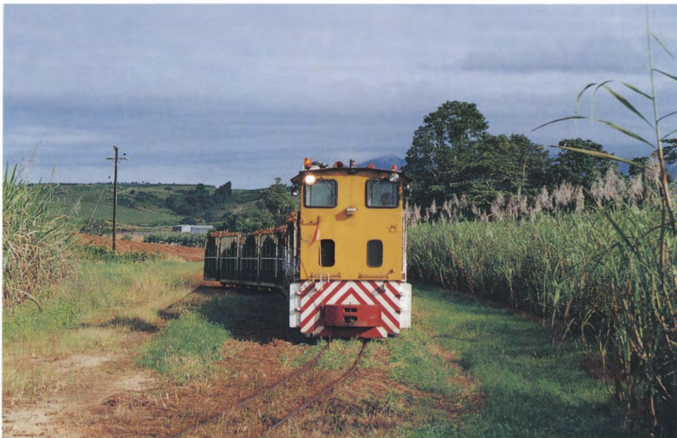
On 7 July 2000, Mourilyan Mill's Clyde 0-6-0DH 14 (63-288 of 1963) heads a rake of cane from Fedalto's siding back towards the main line, not far from the Bruce Highway. The combined buffer/coupler was originally fitted to enable Mourilyan locomotives to haul both mill and Innisfail Tramway stock. Photo: Rod Milne
