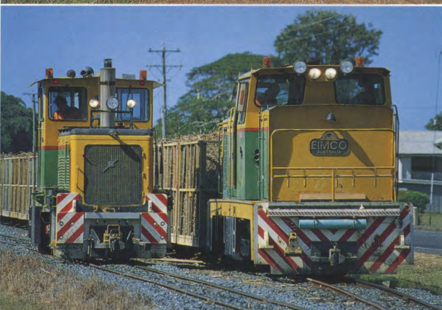
Top: Kalamia Mill's 2ft gauge EM Baldwin B-B DH NORHAM (5383-1-7-74 of 1974) hauls a 3ft 6ins gauge match wagon and molasses tank wagons on the dual gauge link between Ayr Station and the mill, 16 July 2002. Photo: Brian Webber Centre: Proserpine Mill's Clyde 0-6-0DH 7 (65-442 of 1965) on a train of bogie ballast hoppers in the mill yard, May 2002. Photo: David Rowe Above: Mackay Sugar's Pleystowe Mill yard is being used as a marshalling point for bins on their way to Farleigh Mill. Here on 13 July 2002, Clyde 0-6-0DH CONNINGSBY (61-232 of 1961) waits its next run while Eimco B-B DH FARLEIGH (L254 of 1990) heads away with a rake. Photo: David Rowe
