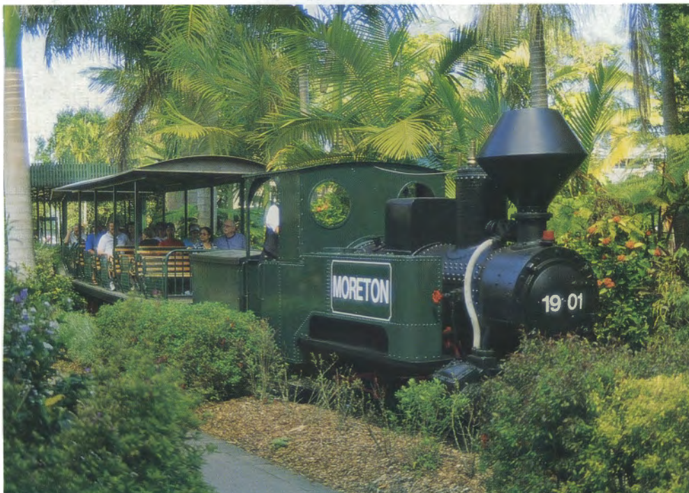
Former Moreton sugar mill 0-6-0T+4wDH MORETON (Krauss 4687/1901), converted to diesel-hydraulic operation from the tender in 1992, at The Ginger Factory, on Queensland's Sunshine Coast, 4 October 2001, Photo: Chris Stratton
