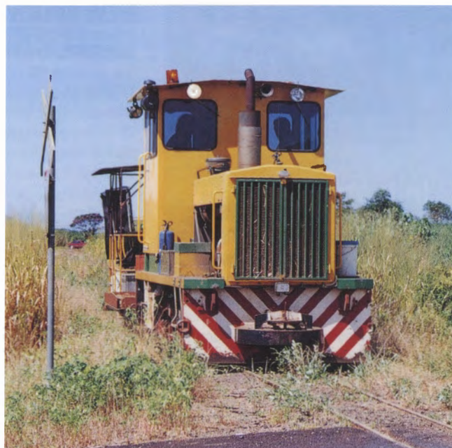
Babinda Mill's Com-Eng 0-6-0DH 9 (AH3979 of 1964), fitted with an enclosed cab at the mill, parts the grass as it hauls a weed spray train before the start of the 2000 season. Photo: Rod Milne
