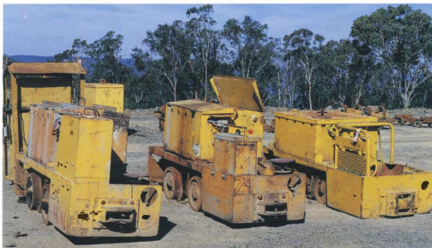
2ft gauge Gemco 3-tonne 4wBE "Hauler" 24 with 29 and an unnumbered unit await the hammer at the New England Antimony Mining auction, Hillgrove, 25 June 2002. Photo: Ray Graf
