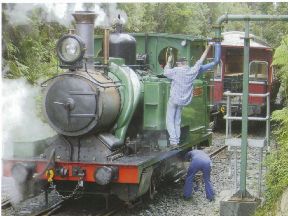
After the arduous climb up the 1 in 16, the fireman waters Mt Lyell No.1 while the driver checks the pinion gear, at Rinadeena, before the return journey to Queenstown on Saturday, February 15, 2002. Photo: Jim Shugg
