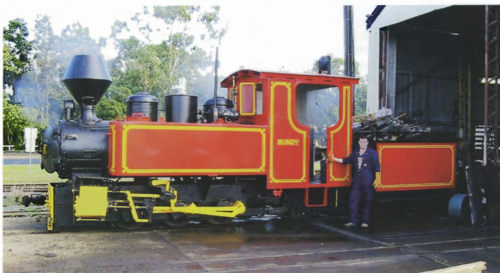
The Ballyhooley Steam Railway's Bundaberg Fowler 0-6-2T BUNDY (Bundaberg Foundry 2 of 1952) is steam tested following repairs and repainting in the Mossman Mill workshops. Photo: Ballyhooley Steam Railway
