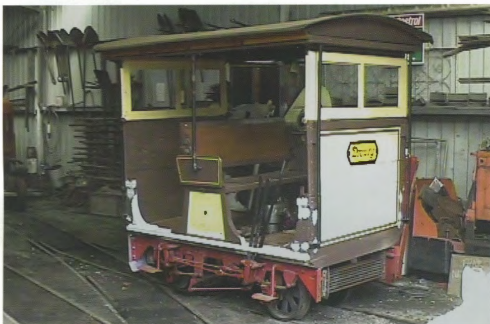
The newly restored former CSR Drewry inspection car (Baguley 1338 of 1924) in the Illawarra Light Railway workshop at Albion Park, April 2003. Photo: John Garaty
