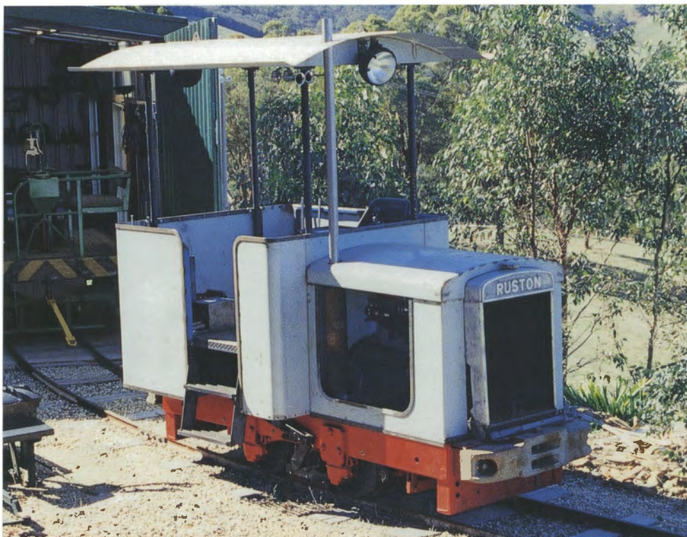
Kerrisdale Mountain Railway's Ruston Hornsby 20DL 4wDM (B/N 285301 of 1949) awaiting final painting and fitting of sandboxes, April 2003.
