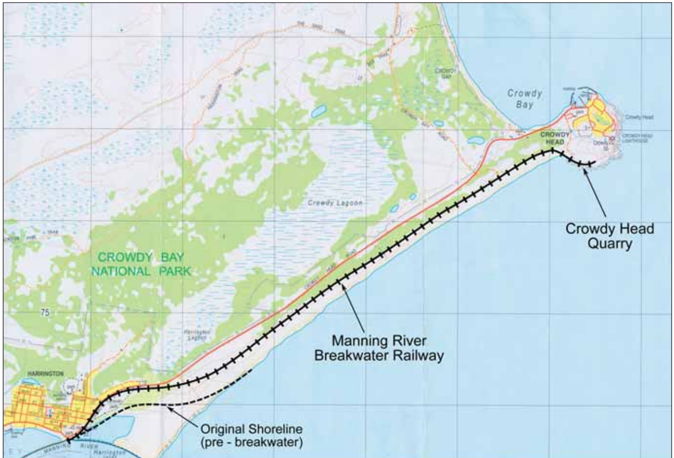
The 7.2km Breakwater Railway was built in 1895 to transport quarried rock from Crowdy Head to Harrington to build the Manning River breakwaters. It ran through thick coastal rain forest behind the beach sand dunes and was plagued by drifting sand for most of its life.
