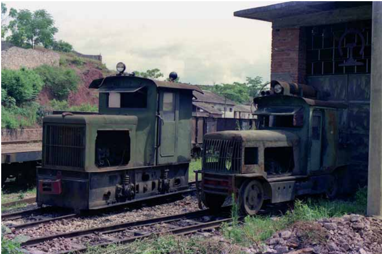
One of the very interesting 762mm gauge four-wheel internal combustion locomotives that hints of Malcolm Moore ancestry, together with what looks like a road truck conversion. Heshui, headquarters of the MeiLong Railway, Guangdong province, China, June 1991. Photo: Robin J Gibbons
