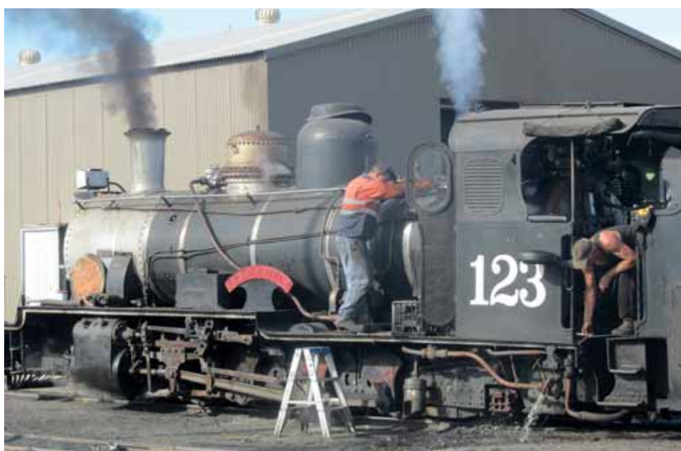
2-8-2 NG123 FREMANTLE (Anglo-Franco-Belge 2670 of 1951) undergoing steam tests on 22 April following overhaul for the 2011 steam season at the Bennett Brook Railway depot at Mussel Pool,
