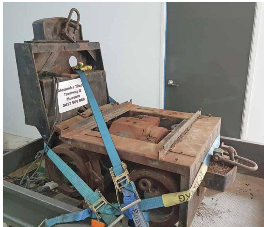
*British Electric Vehicle 0-4-OBE (now minus connecting rods) loaded on a trailer on its way to Alexandra. The vertical section is the driving position folded up for transport. Photo: Stefan Rebgetz*
