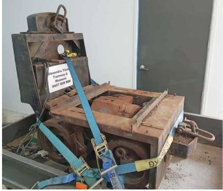
British Electric Vehicle 0-4-0BE (now minus connecting rods) loaded on a trailer on its way to Alexandra. The vertical section is the driving position folded up for transport. Photo: Stefan Rebgetz
