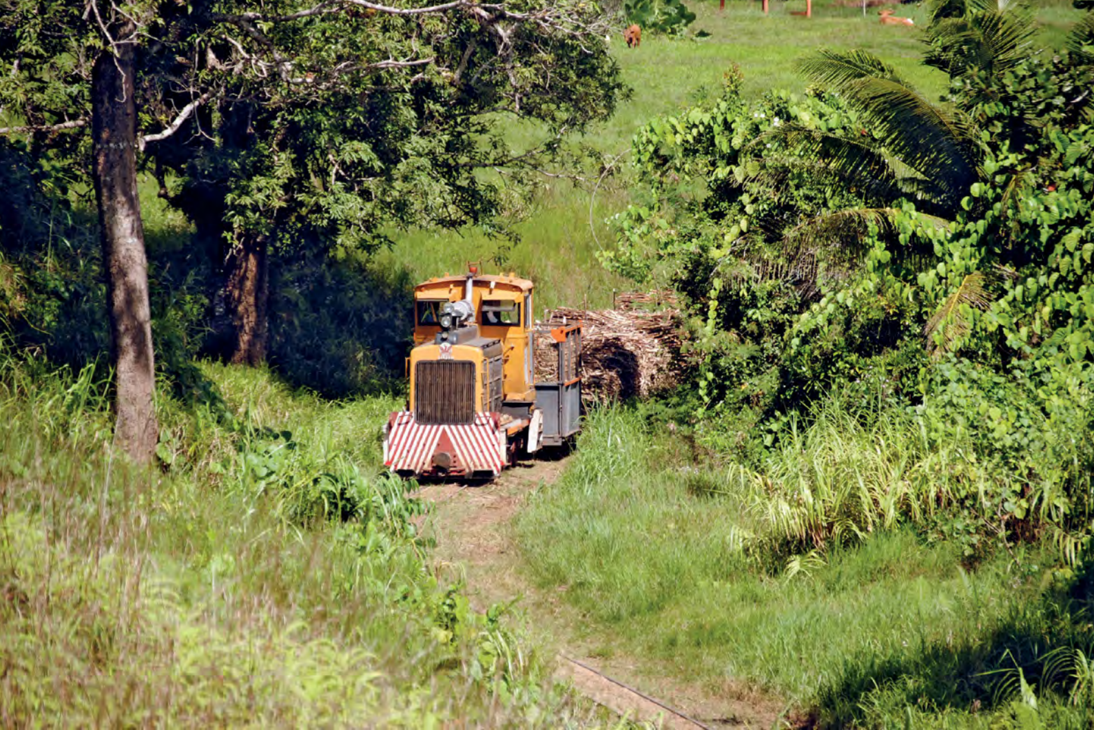
Above: Labasa Mill's Clyde 0-6-0DH 21 (64-385 of 1964) at the Daku Triangle in Fiji on 20 September. Photo: John Browning
