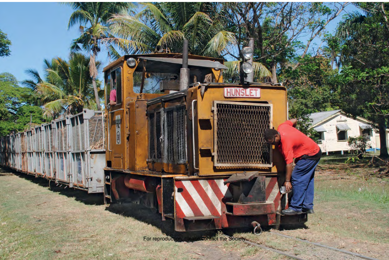
Below: The points boy of Hunslet 6wDH 198 (9273 of 1987) does some hand sanding at Navutu Road on the southern approach to Lautoka Mill in Fiji on 26 September. Photo: John Browning
