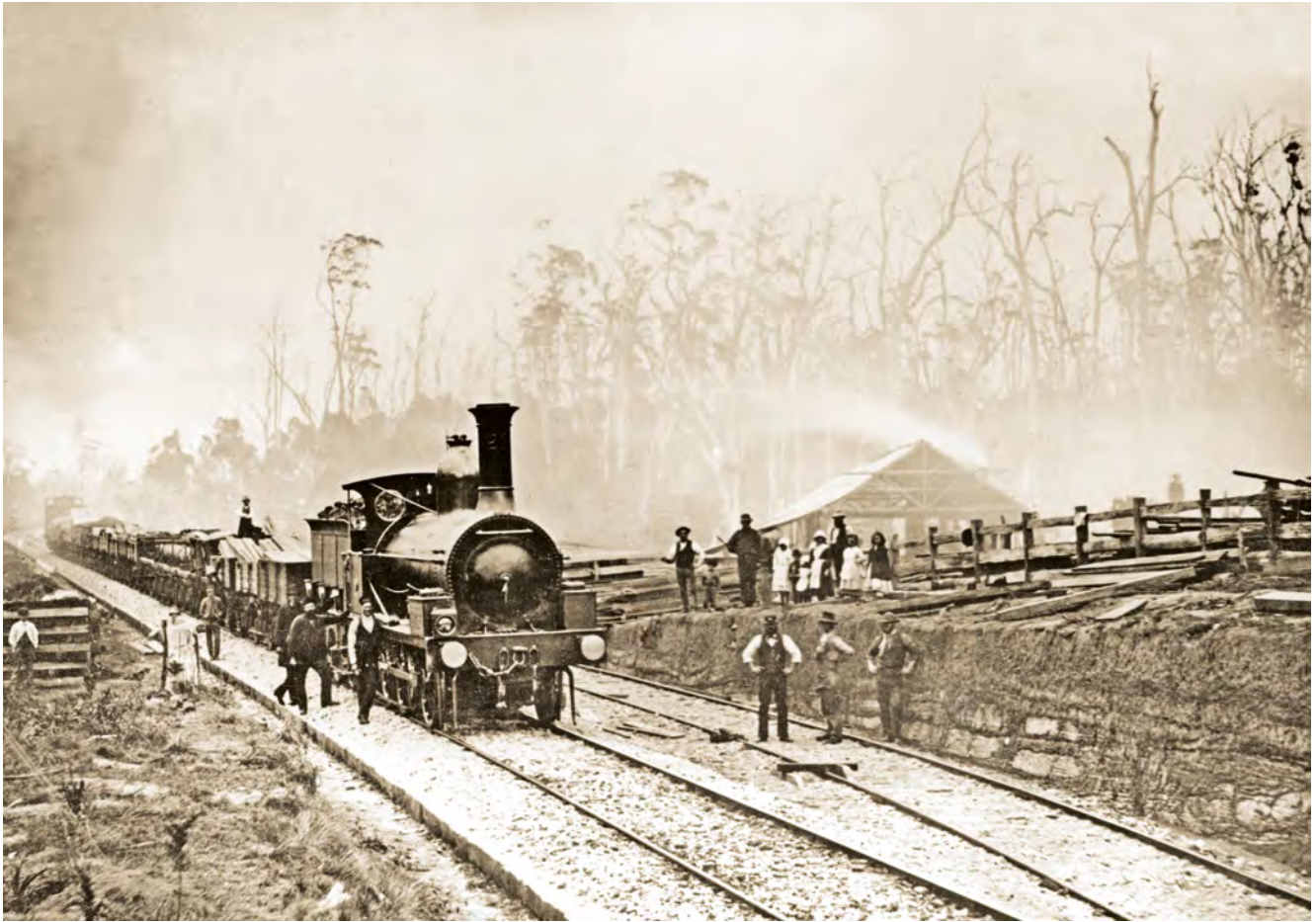
A and R Amos's sawmill and siding, about two miles north of Bundanoon railway station. NSWGR E.17 class locomotive No.20 (Robert Stephenson 1547/1864), sits with a train load of sleepers and logs in the round, on the single track mainline heading in the Down direction. It is presumed that the loco had earlier been shunting the siding as the guard appears to be standing near a stop block. Amos's sawmill, at right is adding to the smokey scene. No.20 was sold to the PWD in 1901. Photo: Author's collection
