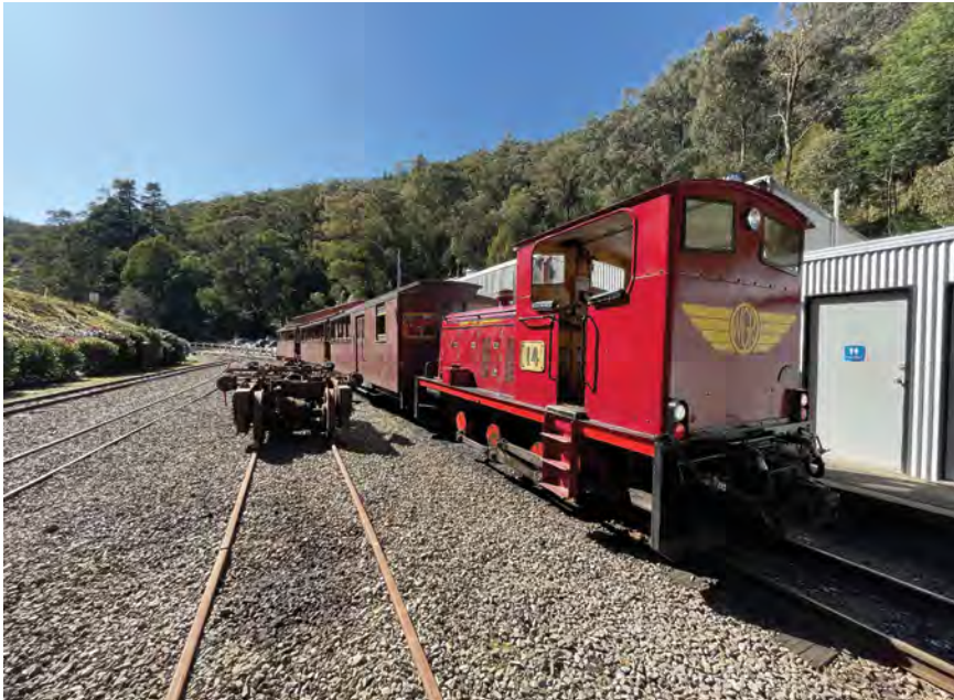
Walhalla Goldfields Railway. 31 August 2022. A perfect sunny, blue-sky day in the mountains. Ex-SECV ex-900mm gauge, John Fowler 0-6-0 diesel loco No. 14 Spirit of Yallourn, stands ready to depart with its 3-car train, from Walhalla to Thomson. Photo: Phillip Milbourne
