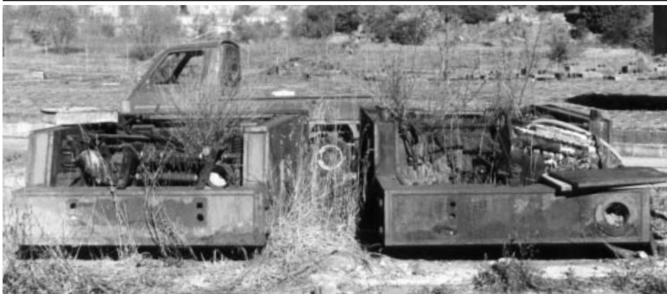
The left hand unit is 3ft 6ins gauge General Electric 4wWE 2989 or 2990 of 1909, as reconstructed at Glen Davis with new frames built by Thirlwell & McKenzie (Wollongong) in 1946. This 8 ton loco had been supplied new for the Sulphide Corporation, but was purchased by the National Oil Pty Ltd, Glen Davis, in 1940. (The right hand unit was built at Glen Davis in 1947 utilising new frames supplied by Goninan.) State Mine Museum, Lithgow, NSW, October 15th 1994. Photo: Ray Graf
