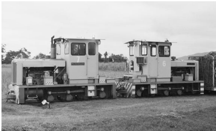
Babinda Sugar: Commonwealth Engineering 0-6-0DH 7 MORRISON (AD1239 of 1960) and 6 ALLISON (C2234 of 1959), newly equipped for working in multiple, on the Bramston Beach Road, 2/10/97.
