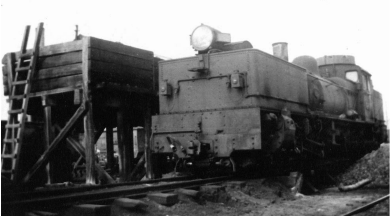
G42 rests by the Colac coal stage in the late 1950s. The two Garratts were fitted with electric lighting in 1958, when a new timetable for the Wednesday Goods moved the departure time from 8am to 2am.
