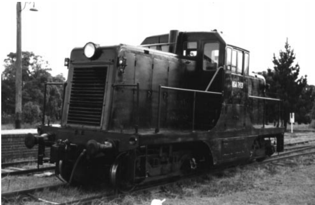
GE "44 Tonner" 17939 of 1943 at the NSW Rail Transport Museum, Thirlmere, in its original guise of USA 7921. Photo: Jim Martin
