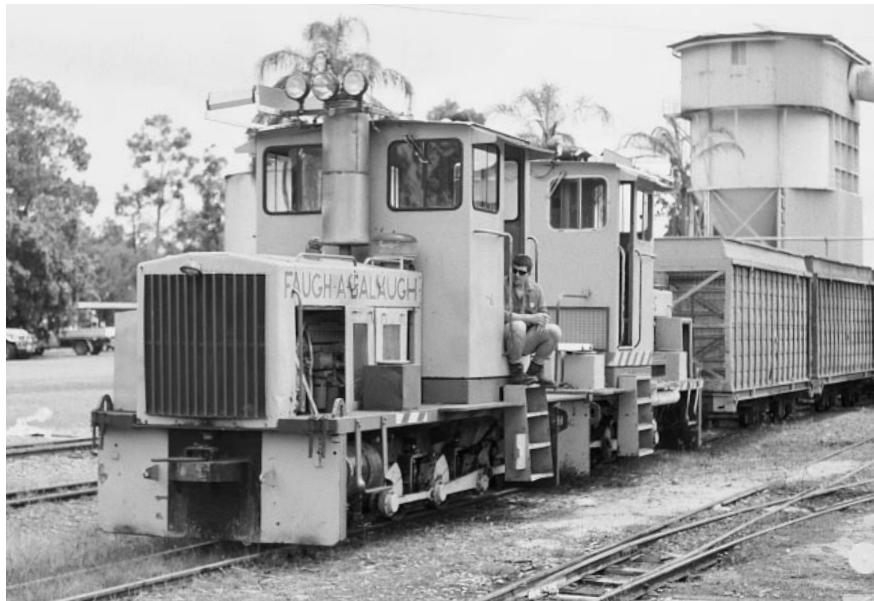
Mossman Central Mill Company: Commonwealth Engineering 0-6-0DH FAUGH A BALOUGH (AL4190 of 1965) and DOUGLAS (AL2562 of 1963), working in multiple, bring a rake of loaded bogie canetainers through the mill yard, 2/10/97.
