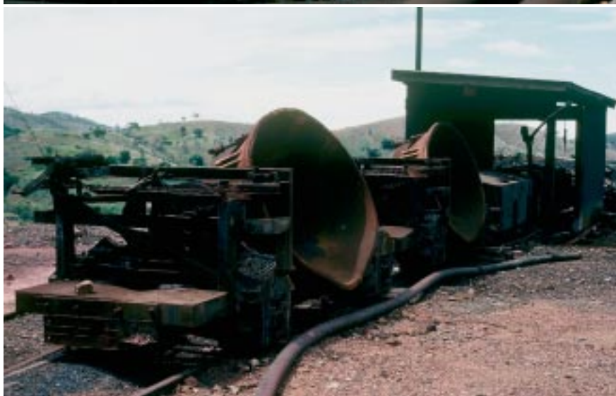
Top: A four-wheel trolley wire electric locomotive on the track above the lime? storage bins at Mt Morgan Above: Two slag cars and two four-wheel electric locomotives stored out of use near the smelter. February 1978 Photos: Tony Weston
