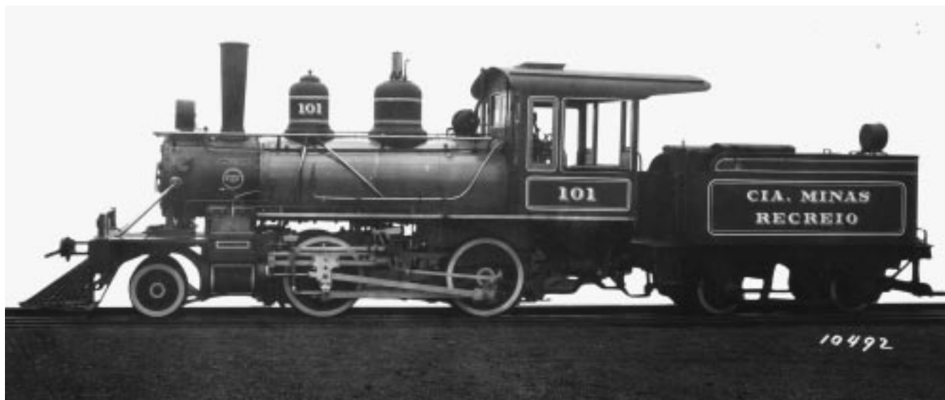
The last Baldwin 6-14C class, it was metre gauge, built for Cia Minas Recreio, Brazil, in 1929, and the only one built to Drawing No.6. The main differences to LITTLE YARRA are Walschaert valve gear, a steel cab, and four wheel tender. Photo: Courtesy Vance Bass
