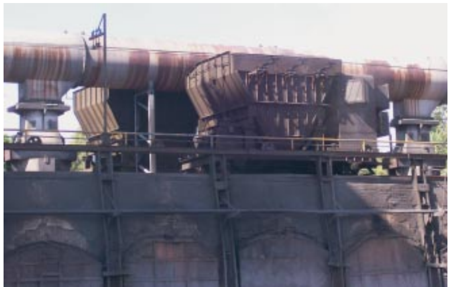
Twin charge cars delivering coal to the ovens at Bowen Coke Works in north Queensland.
