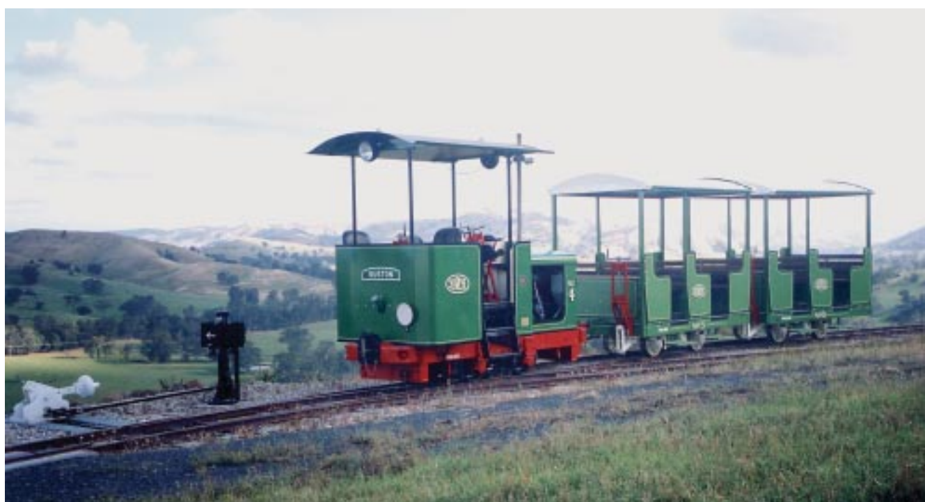
Two of the restored carriages stand in The Summit Loop on the Kerrisdale Mountain Railway with the restored Ruston & Hornsby 20DL locomotive No.4 (B/N 285301 of 1949). The KMR brake pedestals and the 'lift' given by the rubber springing will be noted in comparing this scene with the appearance of the carriages on arrival at Kerrisdale.
