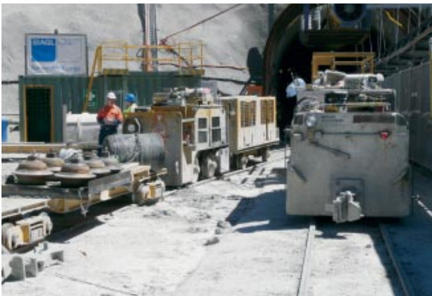
762mm gauge trains waiting at the upper tunnel portal of McConnell-Dowell's Bogong headrace access tunnel in north-eastern Victoria, 16 November 2008. The locomotive on the left is a Clayton 4wDH, almost certainly B1864E of 1979, while on the right is an ex-Mining Equipment Inc Plymouth 4wDH. Both bogie and four-wheel rolling stock can be seen. (See LR 205 p.21 for further details). Photo: Phil Rickard
