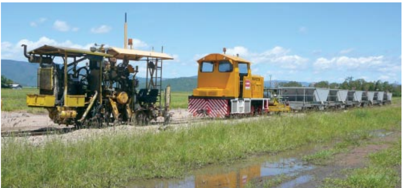
Invicta Mill navy equipment at Dibella's on Victoria Mill's Stone River line, 21 March 2009: Plasser 133 of 1978, Com-Eng 0-4-0DH INVICTA (CA1040 of 1960), a ballast plough and six ballast hoppers.
