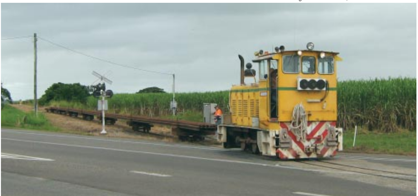
Victoria Mill's Clyde 0-6-ODH INGHAM (64-382 of 1964) heads a train away from Victoria Mill with rail bolsters destined for the new works being carried out at McKell's depot, 4 April 2009.
