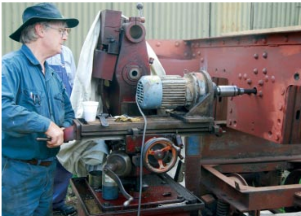
The arrangement set up by volunteers at the Alexandra Timber Tramway to re-drill the holes in the frame of Hudswell Clarke 1098 of 1915. Photo: Peter Evans
