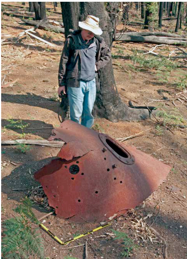
Society Secretary Phil Rickard examining a section of the boiler that exploded at Slocumb & Walker's mill on 23 May 1904 – still lying where it landed. Photo: Colin Harvey, September 2009
