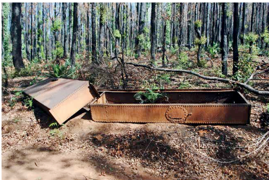
Side tanks off a Hudswell Clarke locomotive, dumped on South Junction Form, 15 April 2016.
