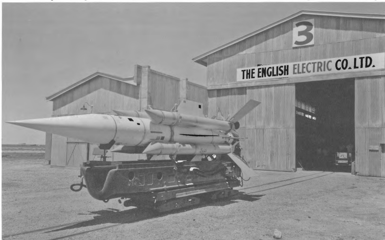
This December 1957 view shows the Red Shoes missile on its launcher trolley outside Test Shop No. 3. The detachable driver's seat can just be seen under the nose of the missile. In the shadows of the Test Shop entrance is the battery electric flat car, The Flier. Photo: LRWE
