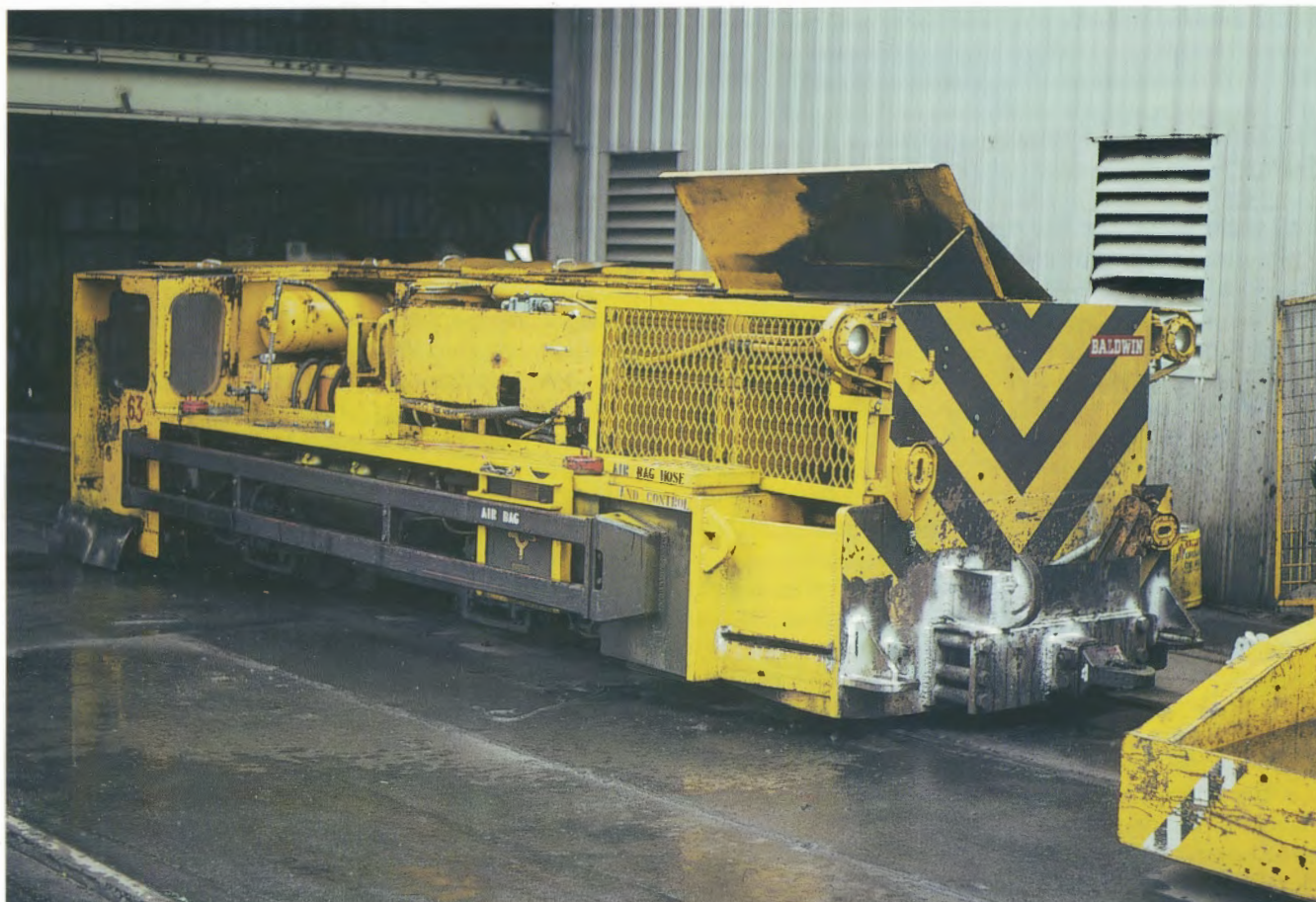
Munmorah State Mine 63 standing at pit top on 22 January 1993. This locomotive rebuild utilised the original Moxon frame with alterations to accommodate the new equipment installed. Photo: Craig Wilson
