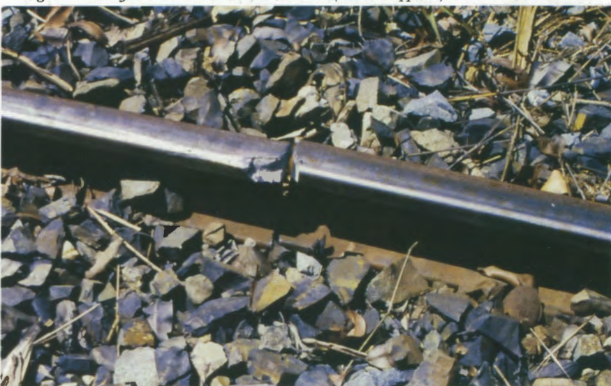
The broken rail that caused all the trouble.
