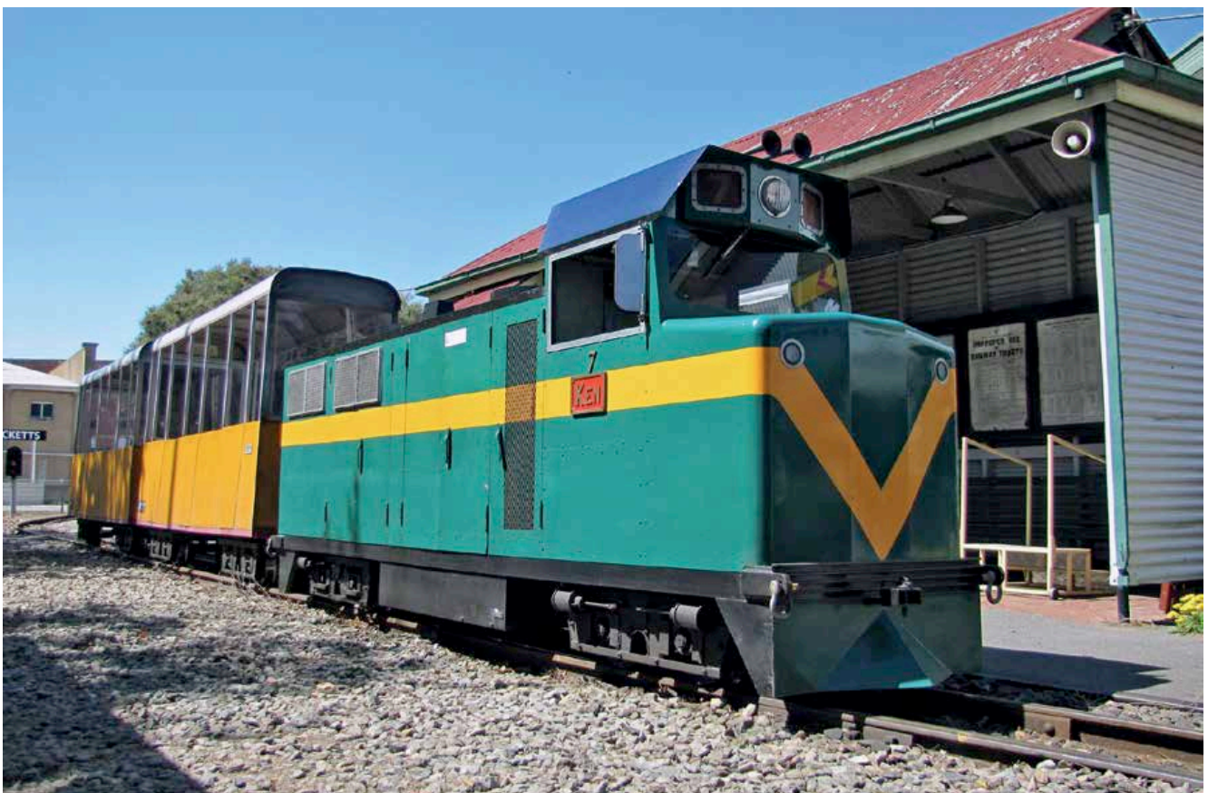
Below: Internal combustion diesel locomotive No.7, named Ken has been in use at the Port Dock site since early 1990s. Ken was designed and built by volunteers at the railway museum. It has spent brief periods working on the Semaphore to Fort Glanville Railway. It is now used extensively at the National Railway Museum as the standard loco power for the miniature train ride. Photo: Michael Chapman
