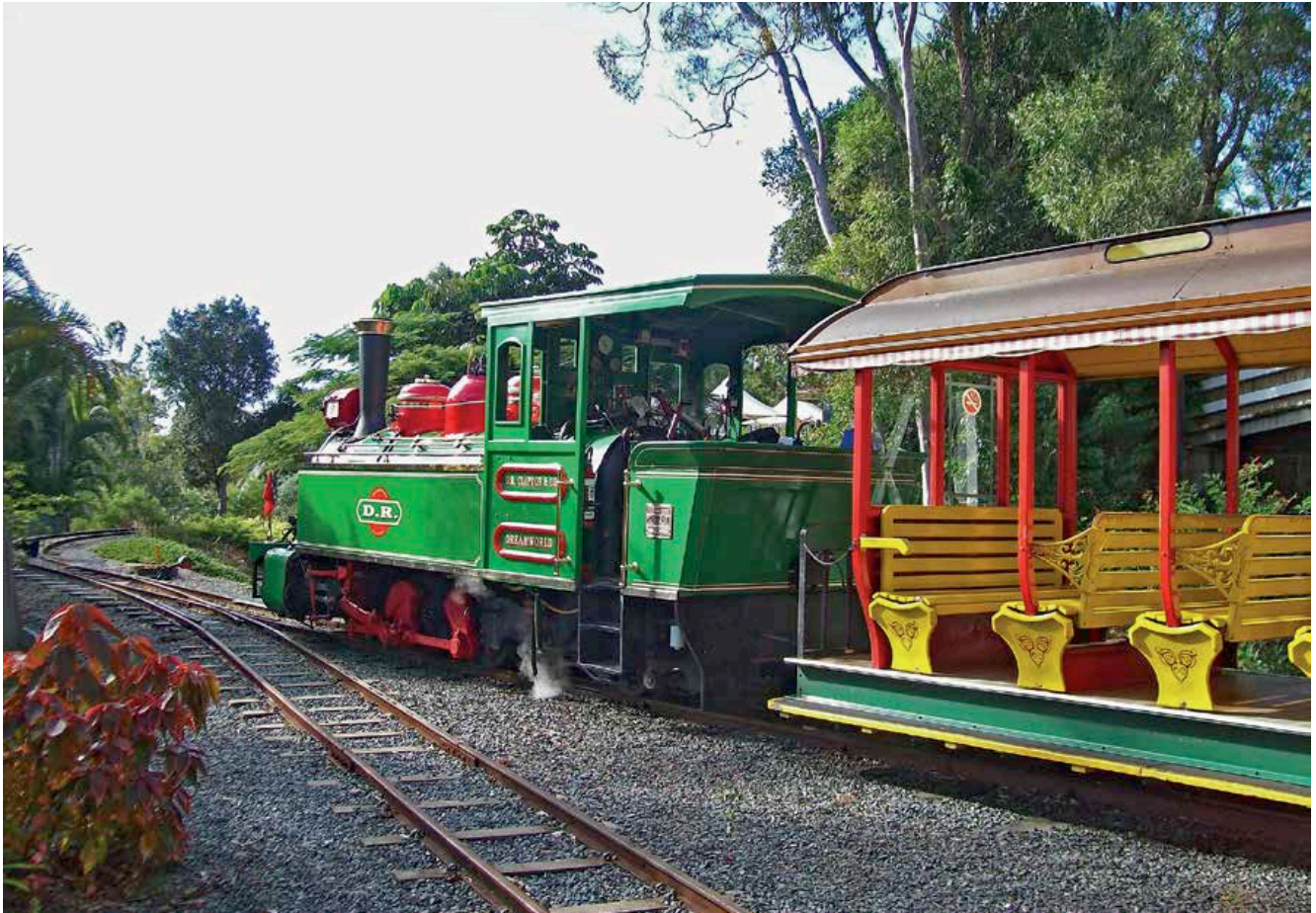
The Perry is ready to depart the Train Shed for the day's run. Notice construction of the carriage – an excellent copy of the carriages at Disneyland except for being 2 feet gauge instead of 3 feet.
