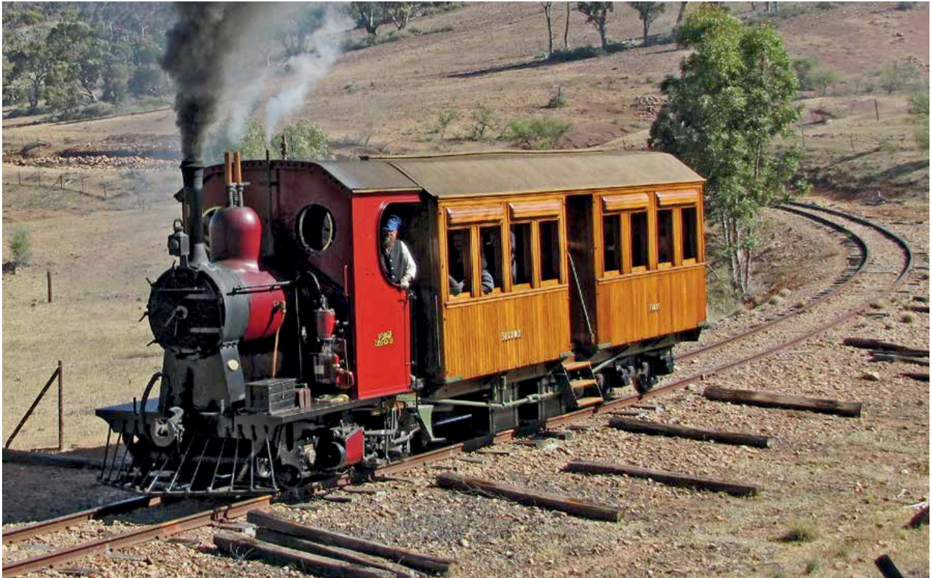
The unique Pichi-Richi Railway Coffeepot, shown approaching the road crossing near the summit, was acquired by the SAR in 1906 as Steam Motor Coach No.1; a 2-2-0WT, the engine unit was Kitson built 4356/1905, the carriage was from Metropolitan Carriage & Wagon Company. Taken over by the CR as NJAB1, it was withdrawn from service in 1932. It was refurbished externally in the late 1950s and transferred to Alice Springs for display by the National Trust. In 1973 it was acquired by the PRRPS and restored to working order by 1984, and ran into the 1990s until the boiler needed work. It was returned to service in 2016. Photo Michael Chapman
